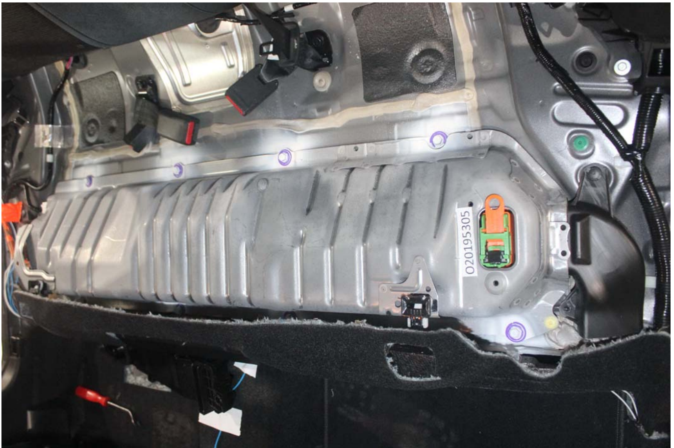
Photo No. 008 - Pre-Impact View of Propulsion Battery
