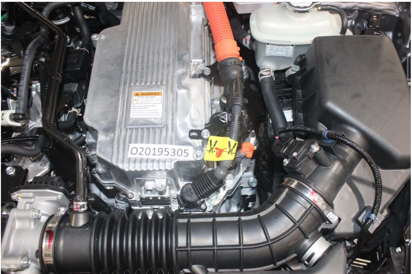
Photo No. 004 - First Responder Warning Location
