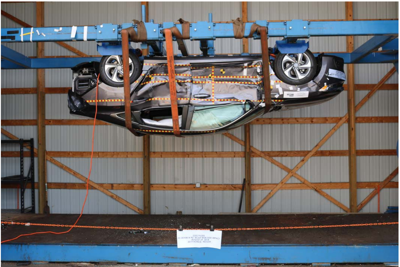
Photo No. 028 - FMVSS No. 305 Static Rollover at 180°
