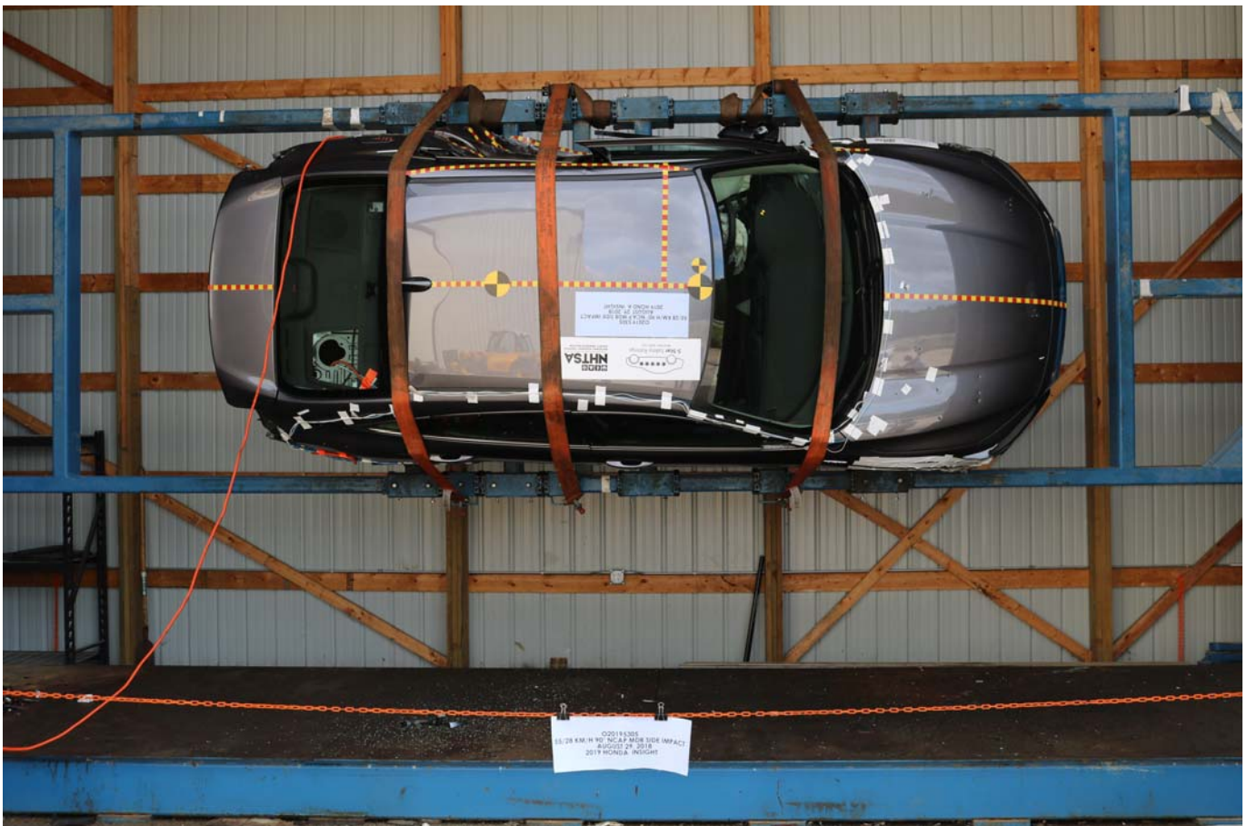
Photo No. 029 - FMVSS No. 305 Static Rollover at 270°
