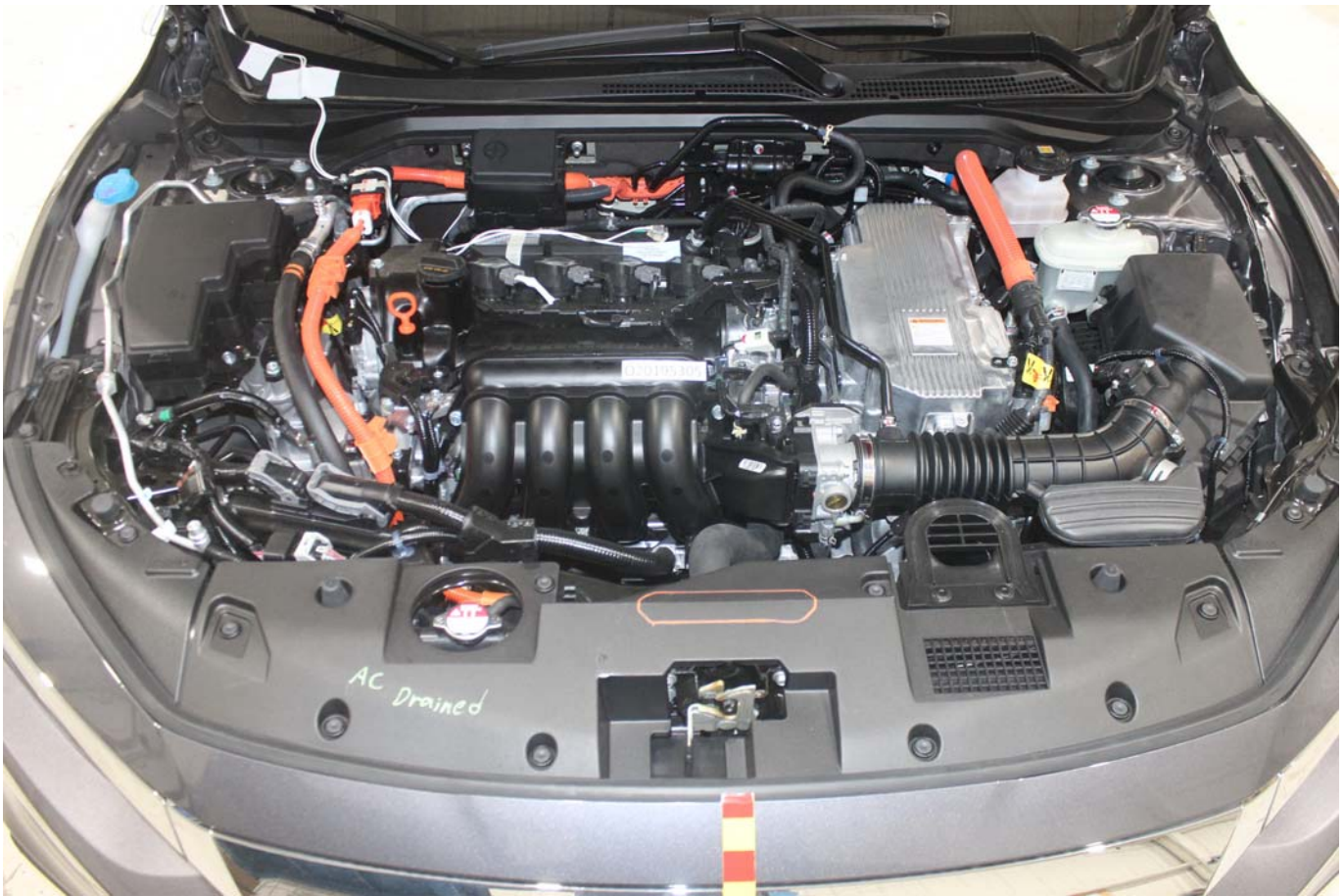
Photo No. 015a - Pre-Impact View of Electric Propulsion Drive
