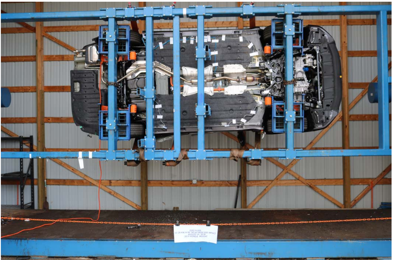
Photo No. 027 - FMVSS No. 305 Static Rollover at 90°
