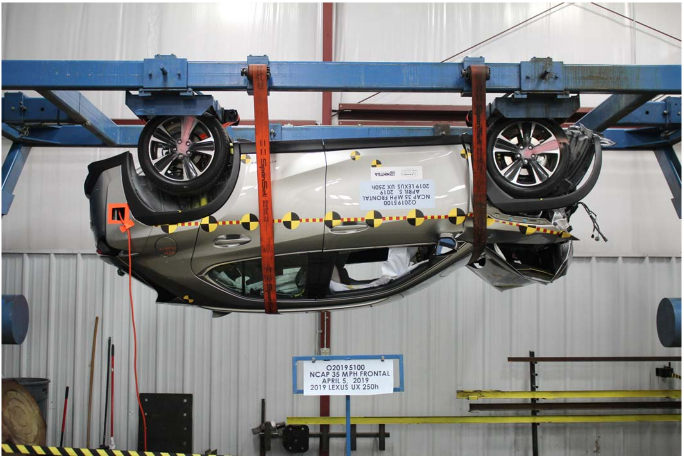
Photo No. 028 - FMVSS No. 305 Static Rollover at 180°
