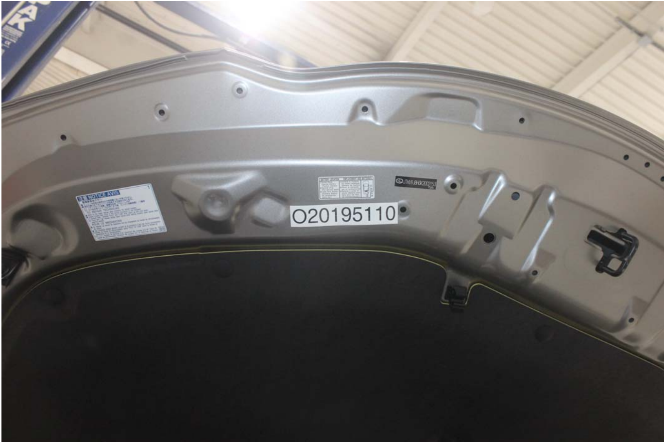
Photo No. 004 - First Responder Warning Location
