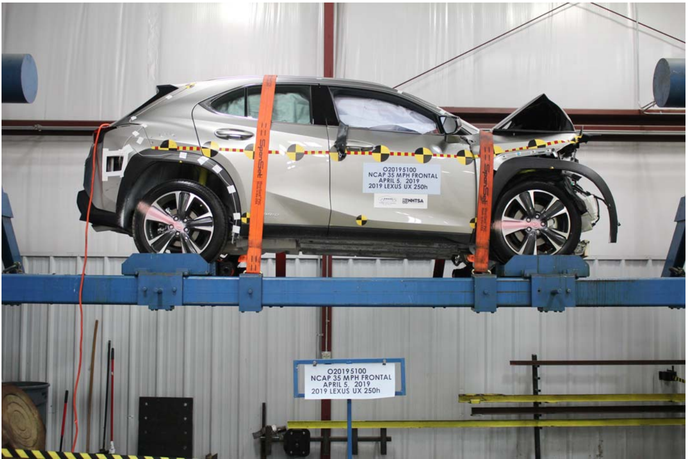
Photo No. 030 - FMVSS No. 305 Static Rollover at 360°
