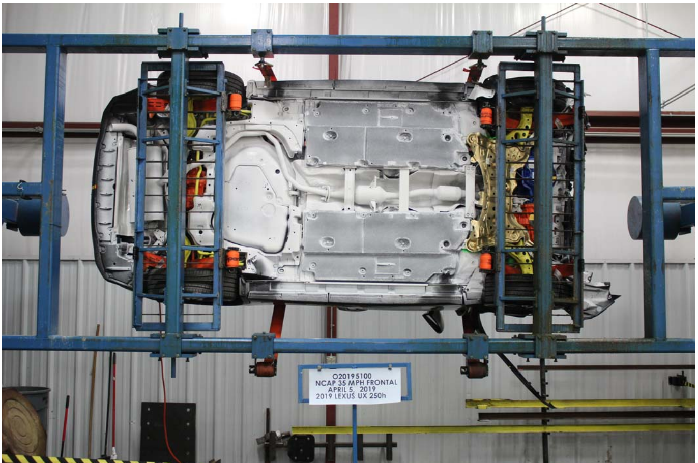
Photo No. 027 - FMVSS No. 305 Static Rollover at 90°
