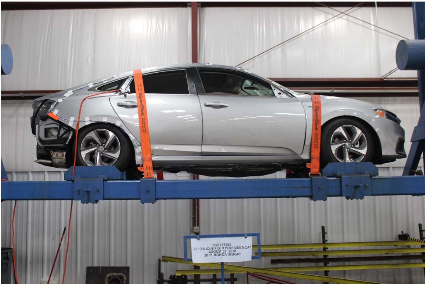
Photo No. 030 - FMVSS No. 305 Static Rollover at 360°
