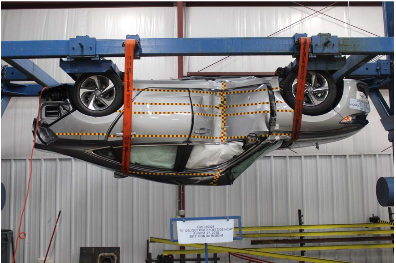
Photo No. 028 - FMVSS No. 305 Static Rollover at 180°
