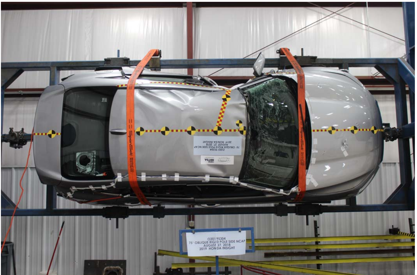
Photo No. 029 - FMVSS No. 305 Static Rollover at 270°
