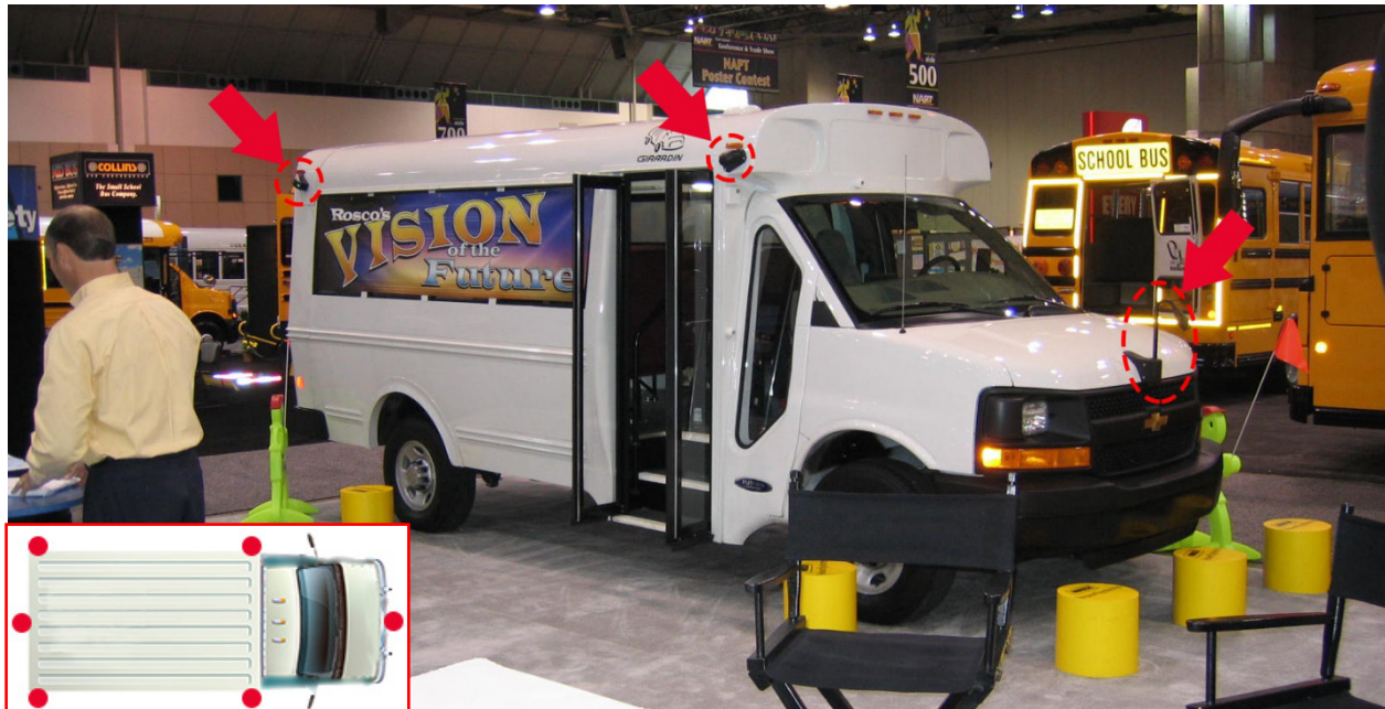
Mirrorless Vehicle Exterior - A total of six cameras were installed (two LH + two RH + one Front + one Rear)
