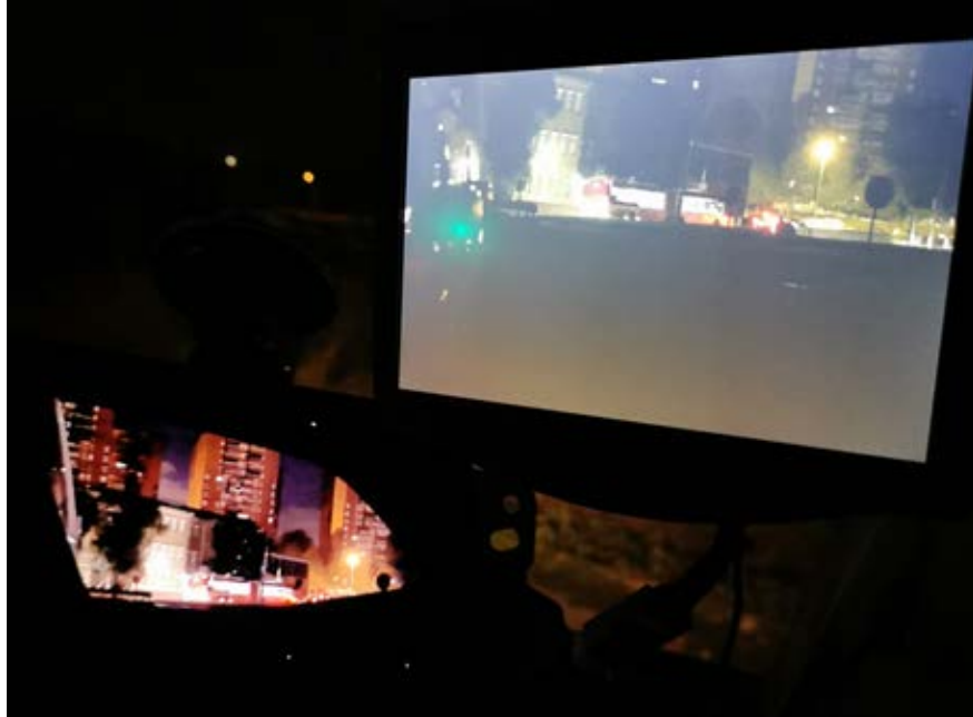
Figure 7. CMS evaluation of perceived brightness in low light environment, comparison between a system adjusted based in the SAE J1757 standard (left) and a system adjusted without using SAE J1757 standard as reference (right)
