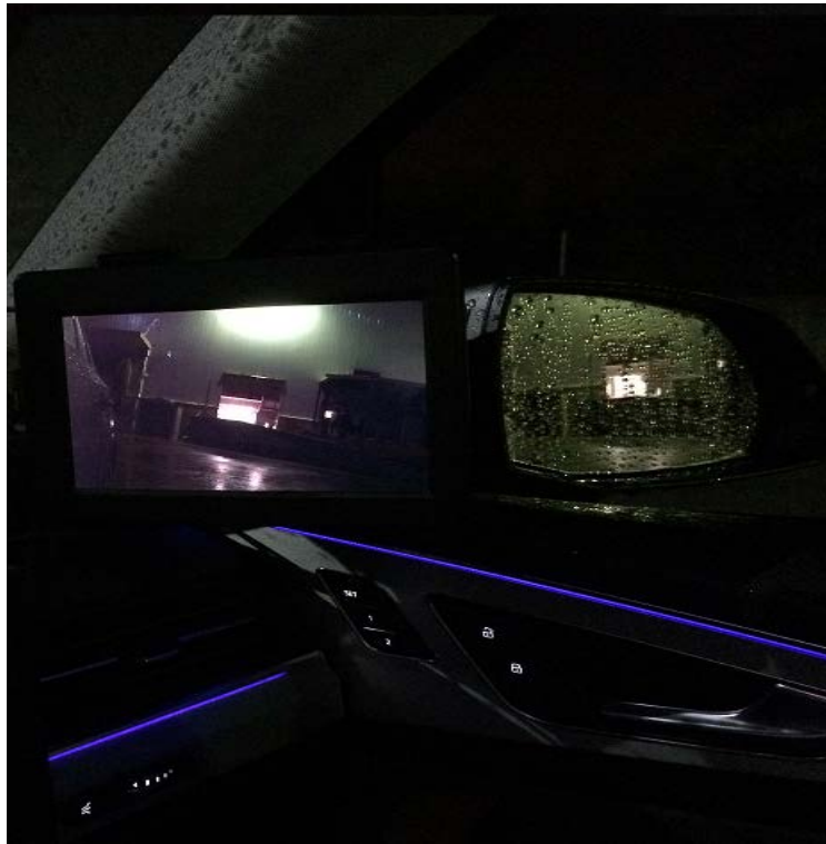
Figure 13. CMS performance evaluation under rainy weather condition ©FICOSA International SA
