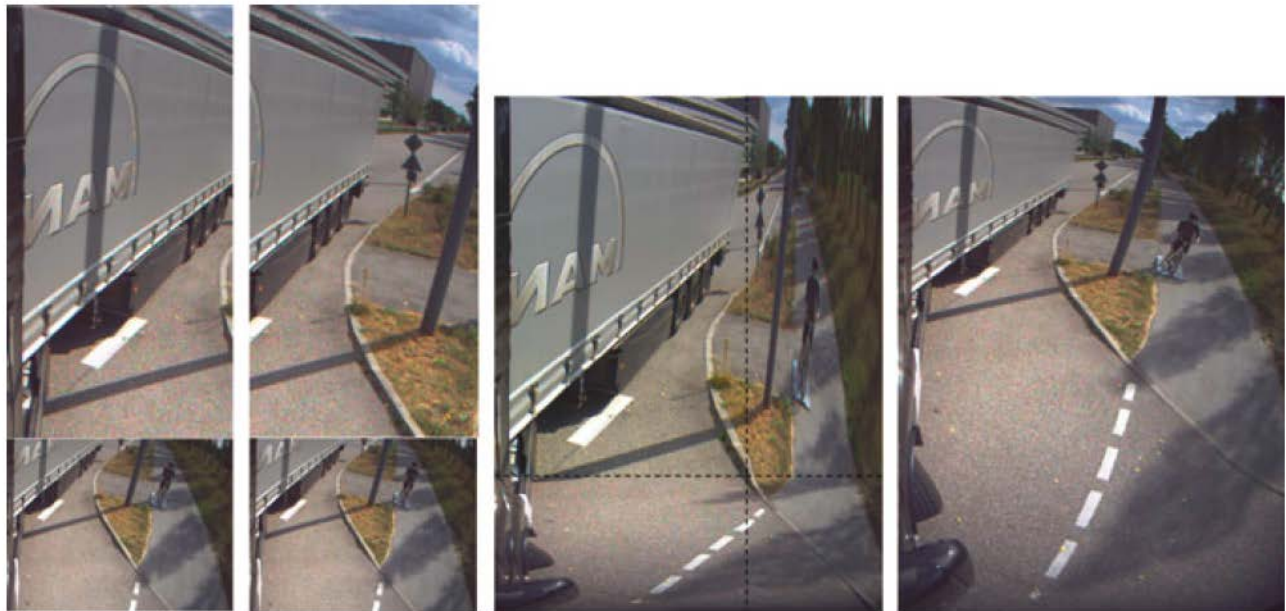
Fig. 12 Comparison of different presentation concepts ( left to right ): 1:1 replacement; 1:1 replacement with camera panning; combined replacement; combined replacement with maneuver view
