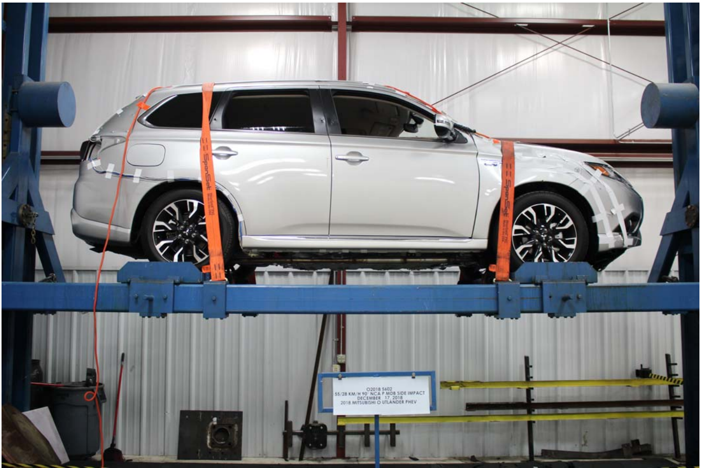
Photo No. 030 - FMVSS No. 305 Static Rollover at 360°
