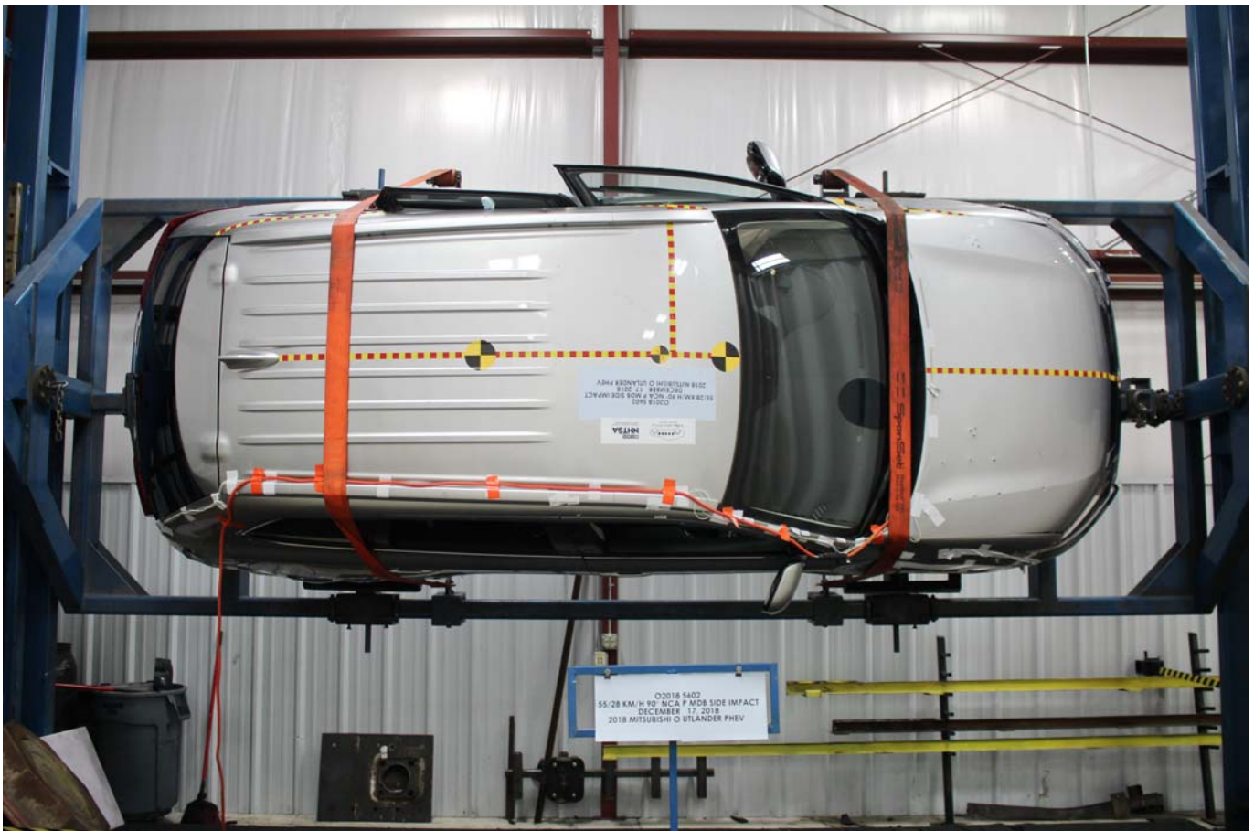
Photo No. 029 - FMVSS No. 305 Static Rollover at 270°
