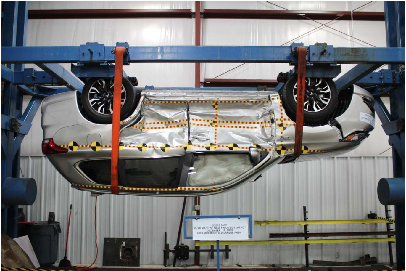
Photo No. 028 - FMVSS No. 305 Static Rollover at 180°
