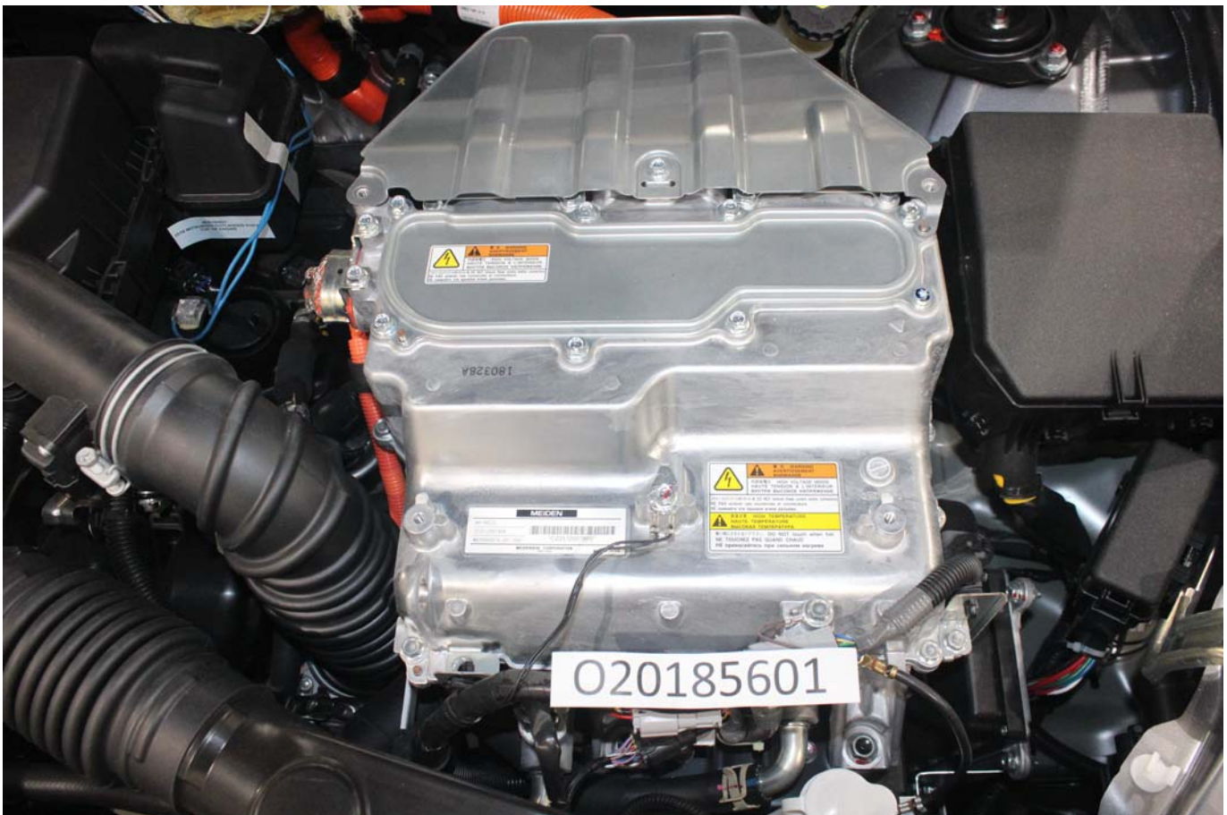
Photo No. 002 - Power Inverter Warning Label
