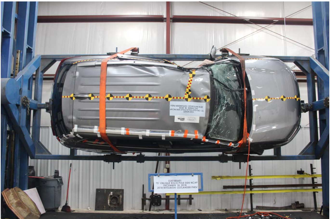
Photo No. 029 - FMVSS No. 305 Static Rollover at 270°
