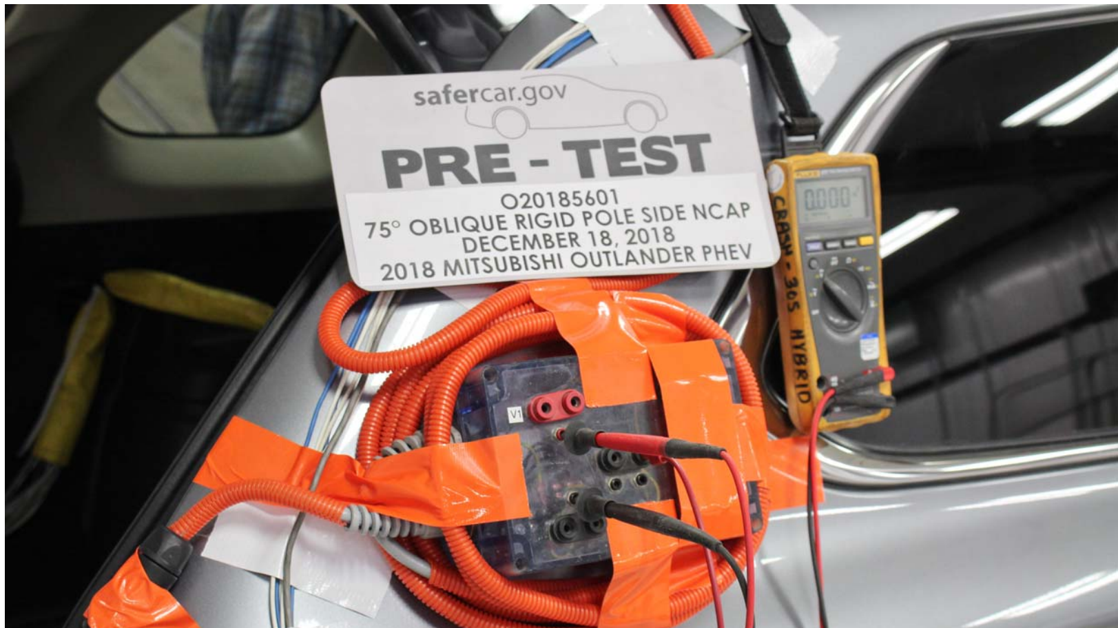
Photo No. 023 - Pre-Impact View of Installed Impact Interface Port
