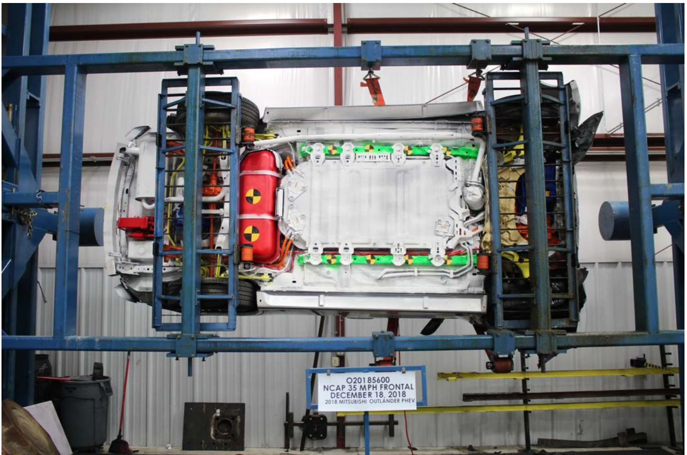
Photo No. 027 - FMVSS No. 305 Static Rollover at 90°
