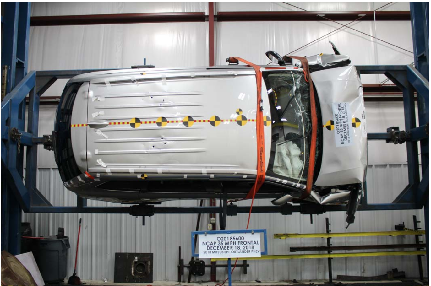
Photo No. 029 - FMVSS No. 305 Static Rollover at 270°
