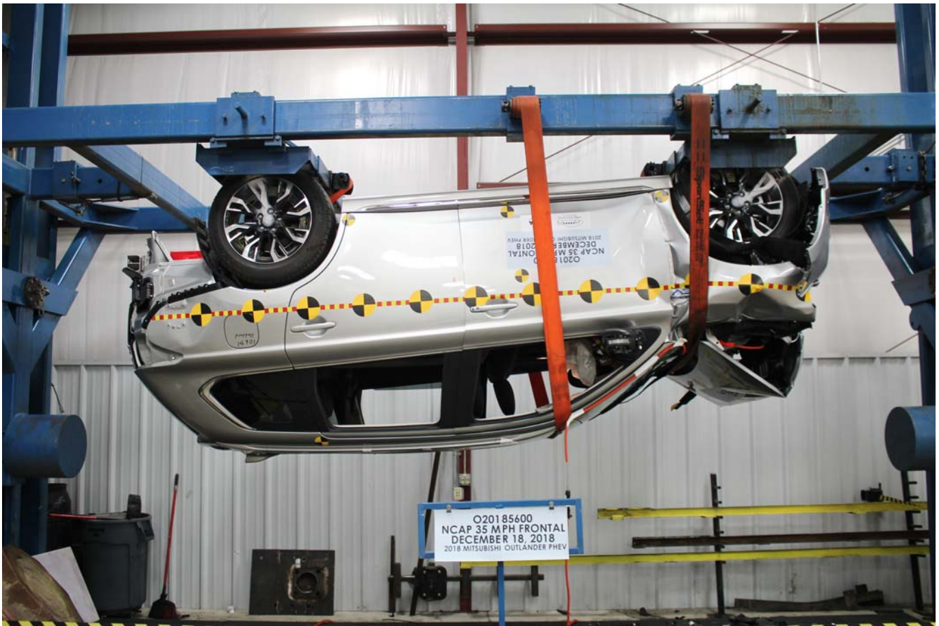
Photo No. 028 - FMVSS No. 305 Static Rollover at 180°
