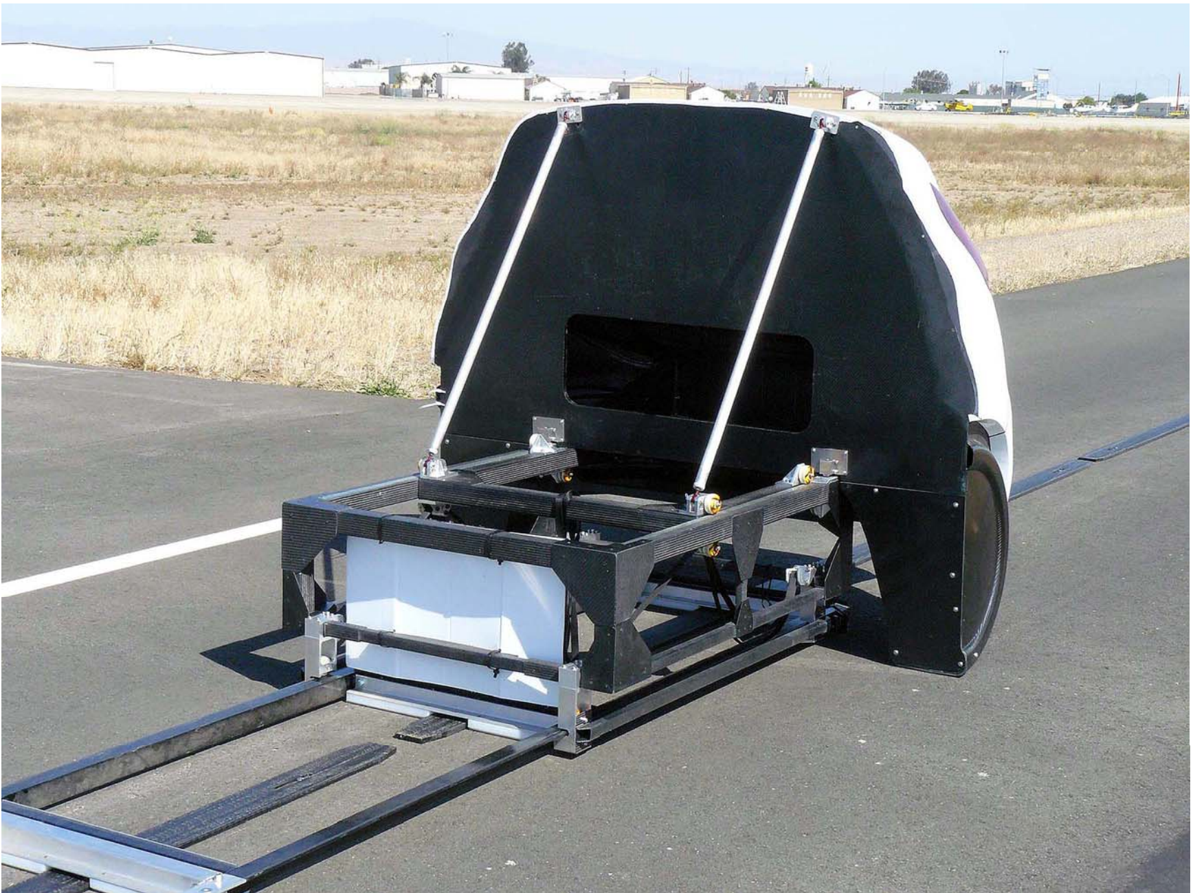
Figure A7. Load Frame/Slider of SSV
