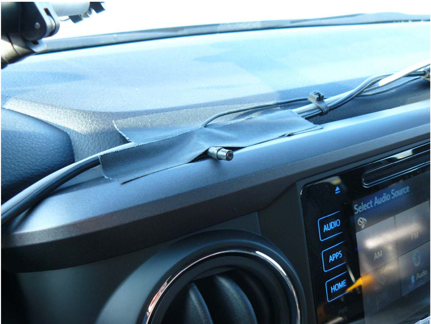
Figure A11. Sensor for Detecting Auditory Alerts
