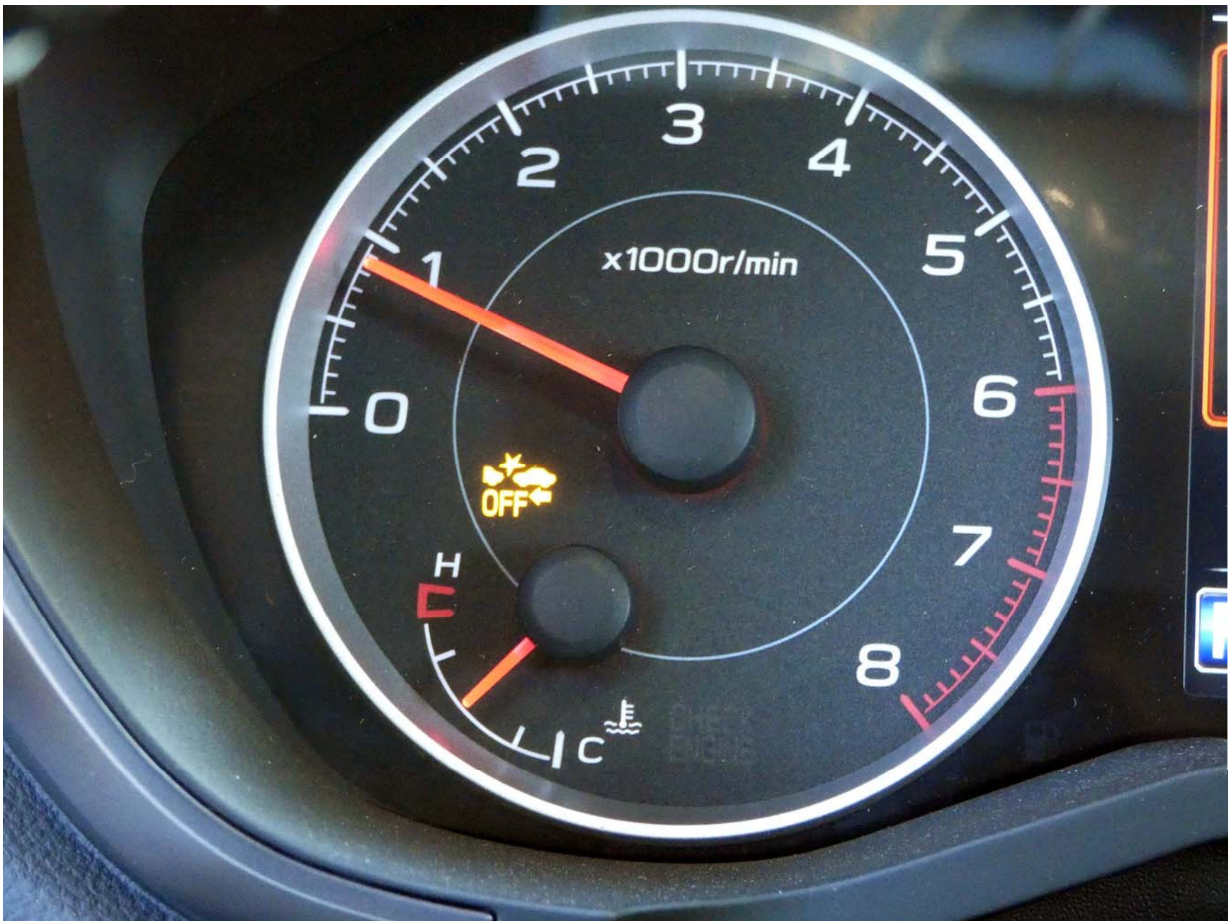
Figure A17. AEB Off Indicator Light
