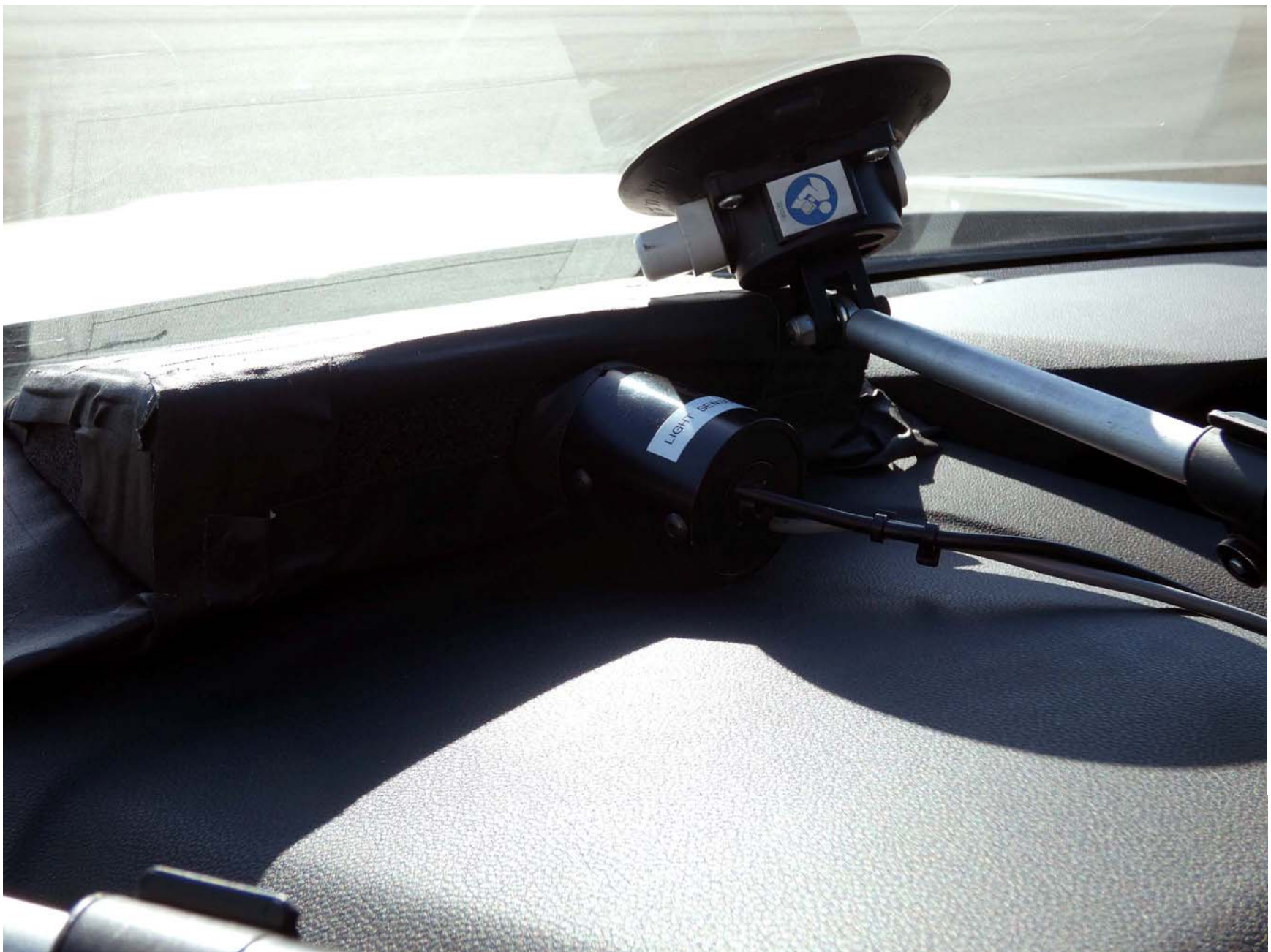
Figure A12. Sensor for Detecting Visual Alerts
