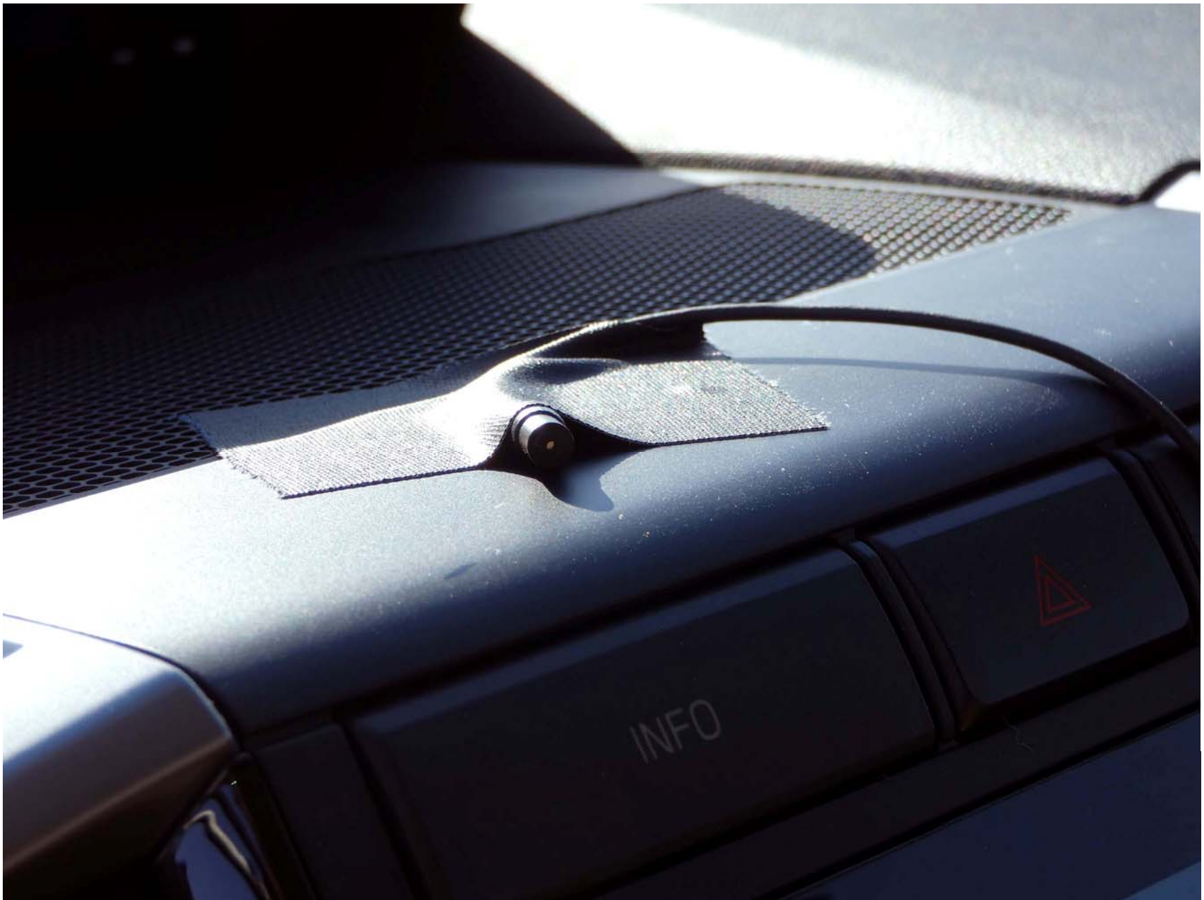
Figure A11. Sensor for Detecting Auditory Alerts
