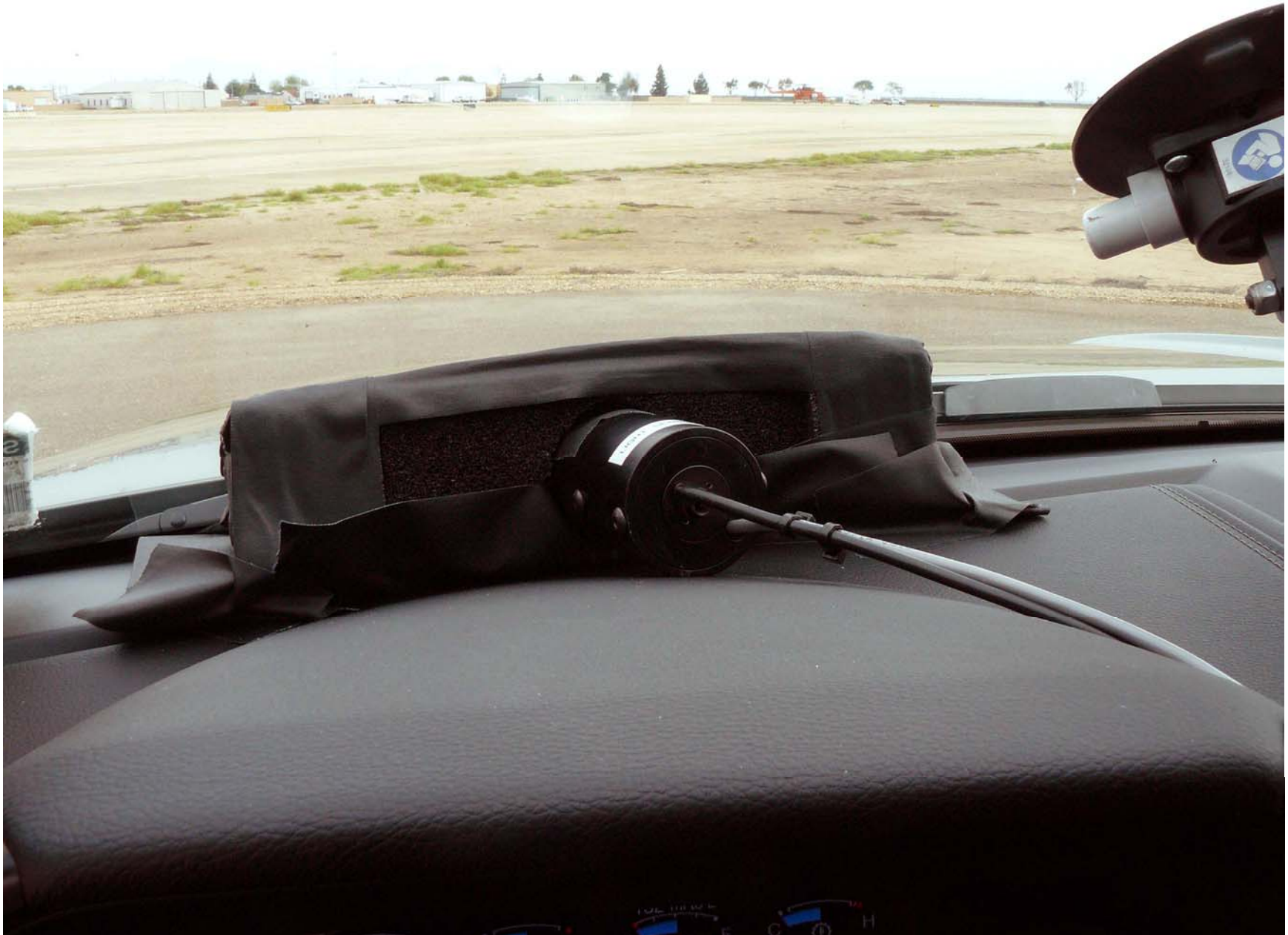
Figure A12. Sensor for Detecting Heads Up Visual Alerts
