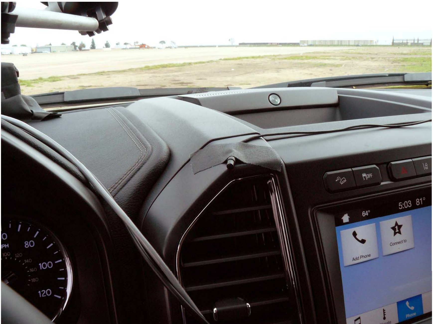
Figure A11. Sensor for Detecting Auditory Alerts
