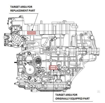
\* VIN plate for originally equipped part will be attached to either ① or ②.
