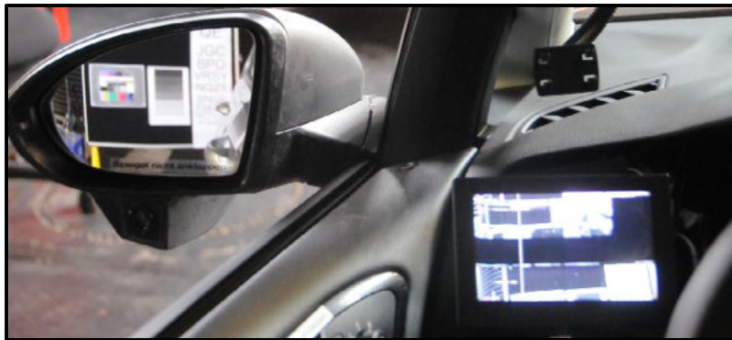
Figure 40: Error in image caused by electromagnetic radiation.
