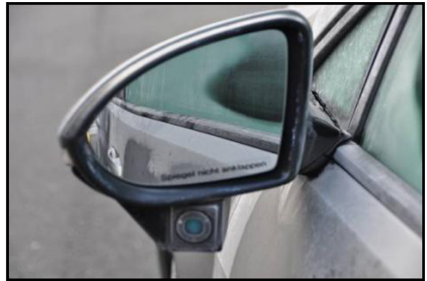
Figure 45: Mirror is clear, camera still shows condensation.
