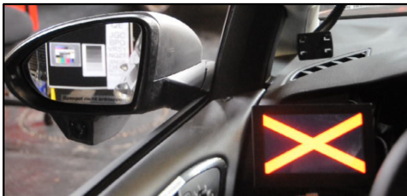
Figure 41: Loss of image caused by electromagnetic radiation.
