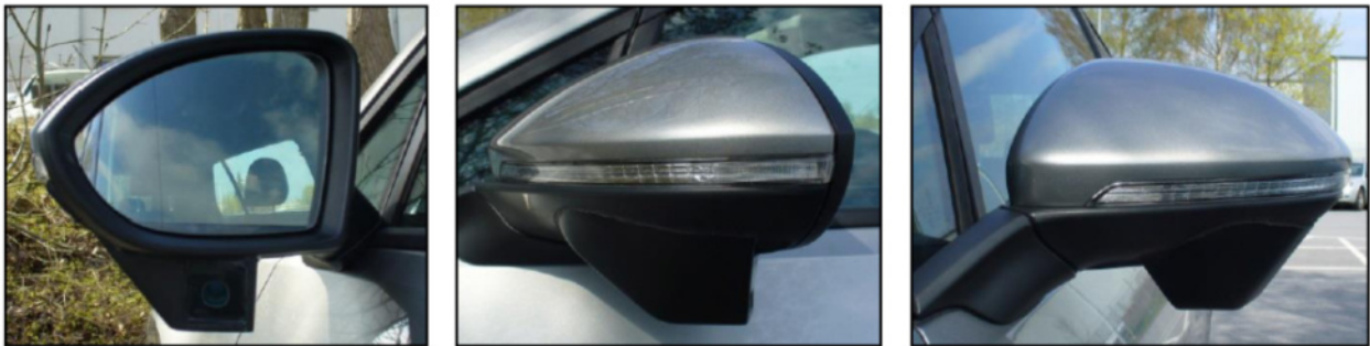
Figure 3: Left exterior mirror with camera mounted to the mirror housing.
