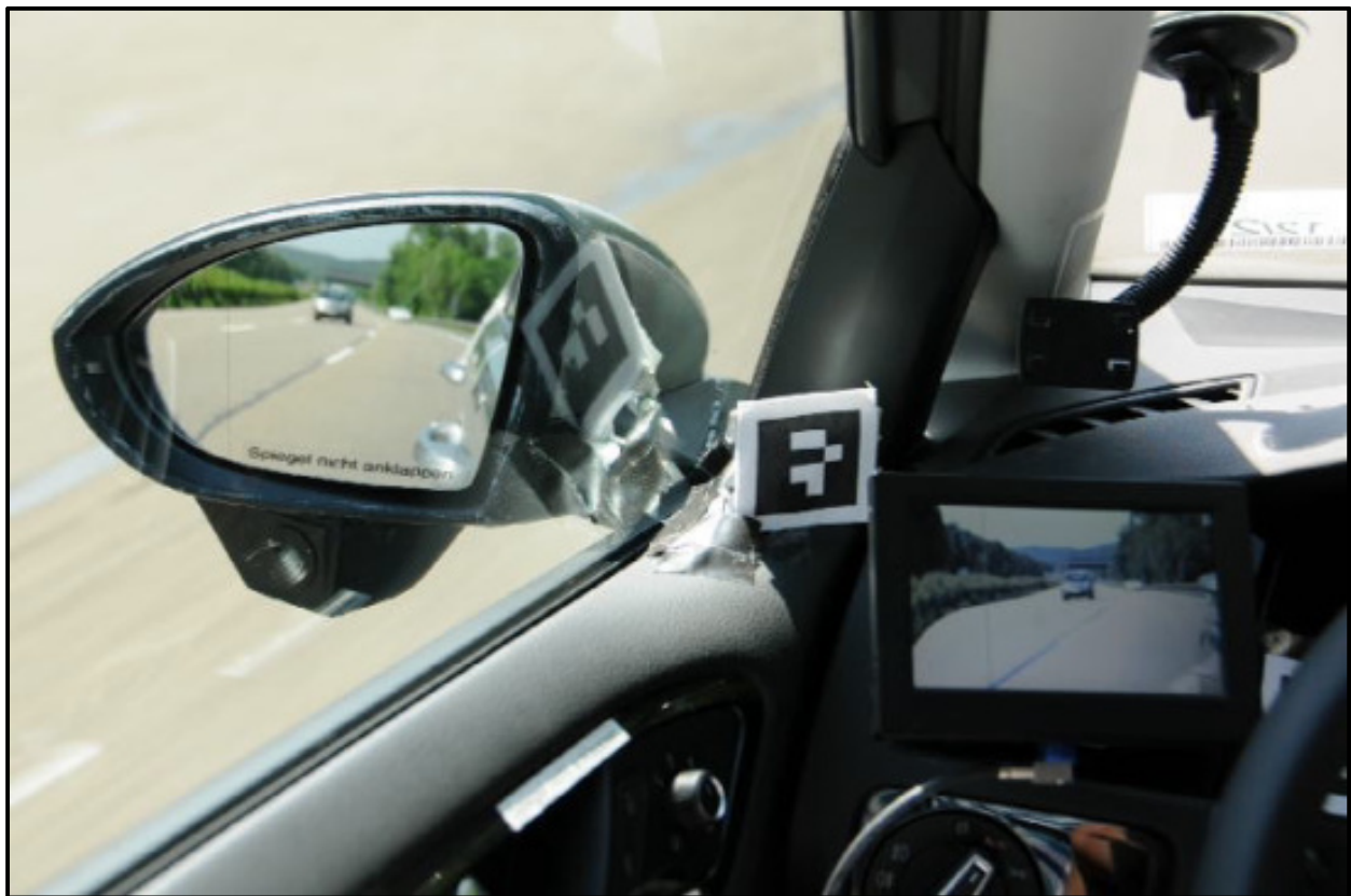
Figure 18: Difficult to detect vehicle in the background (white vehicle on beige concrete carriageway).
