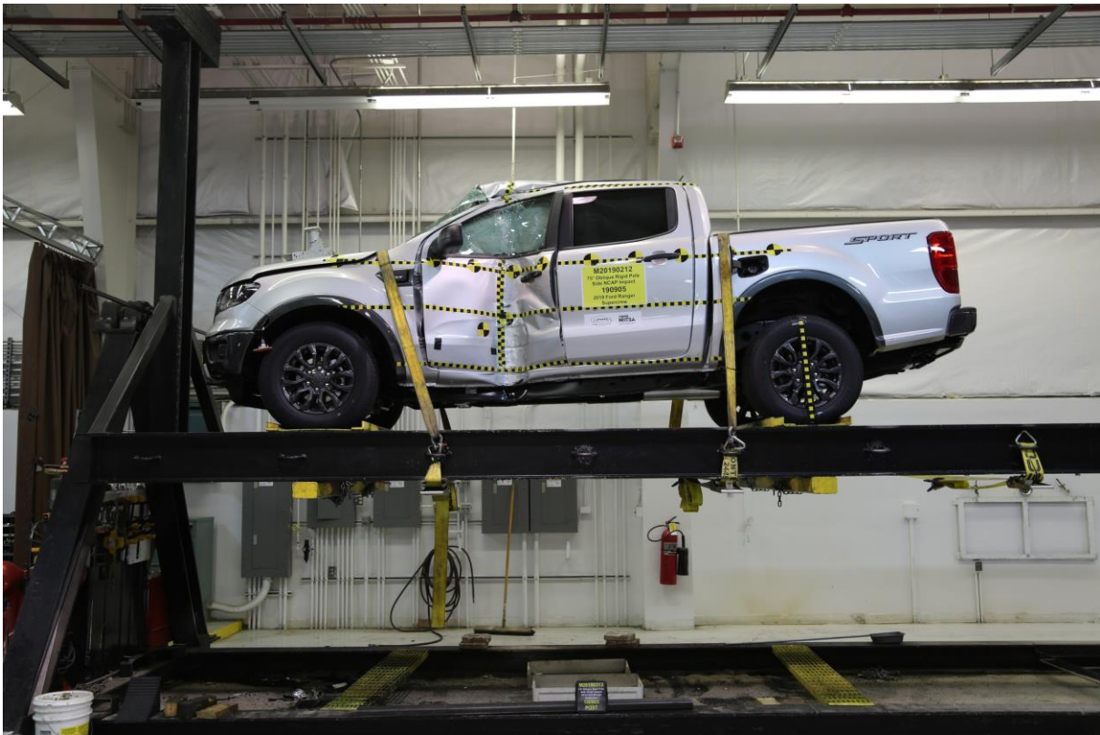
No. 063 FMVSS No. 301 Static Rollover 0 Degrees
