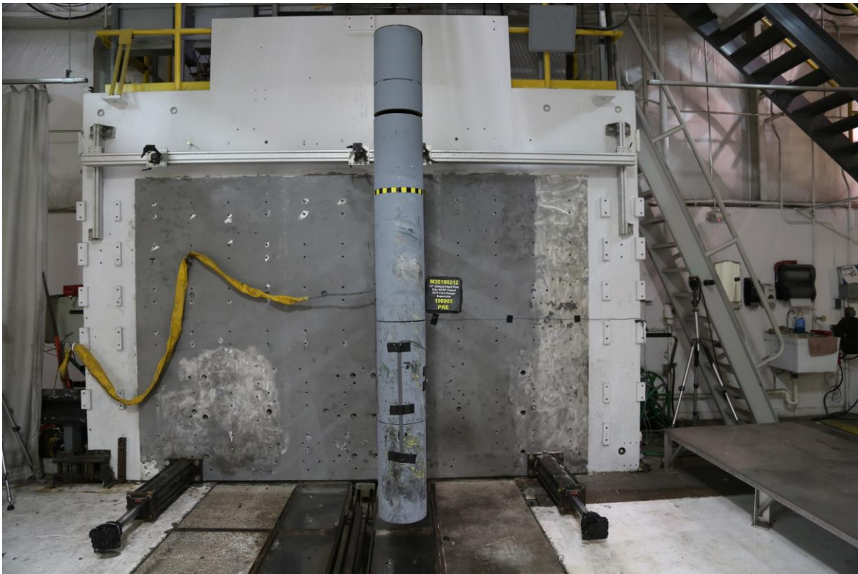
No. 057 Pre-Test Pole Barrier Front View
