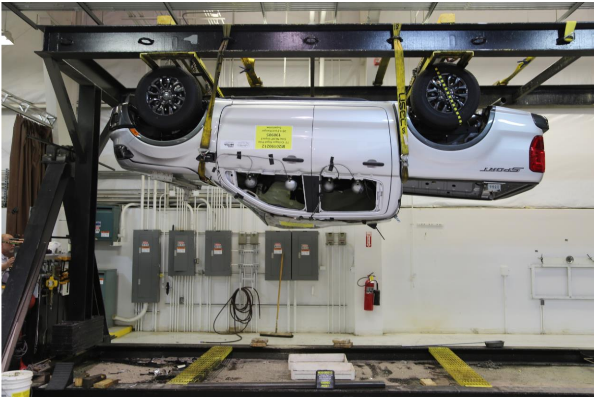
No. 065 FMVSS No. 301 Static Rollover 180 Degrees
