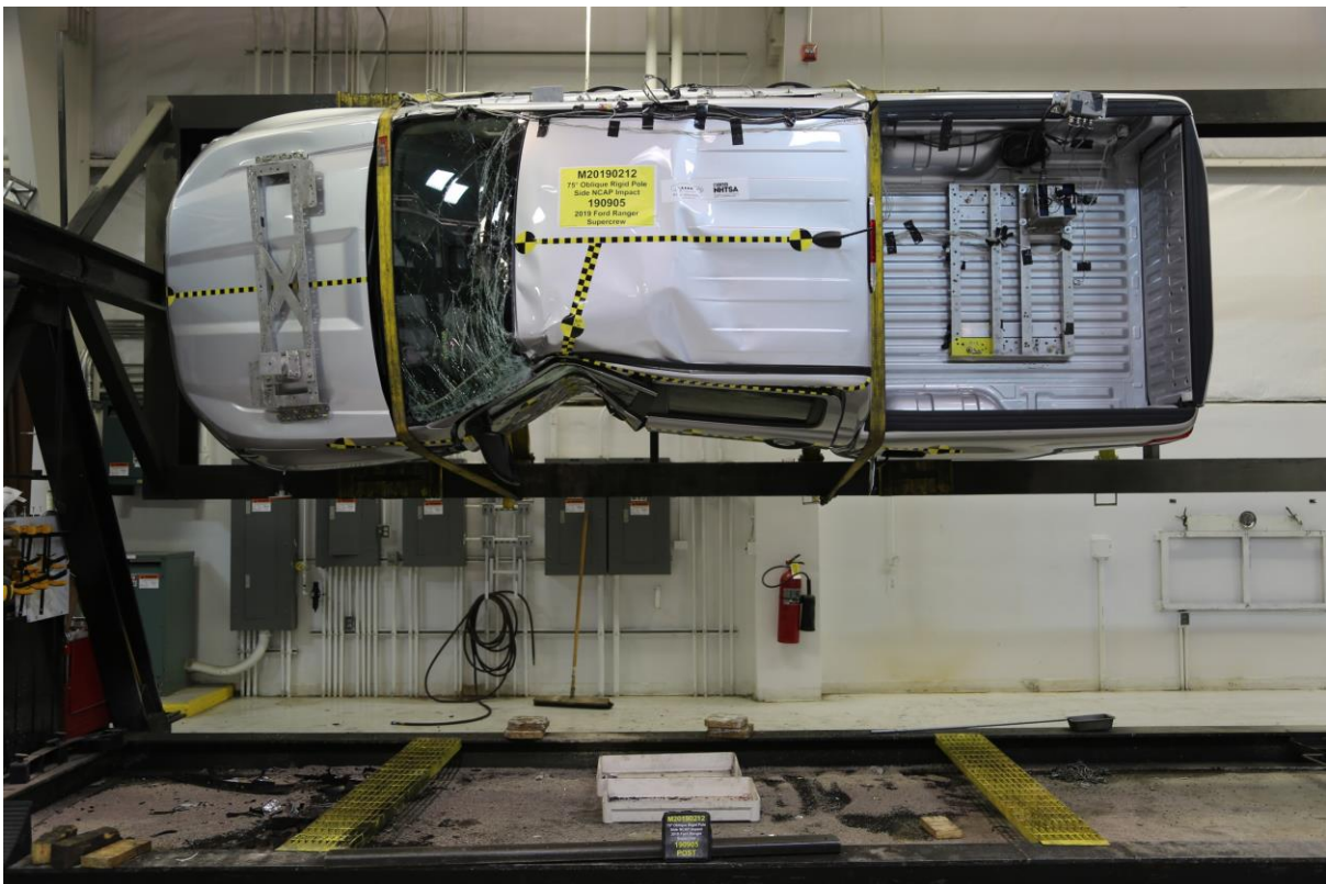
No. 064 FMVSS No. 301 Static Rollover 90 Degrees
