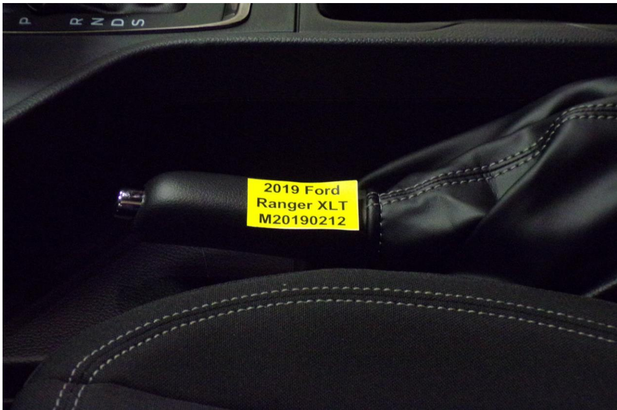
No. 035 Pre-Test View of Disengaged Parking Brake
