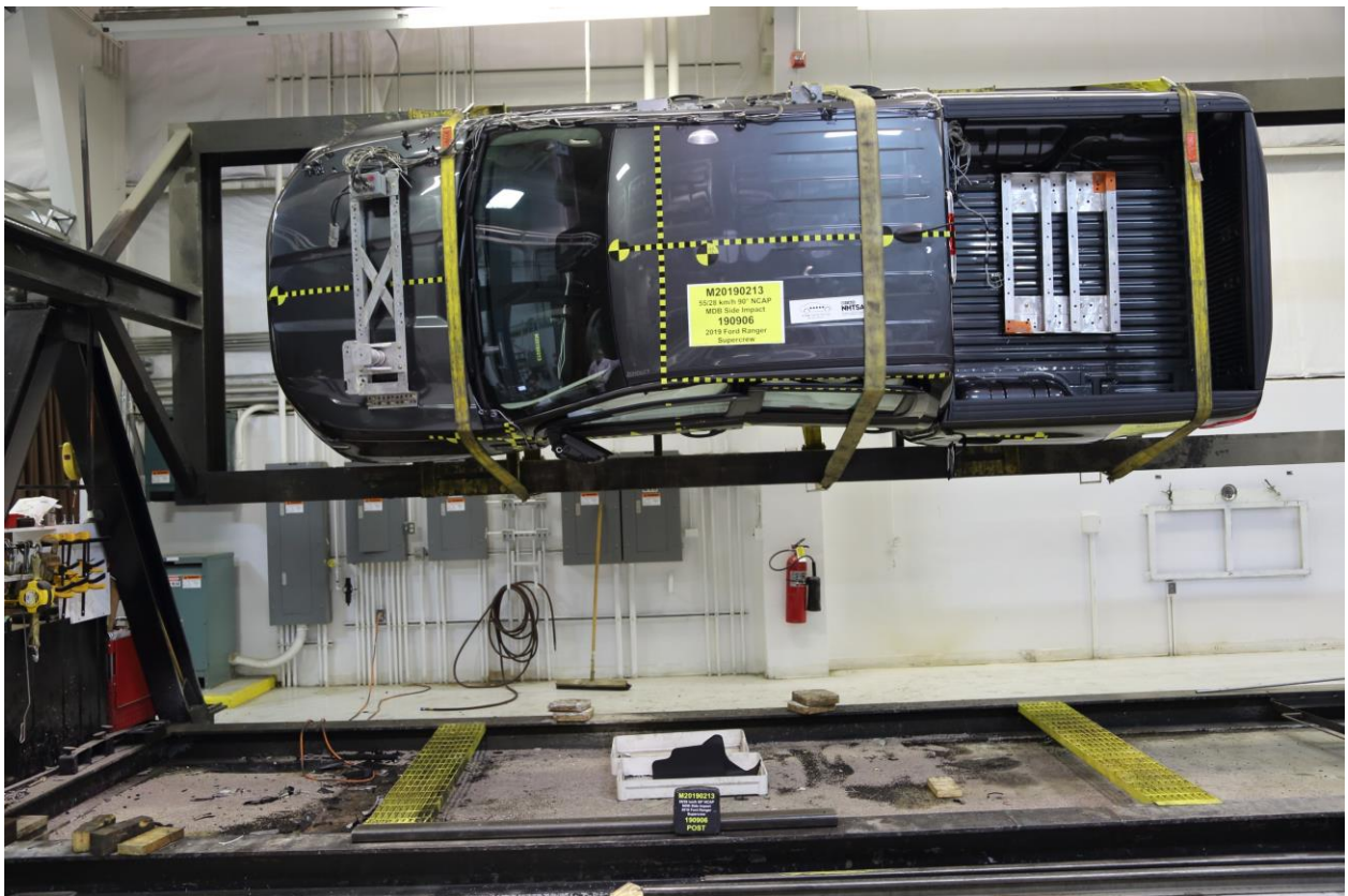
097 FMVSS No. 301 Static Rollover 90 Degrees
