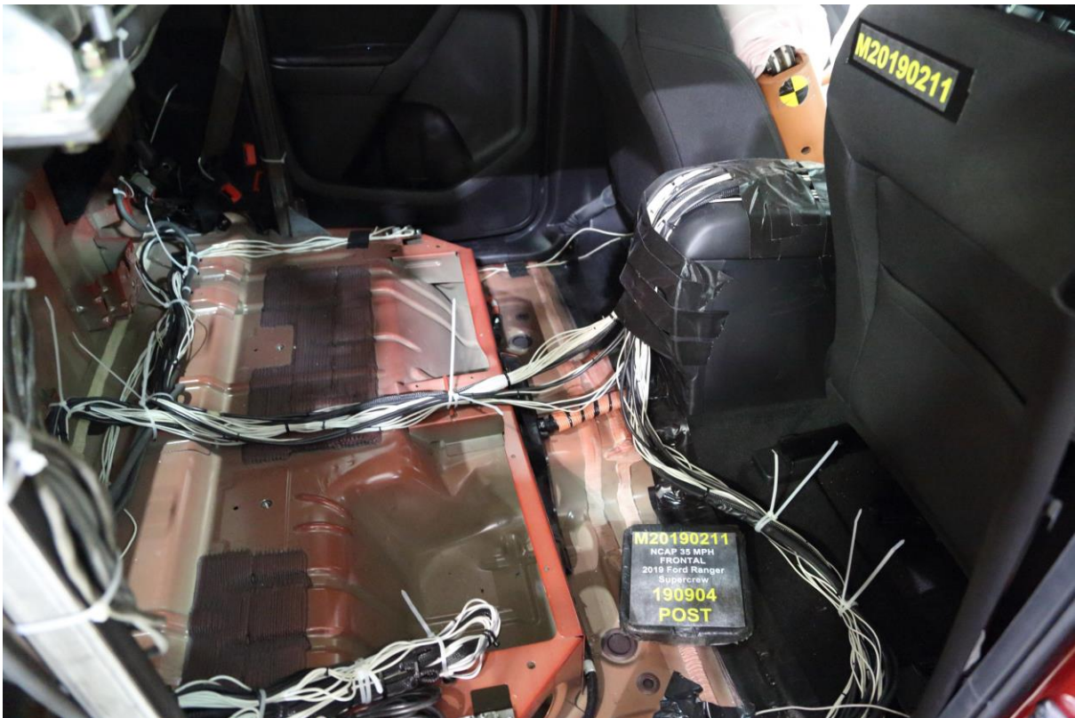
029 Post-Test Dummy Cable Routing
