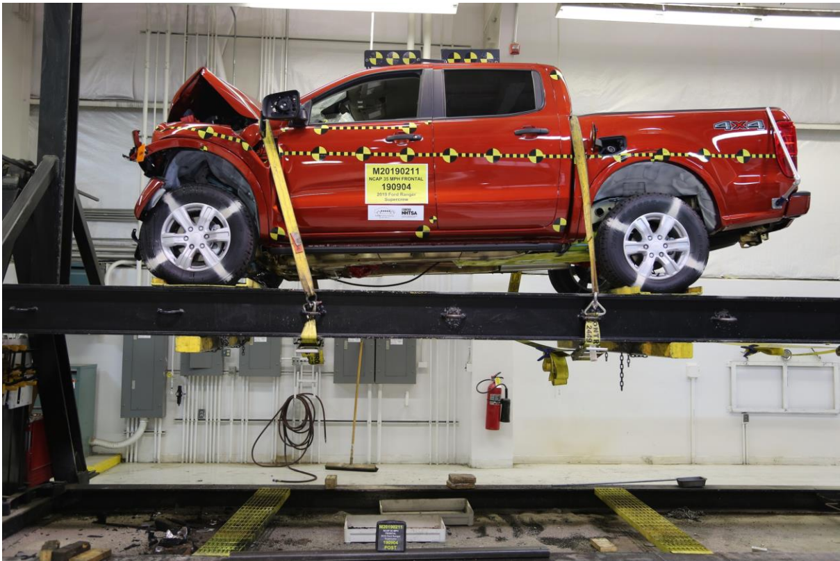
081 Vehicle at 360° on Static Rollover Device
