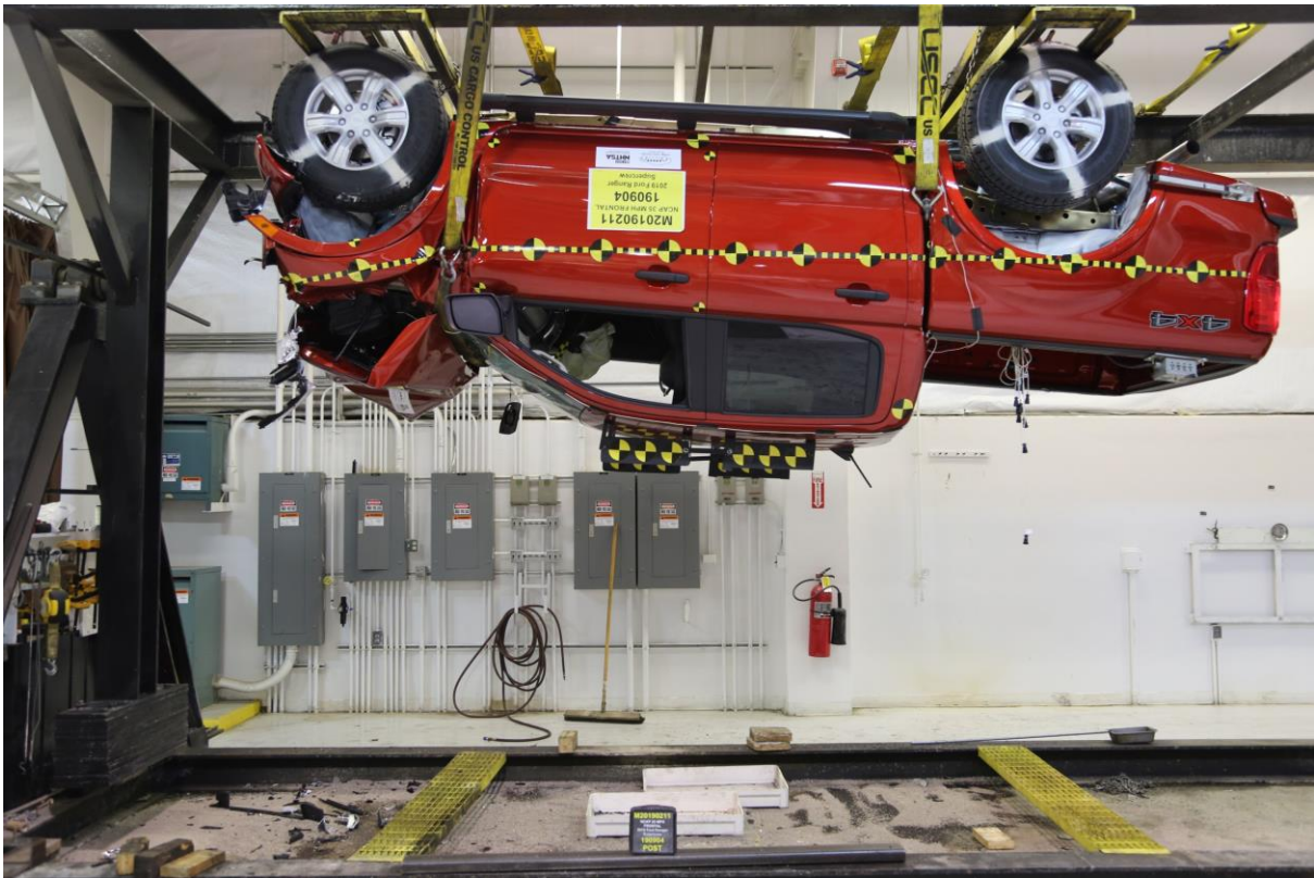
079 Vehicle at 180° on Static Rollover Device
