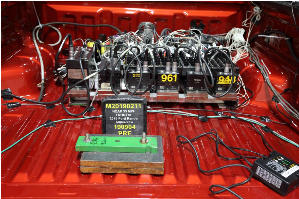
074 Photograph of Ballast Installed in Vehicle
