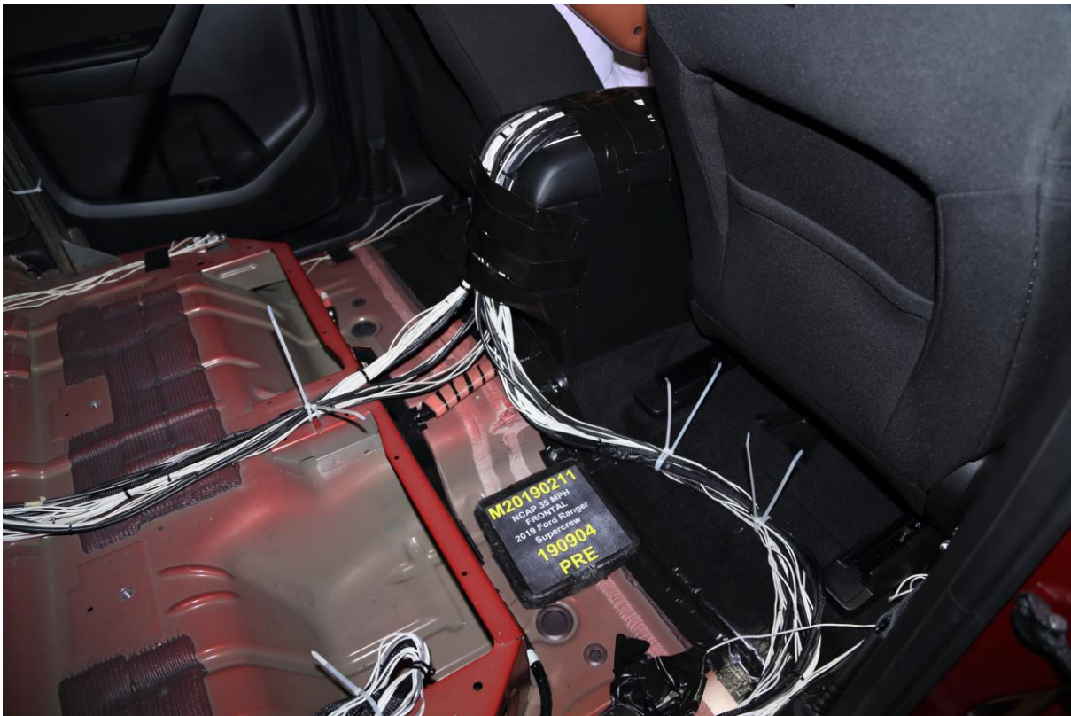
028 Pre-Test Dummy Cable Routing
