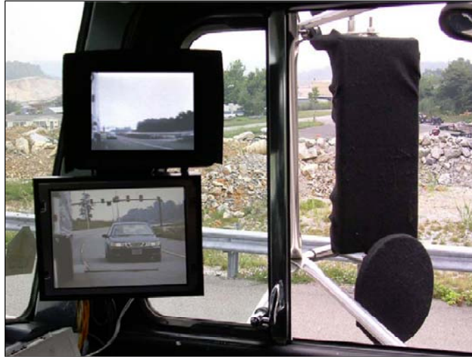
Figure 40. Passenger-Side Monitors Mounted at the A-pillar; Note the Covers Over the Mirrors, and also Note that the Upper Monitor was Hooded to Reduce Glare, Taken from Wierwille, Schaudt, Spaulding, et al. (2008)
