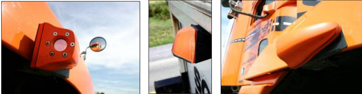
Figure 3. Placement of A-C/VIS Fender and Trailer Cameras
