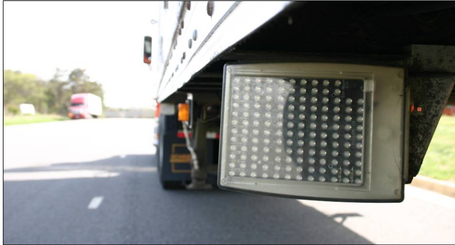
Figure 7. Infrared Illuminators Mounted on Truck and Trailer
