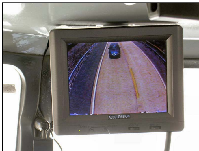
Figure 38. Peterbilt In-Cab Monitor for the Wide-Angle Rear Multipurpose Trailer Look-Down C/VIS, Taken from Wierwille, Schaudt, Spaulding, et al. (2008)
