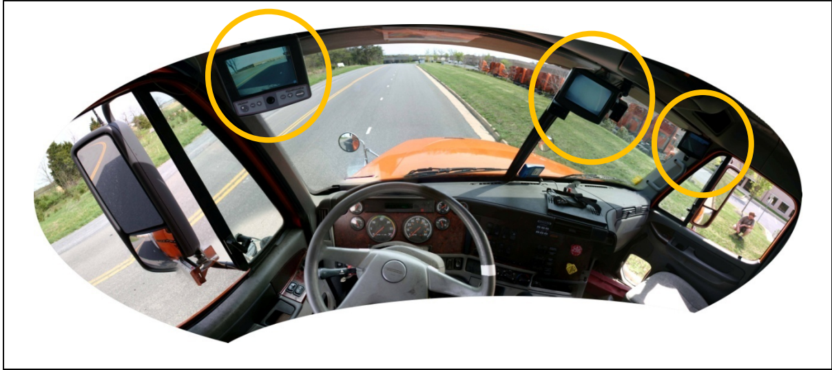
Figure 5. Placement of A-C/VIS Monitors in Truck Cab
