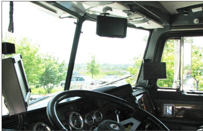
Figure 25. Placement of E-C/VIS Monitors in Truck Cabin, Taken from Wierwille et al. (in press)
