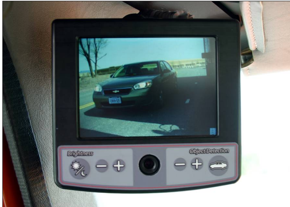
Figure 31. The A-C/VIS DVI Built Into the Left Monitor
