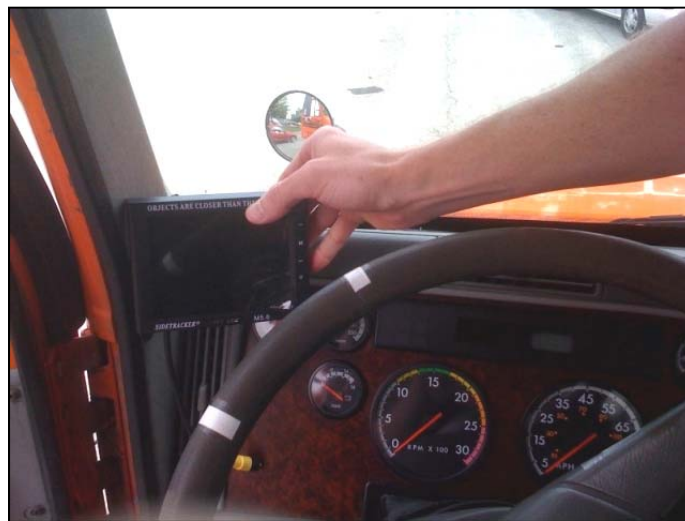
Figure 222. Potential Placement of Commercial C/VIS's Left Monitor to Avoid Potential Obstruction of Left Fender Mirror; Elements of the Instrument Panel and Window Defroster are Obstructed
