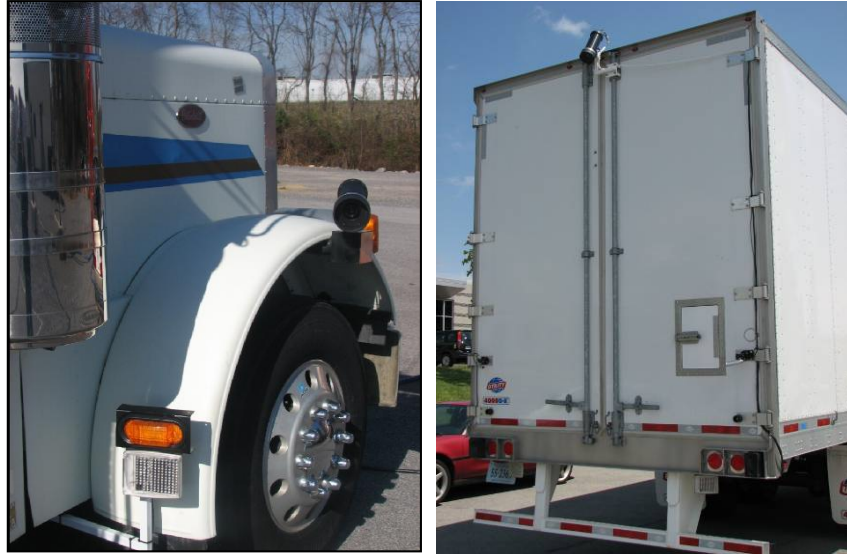
Figure 24. Placement of E-C/VIS Fender and Trailer Cameras, Taken from Wierwille et al. (in press)
