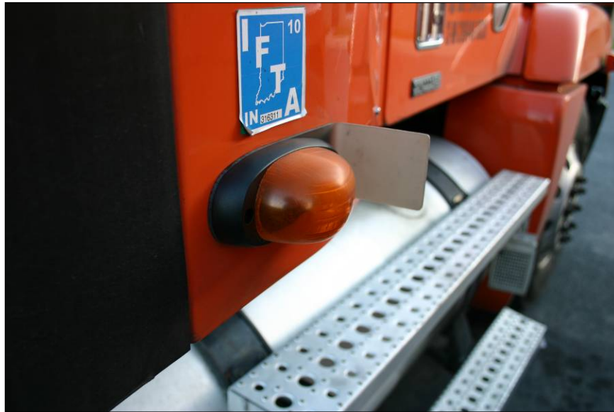
Figure 89. A-C/VIS Light Diffuser Mounted in Front of Right Turn Signal
