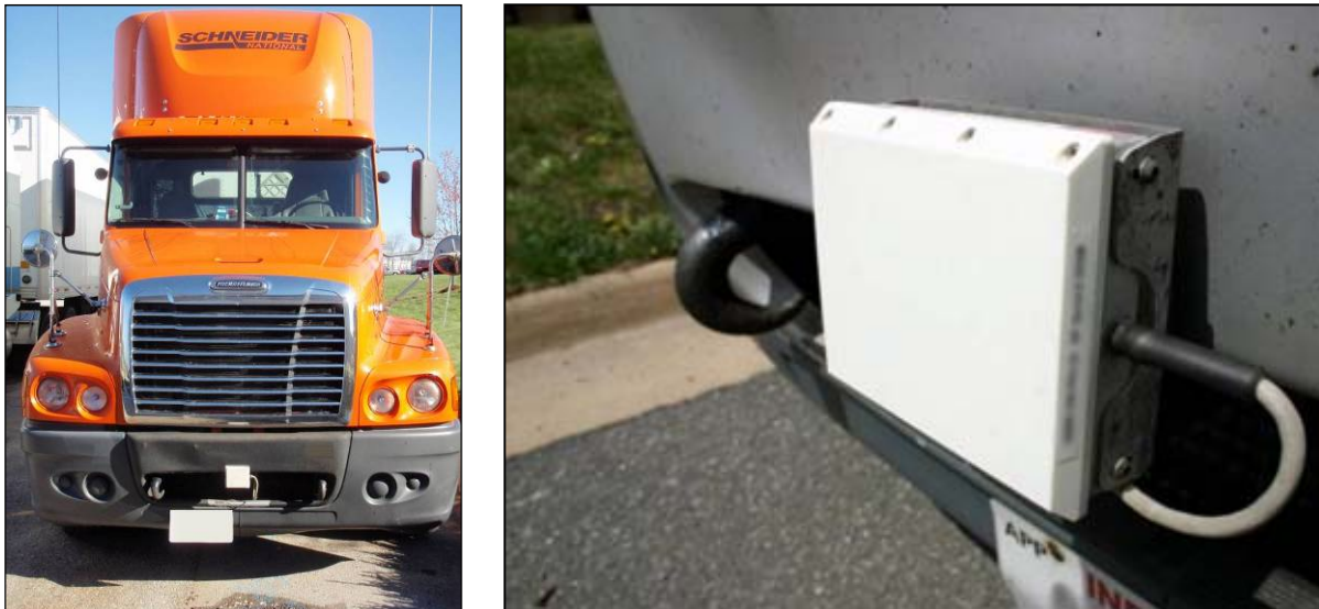
Figure 97. Radar Unit Mounted on the Front of the Truck (Left) and Close View of Radar Unit Mounted on the Front of the Truck (Right)
