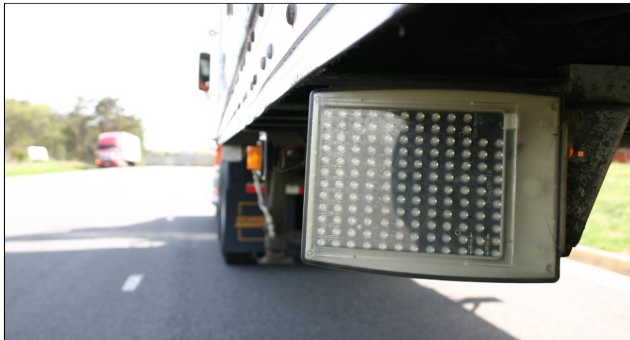
Figure 32. Infrared Illuminators Mounted on Truck and Trailer
