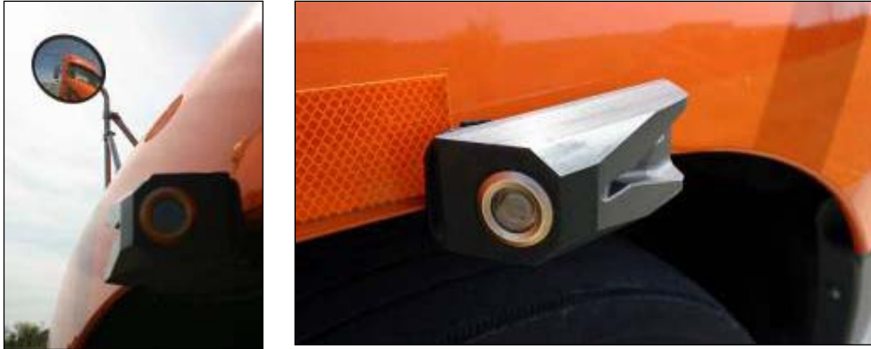
Figure 8. Placement of Commercial C/VIS's Cameras on Left and Right Fenders
