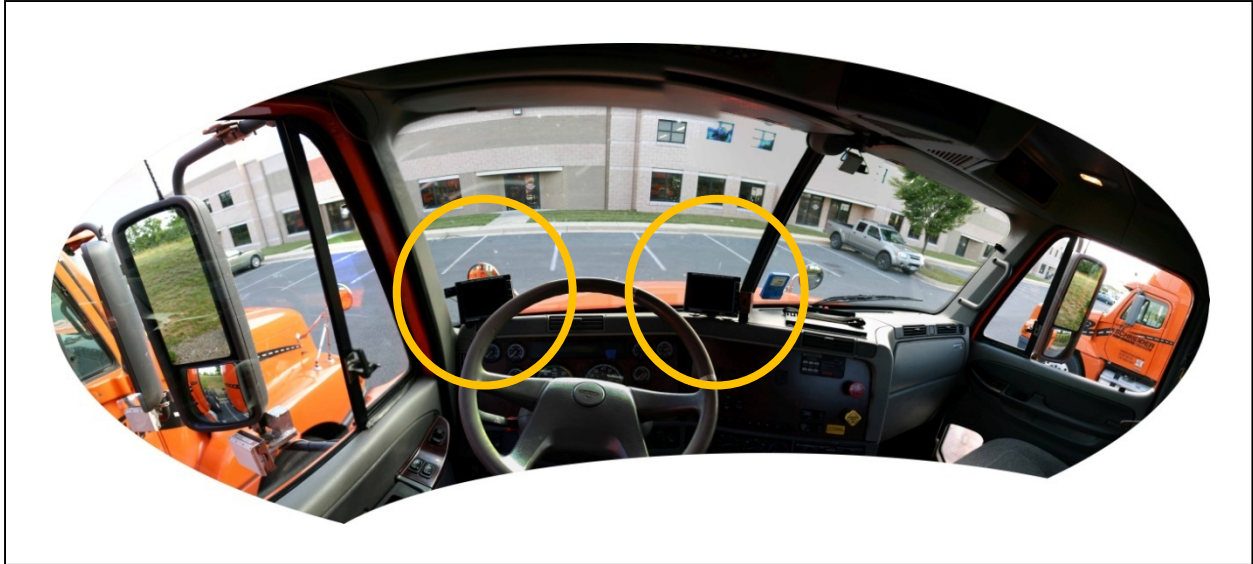
Figure 10. Placement of Commercial C/VIS's Monitors on Truck Dash
