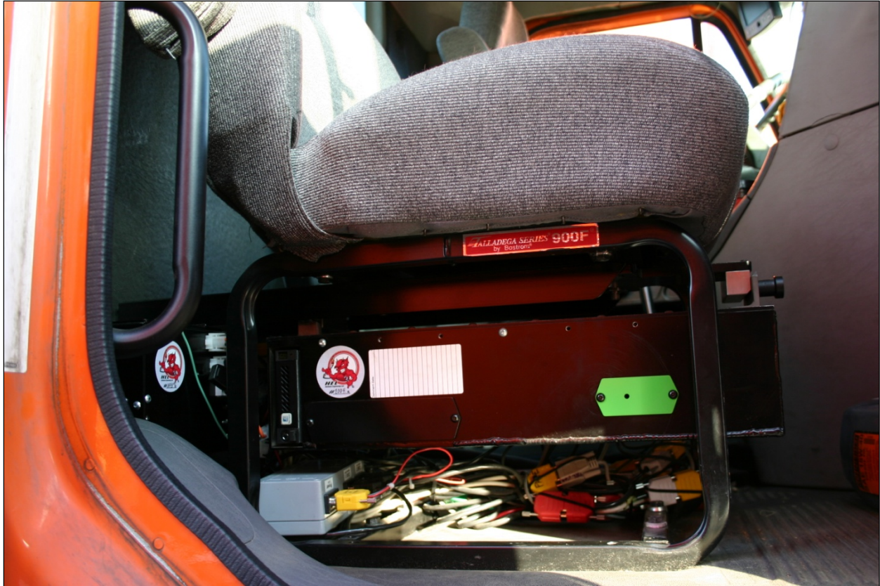
Figure 94. The DAS Unit Installed Under the Passenger Seat
