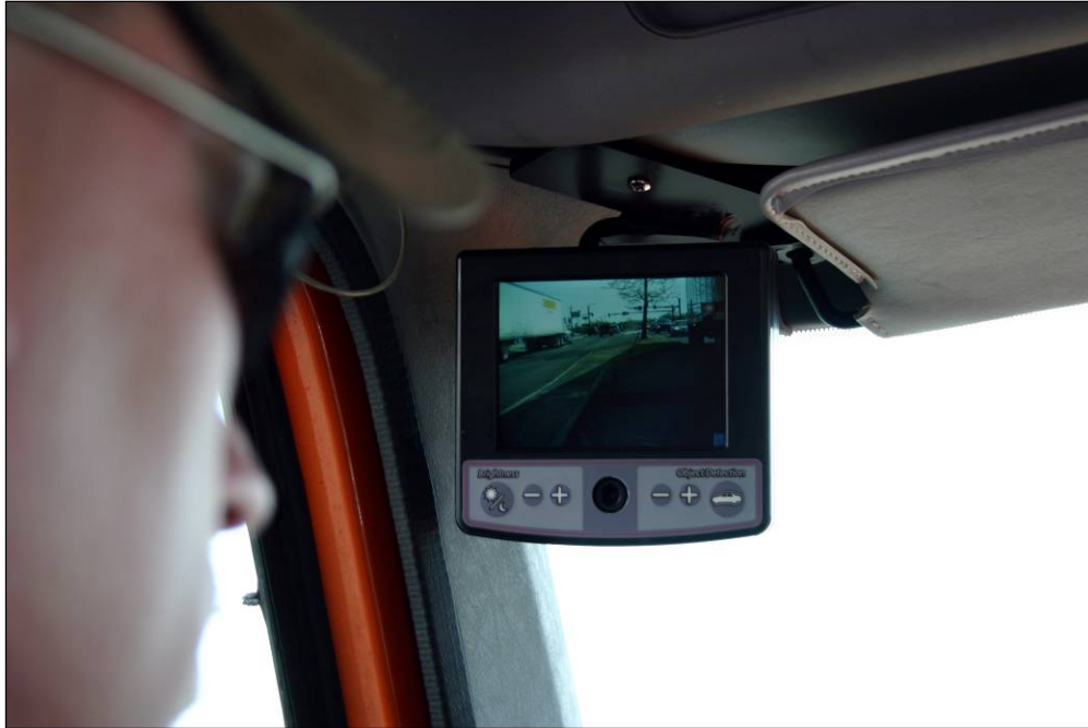
Figure 62. View of DVI on Left Monitor Housing
