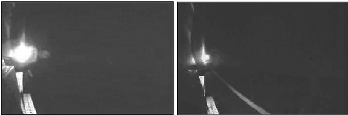
Figure 92. Left: Commercial C/VIS Monitor Showing Side Marker Light without Light Diffuser; Right: Commercial C/VIS Monitor Showing Side Marker Light with Light Diffuser
