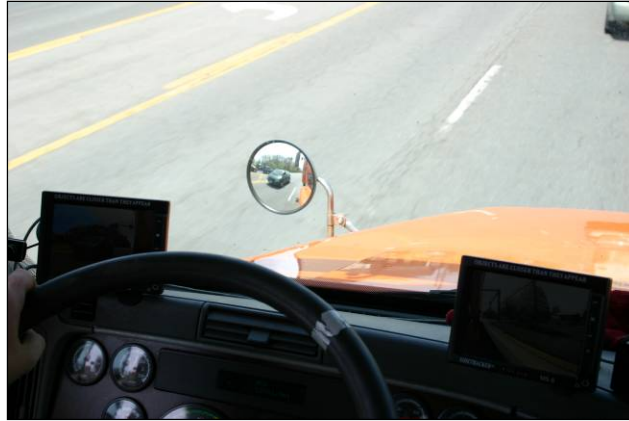
Figure 23. Placement of Commercial C/VIS's Monitors on Truck Dash
