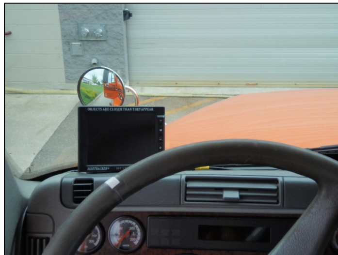
Figure 20. Placement of Commercial C/VIS's Left Monitor, According to VTECH USA, LLC Specification
