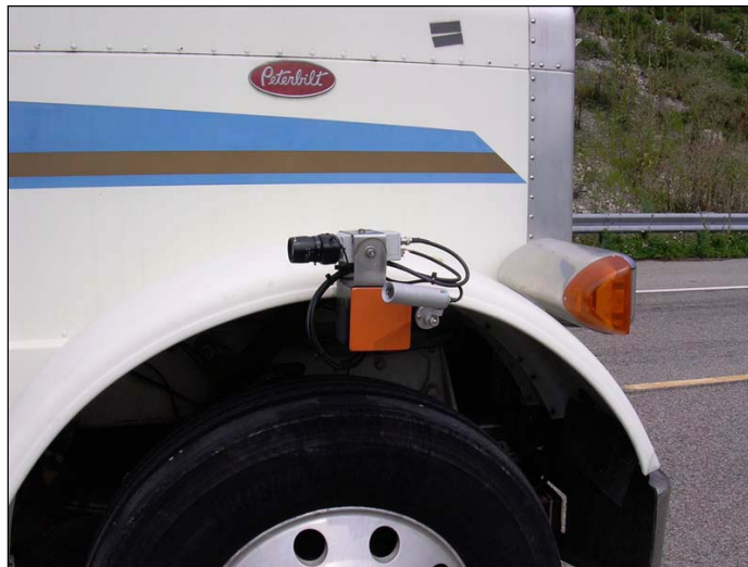
Figure 42. Passenger-Side Cameras at the Front Fender; the Round Camera is for the Convex Mirror Surrogate, and the Rectangular Camera is for the West Coast Mirror Surrogate, Taken from Wierwille, Schaudt, Spaulding, et al. (2008)
