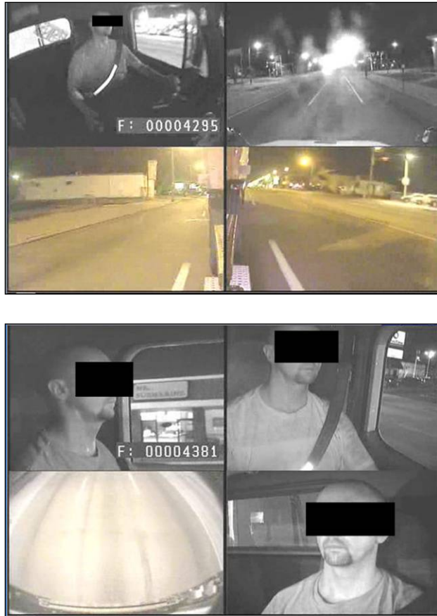
Figure 95. Eight A-C/VIS Camera Images Multiplexed into Two Images
