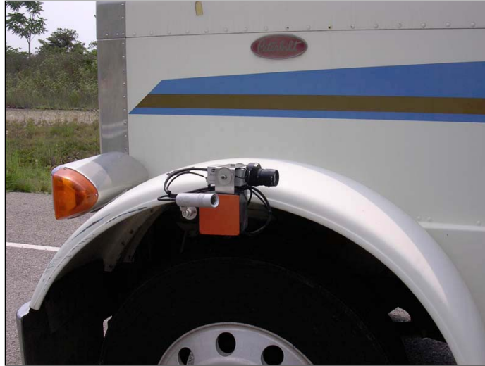
Figure 41. Driver-Side Cameras at the Front Fender; the Round Camera is for the Convex Mirror Surrogate, and the Rectangular Camera is for the West Coast Mirror Surrogate, Taken from Wierwille, Schaudt, Spaulding, et al. (2008)
