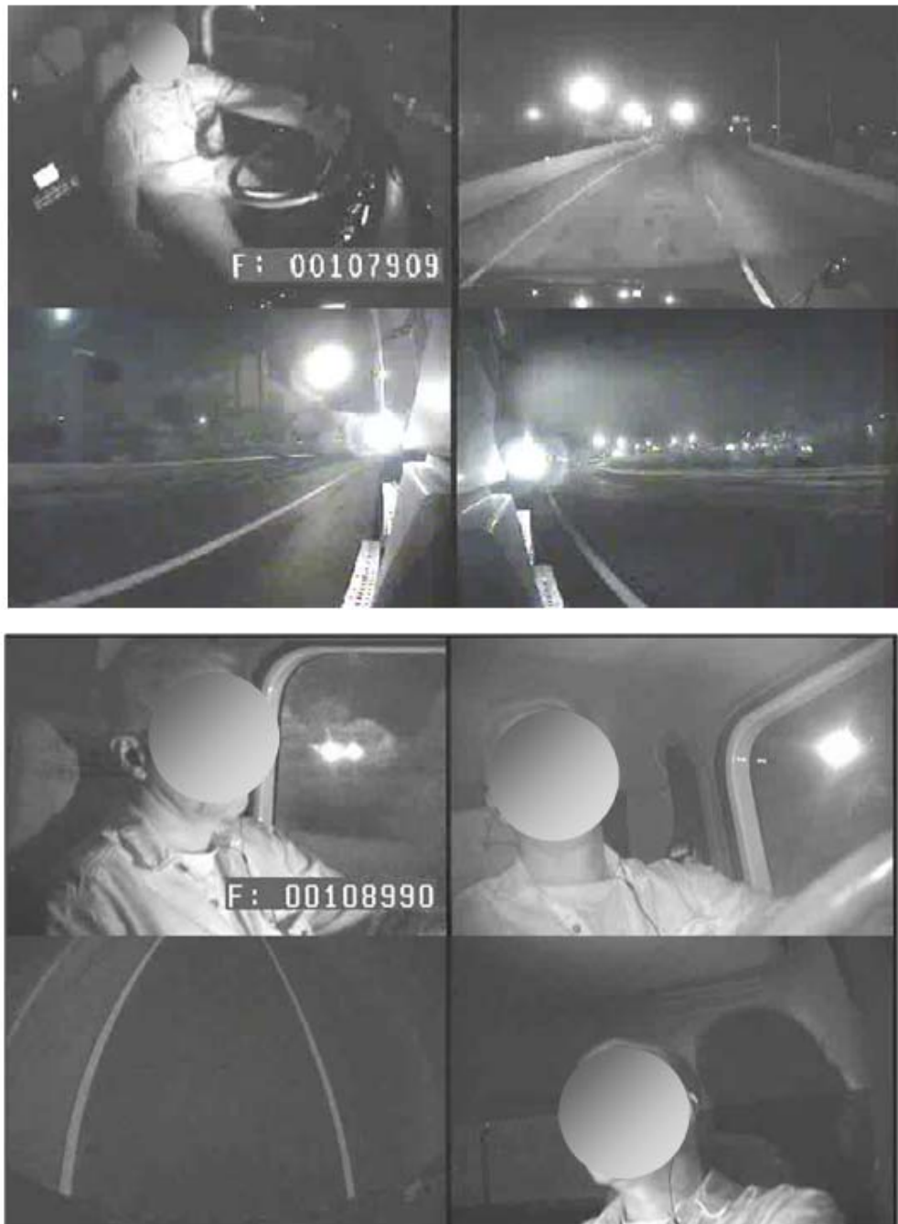
Figure 96. Eight Commercial C/VIS Camera Images Multiplexed into Two Images
