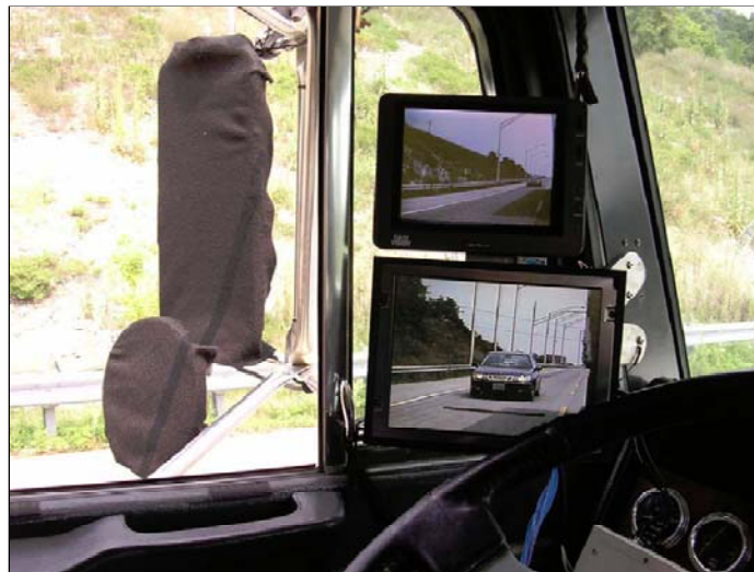
Figure 39. Driver-Side Monitors Mounted at the A-pillar; Note the Covers Over the Mirrors, Taken from Wierwille, Schaudt, Spaulding, et al. (2008)
