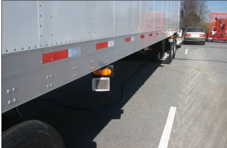
Figure 26. Placement of E-C/VIS Infrared Illuminators, Taken from Wierwille et al. (in press)
