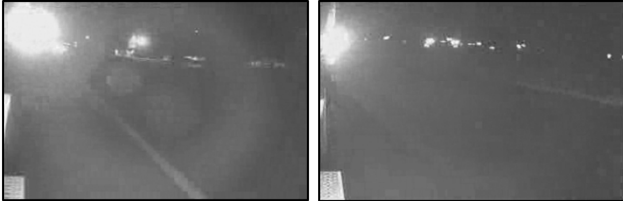
Figure 18. Left: A-C/VIS Monitor Image of Turn Signal Activation without Light Diffuser; Right: A-C/VIS Monitor Image of Turn Signal Activation with Light Diffuser
