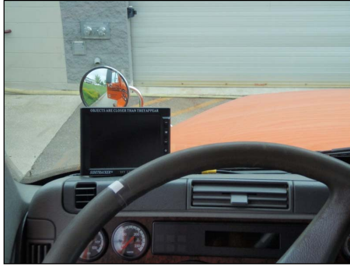
Figure 221. Placement of Commercial C/VIS's Left Monitor According to VTECH USA, LLC Specification
