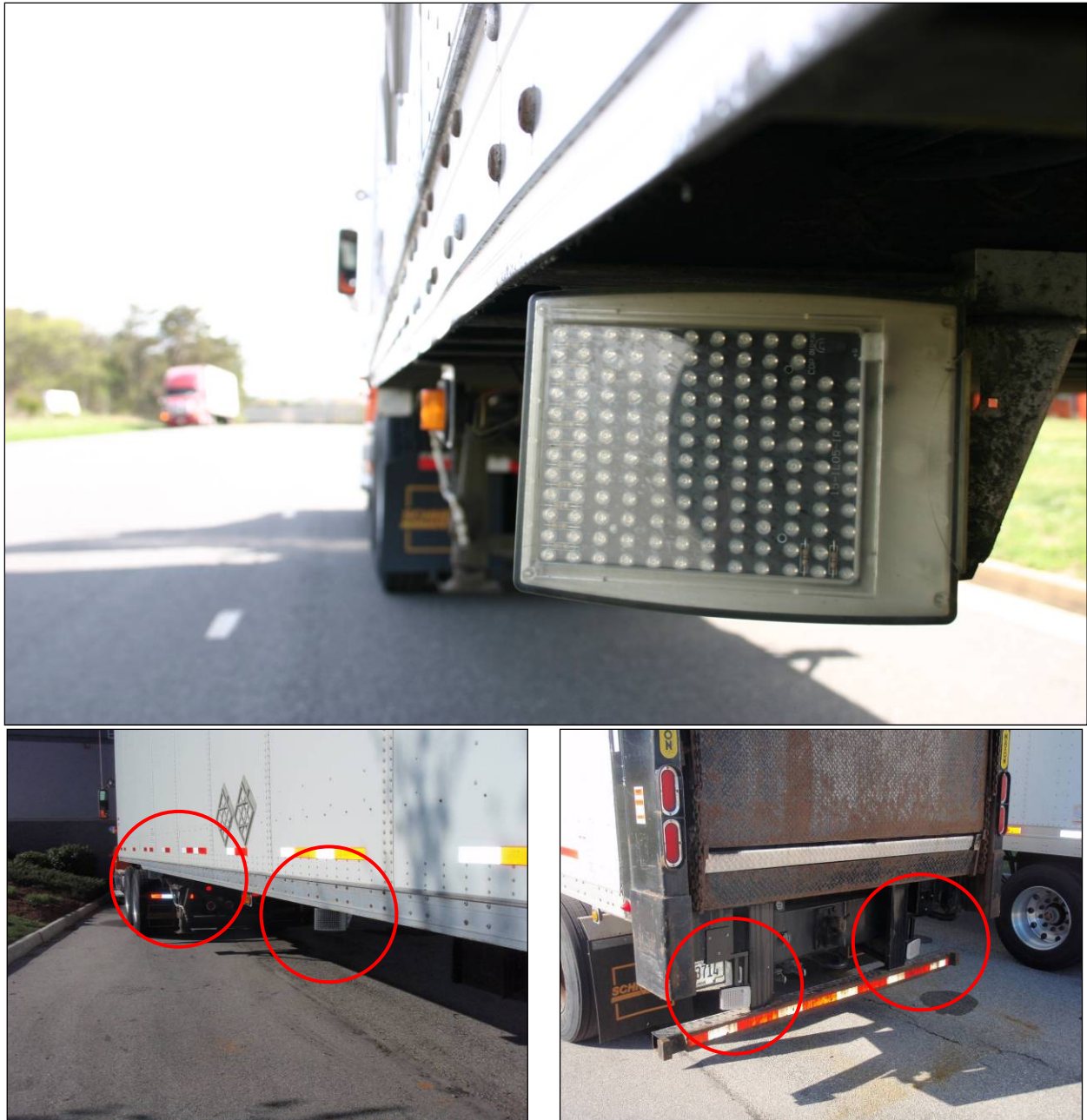
Figure 52. IR Illuminators Mounted Underneath Trailer
