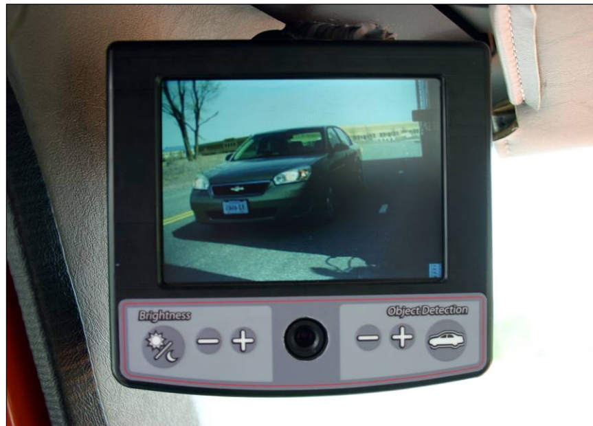
Figure 6. The A-C/VIS DVI Built Into the Left Monitor
