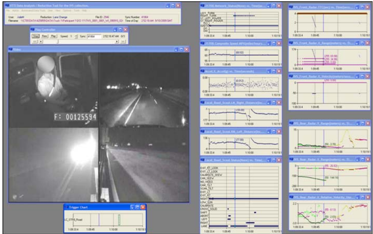
Figure 108. Example of the Data Charts Referenced During Application of the Lane Change Summary Measure Directory. Referenced Views Include Front and Rear Radar Parameters, Turn Signal Indicators, and Lane Marking Distance Measures
