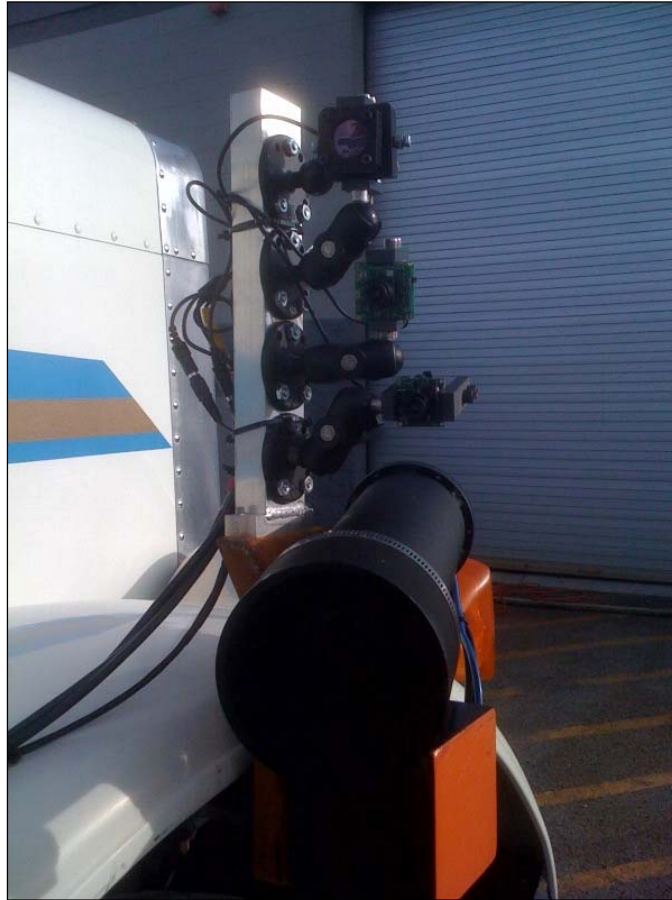
Figure 51. Candidate Cameras Mounted to Fender of Test Truck
