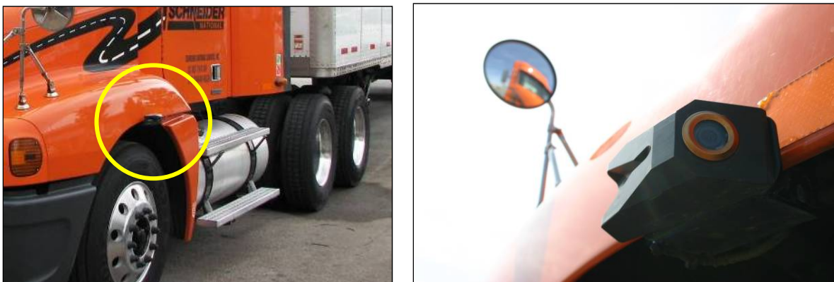
Figure 22. Placement of Commercial C/VIS's Cameras on Left Fender
