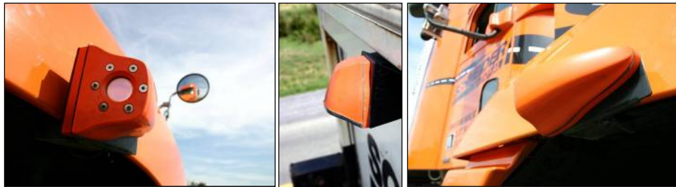
Figure 28. Placement of A-C/VIS Fender and Trailer Cameras
