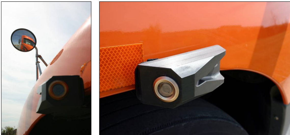
Figure 74. Commercial C/VIS Camera and Weatherproof Housing Installation
