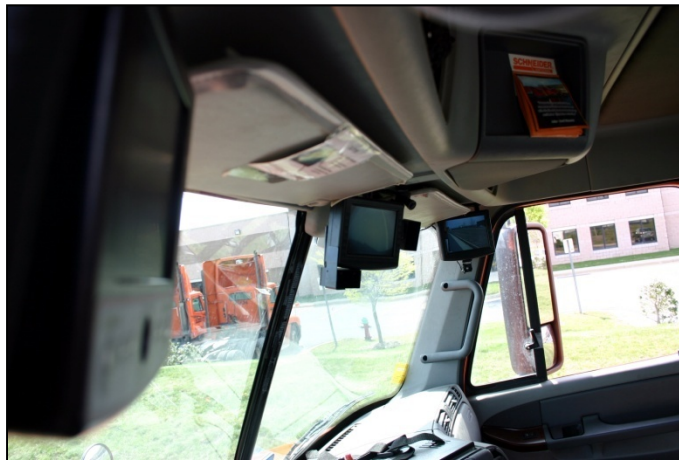
Figure 220. Placement of A-C/VIS Monitors in Truck Cab
