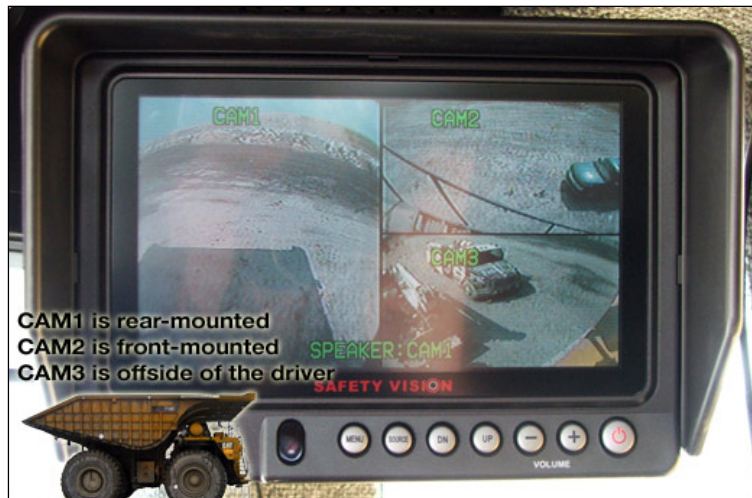
Figure 64. Safety Vision® On-board Camera System (Source: http://www.electricmotorsvc.com/safety/ )
