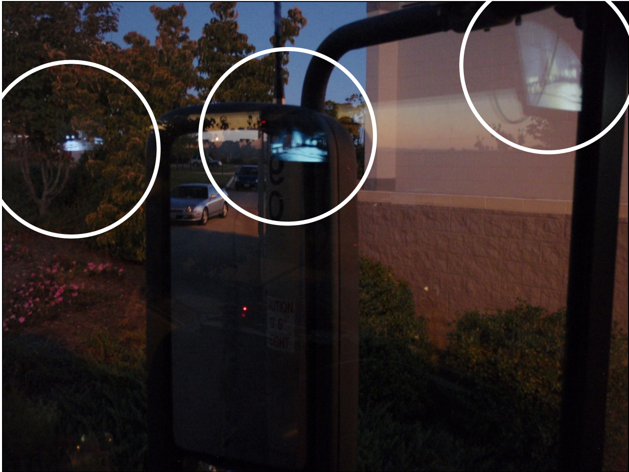
Figure 60. Cross Reflection Produced by A-C/VIS Monitors on the Left Side Window
