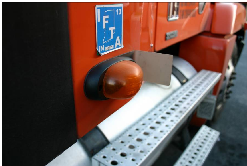
Figure 17. A-C/VIS Light Diffuser Mounted in Front of Right Turn Signal
