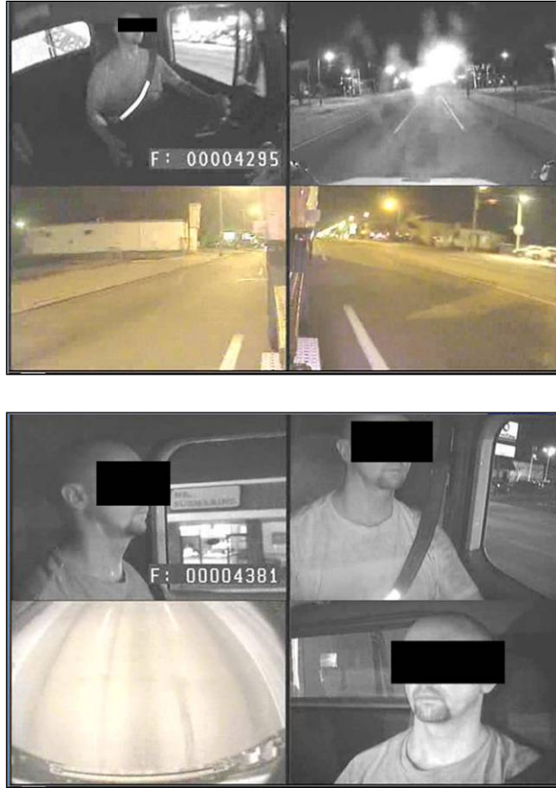
Figure 15. Eight Camera Images Multiplexed into Two Images
