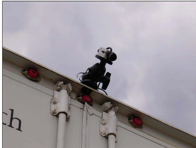
Figure 37. Wide-Angle Rear Multipurpose Look-Down Camera at Back of Trailer, Taken from Wierwille, Schaudt, Spaulding, et al. (2008)
