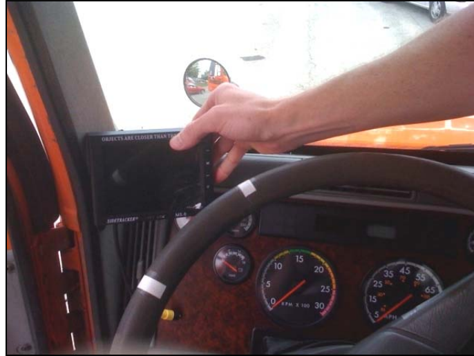
Figure 21. Potential Placement of Commercial C/VIS's Left Monitor to Avoid Potential Obstruction of Left Fender Mirror; Elements of the Instrument Panel and Window Defroster are Obstructed
