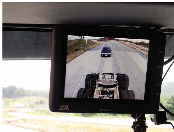
Figure 36. Monitor in Volvo Tractor for Rear-View C/VIS, Taken from Wierwille, Schaudt, Spaulding, et al. (2008)
