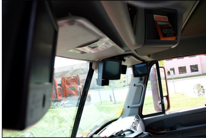
Figure 19. Placement of A-C/VIS Monitors in Truck Cab
