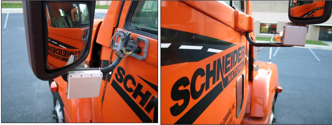
Figure 98. Radar Unit Mounted on the Left and Right West Coast Mirrors
