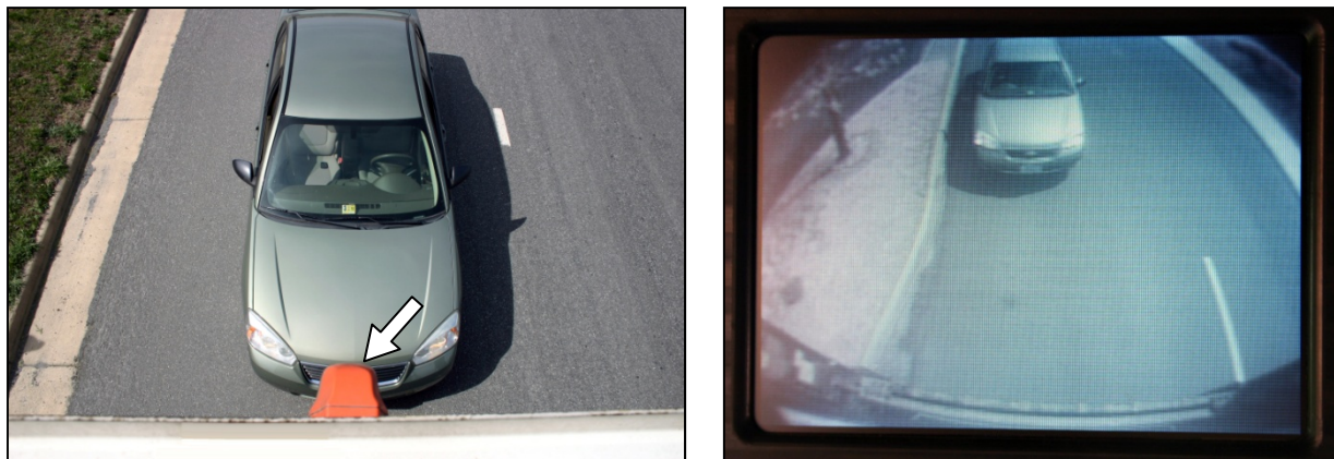
Figure 2. Left: C/VIS Camera Mounted on Trailer; Right: Video Image from C/VIS Camera
