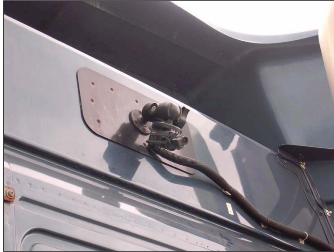
Figure 35. Rear of the Volvo Tractor Cab Showing the Rear-View C/VIS Camera Location, Taken from Wierwille, Schaudt, Spaulding, et al. (2008)
