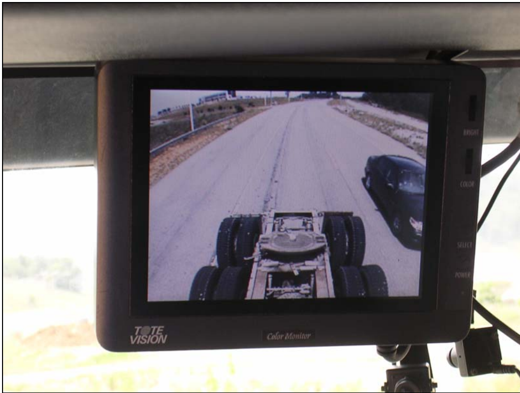
Figure 59. Confederate automobile passing Volvo tractor in the rear-view C/VIS tests.
