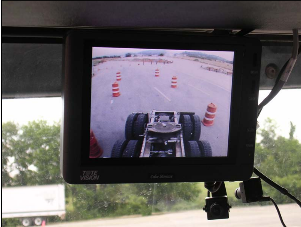
Figure 62. Volvo tractor rear-view monitor during the S-curve backing subtask.
