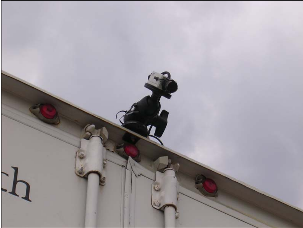
Figure 63. Wide-angle rear multipurpose look-down camera at back of trailer.
