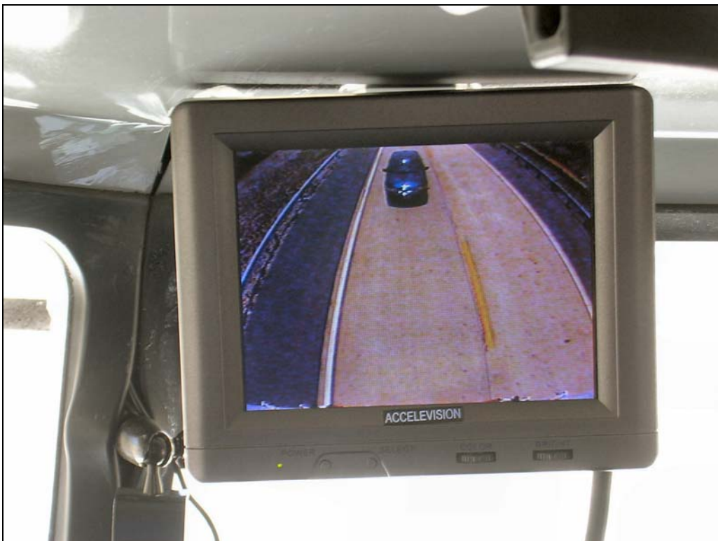
Figure 64. Peterbilt in-cab monitor for the wide-angle rear multipurpose trailer look-down C/VIS.
