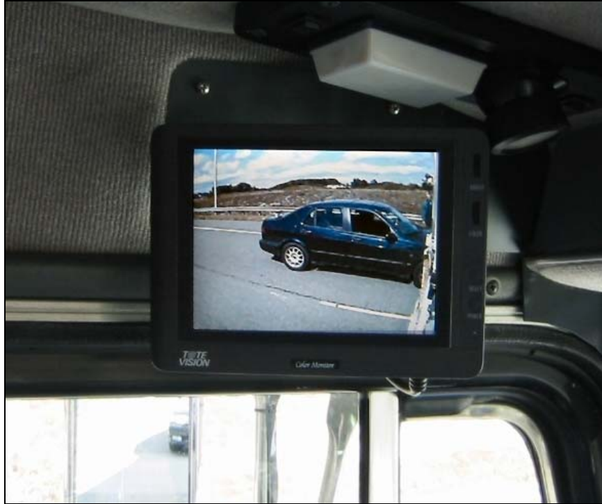
Figure 70. Driver-side monitor for the left merge/re-merge enhancement.
