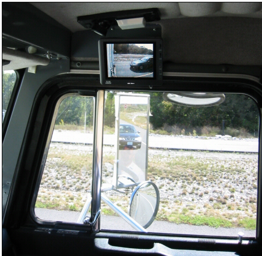
Figure 71. Passenger-side monitor for the right merge/re-merge enhancement.
