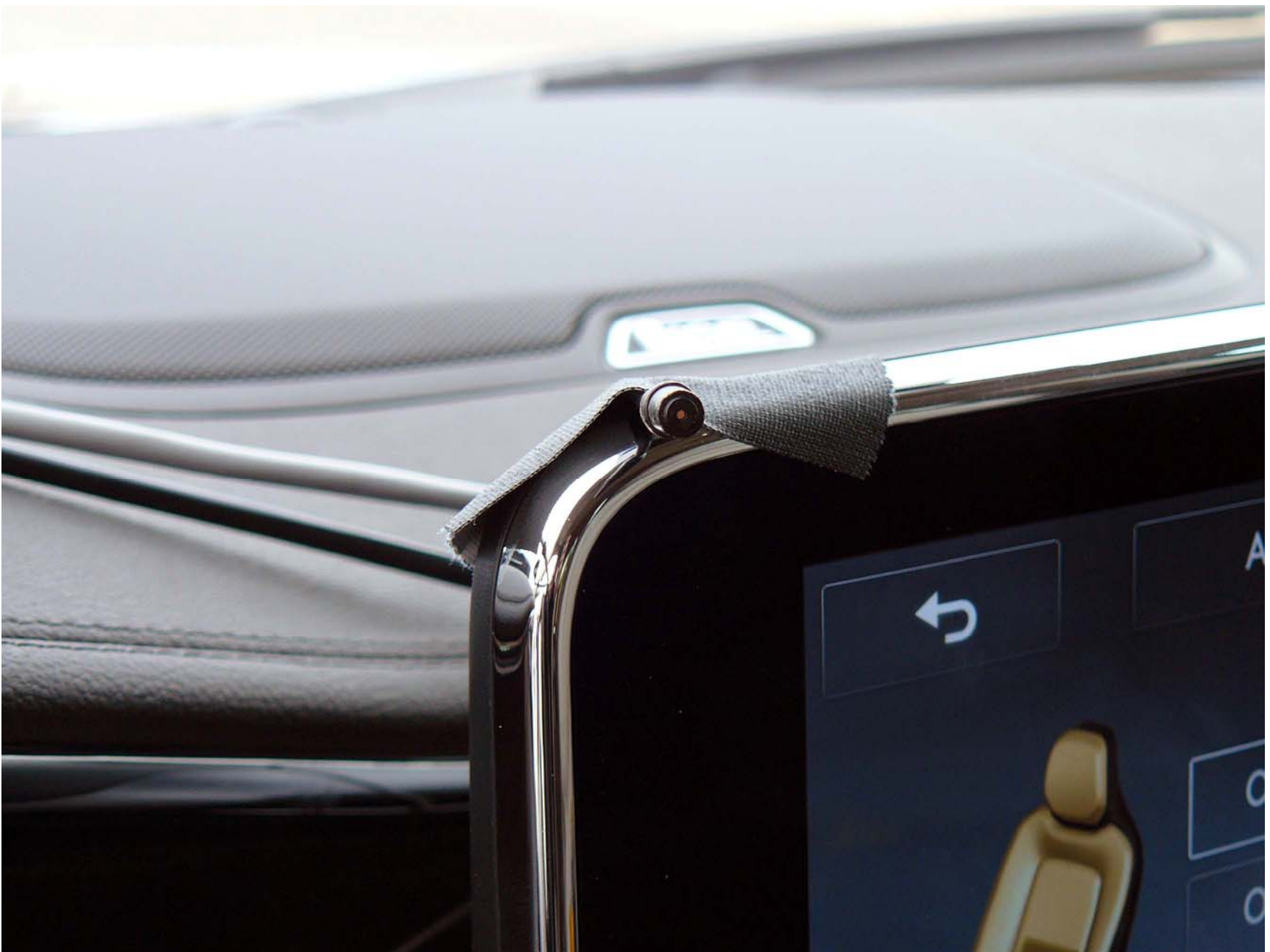
Figure A12. Sensor for Detecting Auditory Alerts
