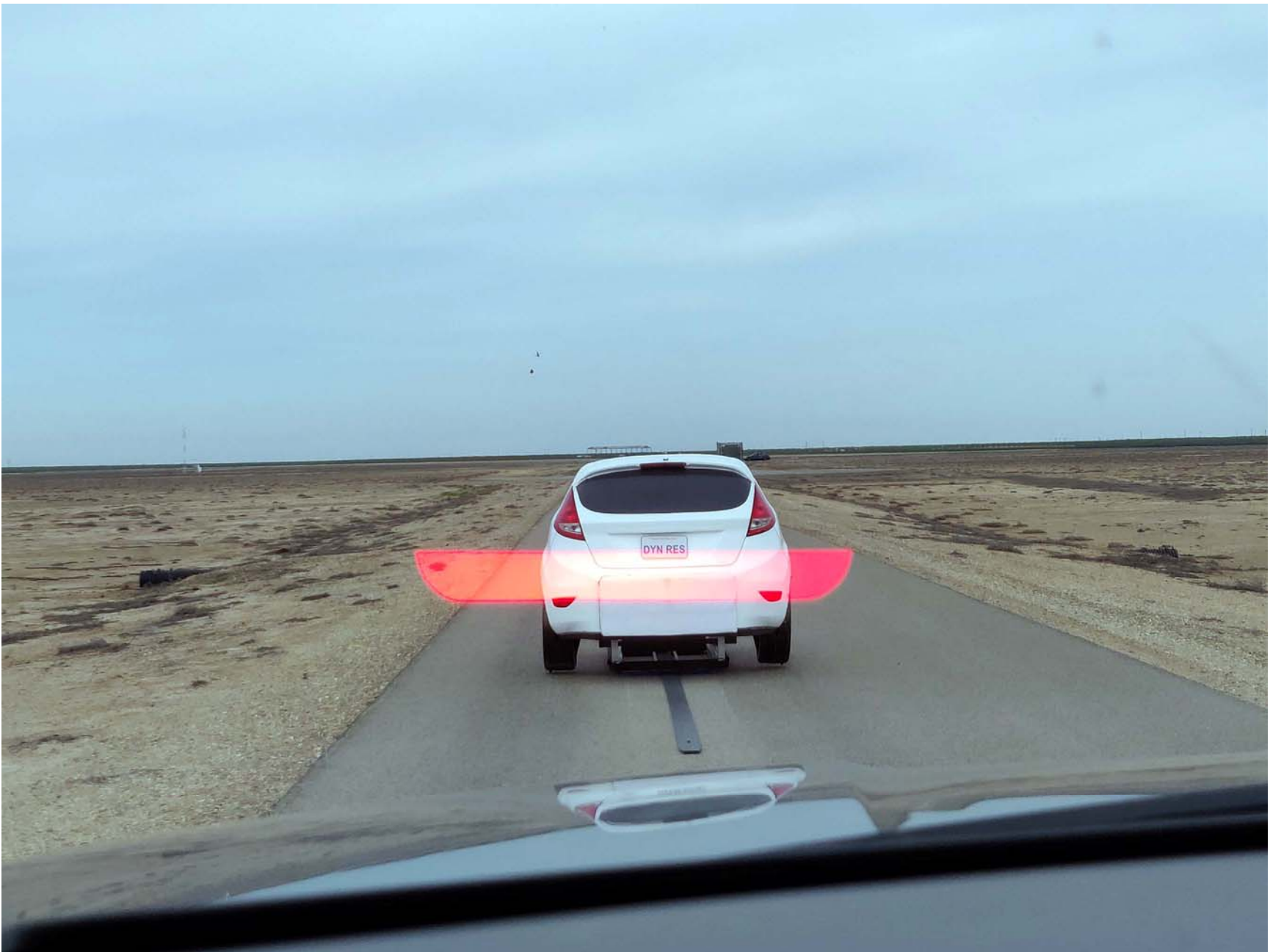
Figure A15. Heads Up AEB Visual Alert
