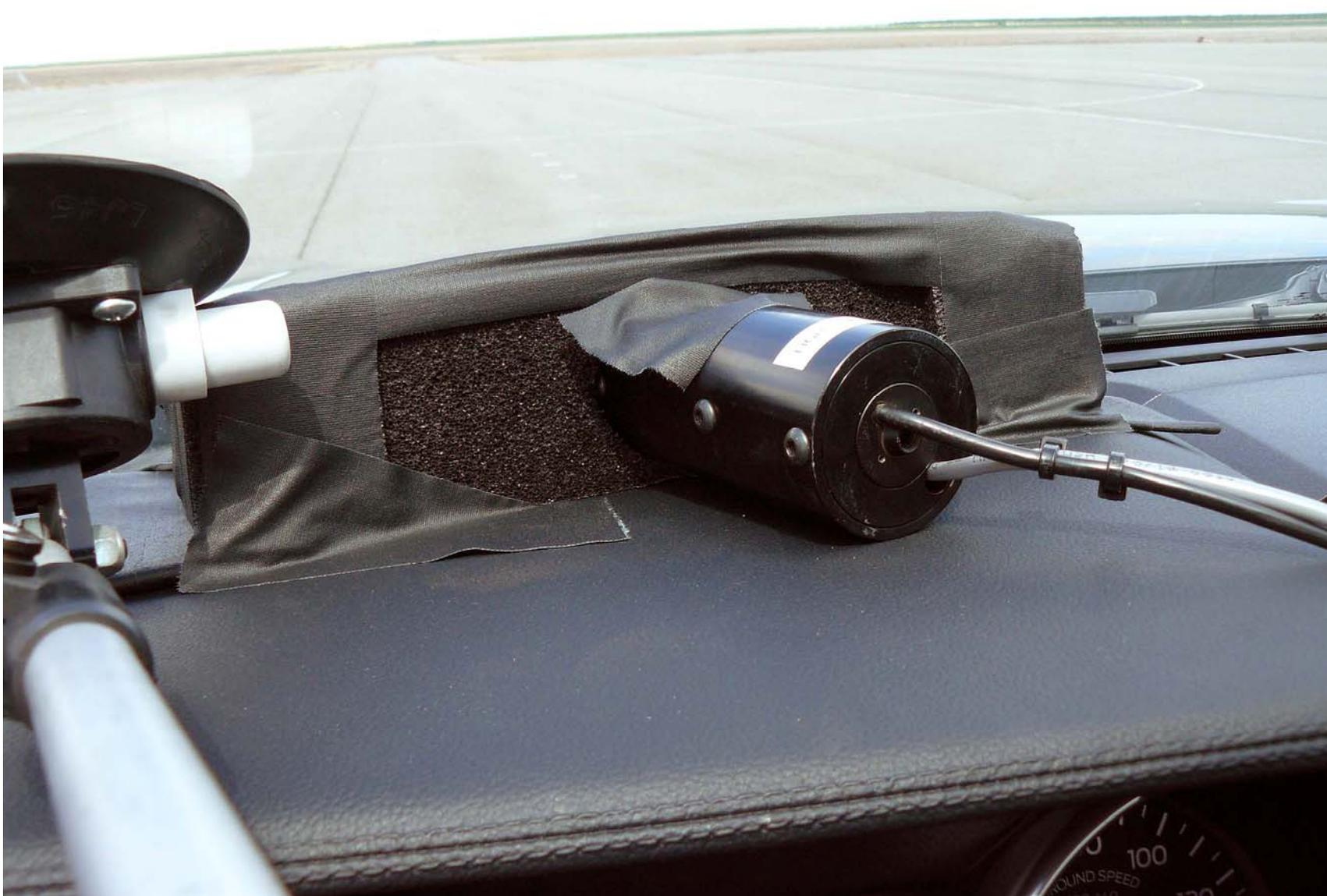
Figure A11. Sensor for Detecting Visual heads Up Alert
