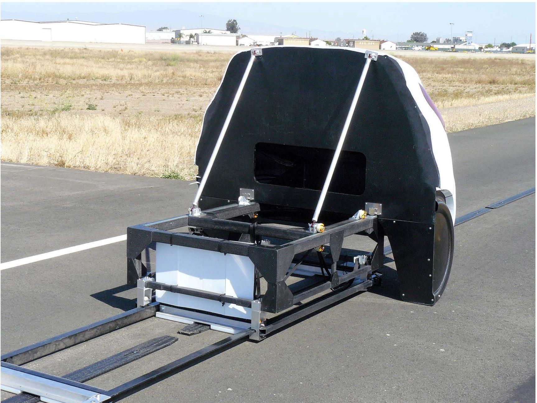
Figure A7. Load Frame/Slider of SSV
