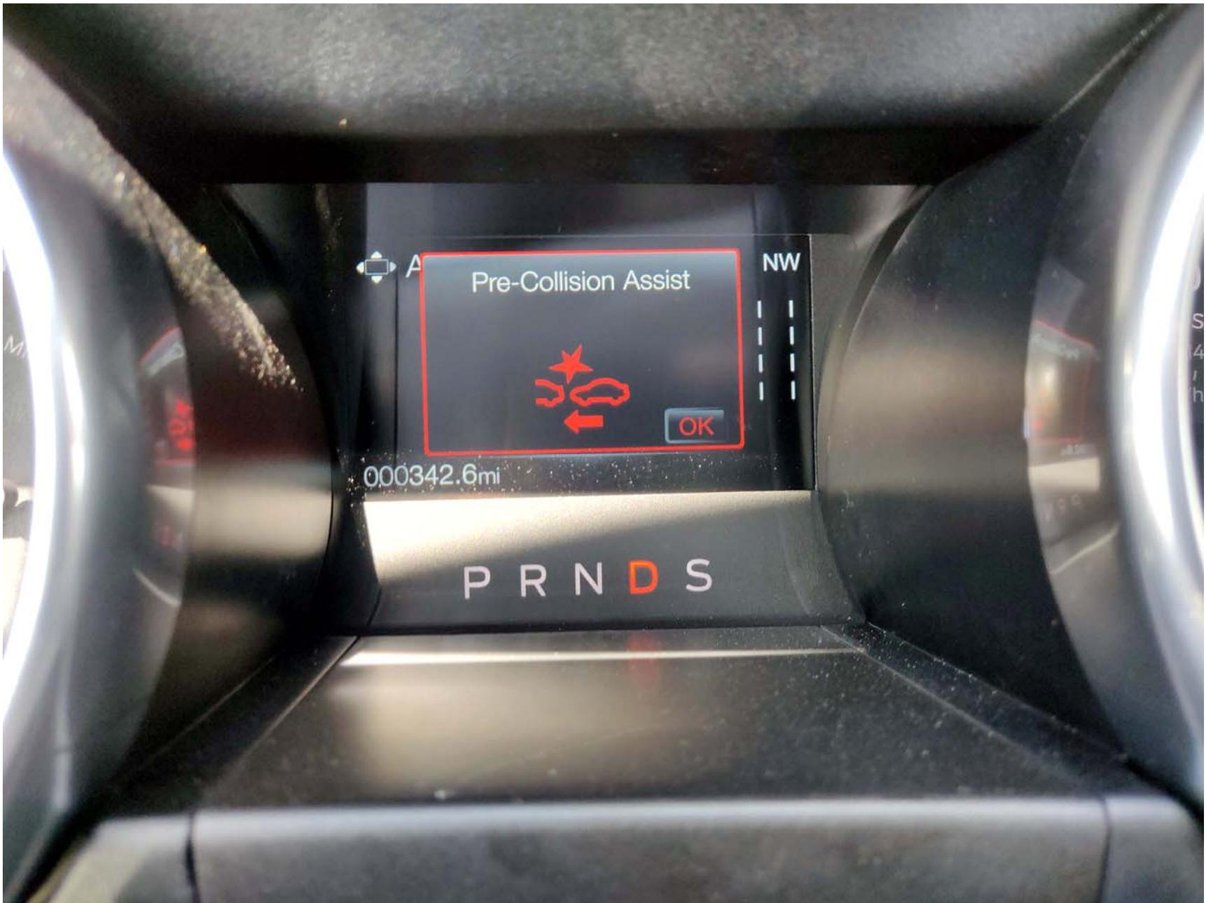
Figure A16. Instrument Panel AEB Visual Alert
