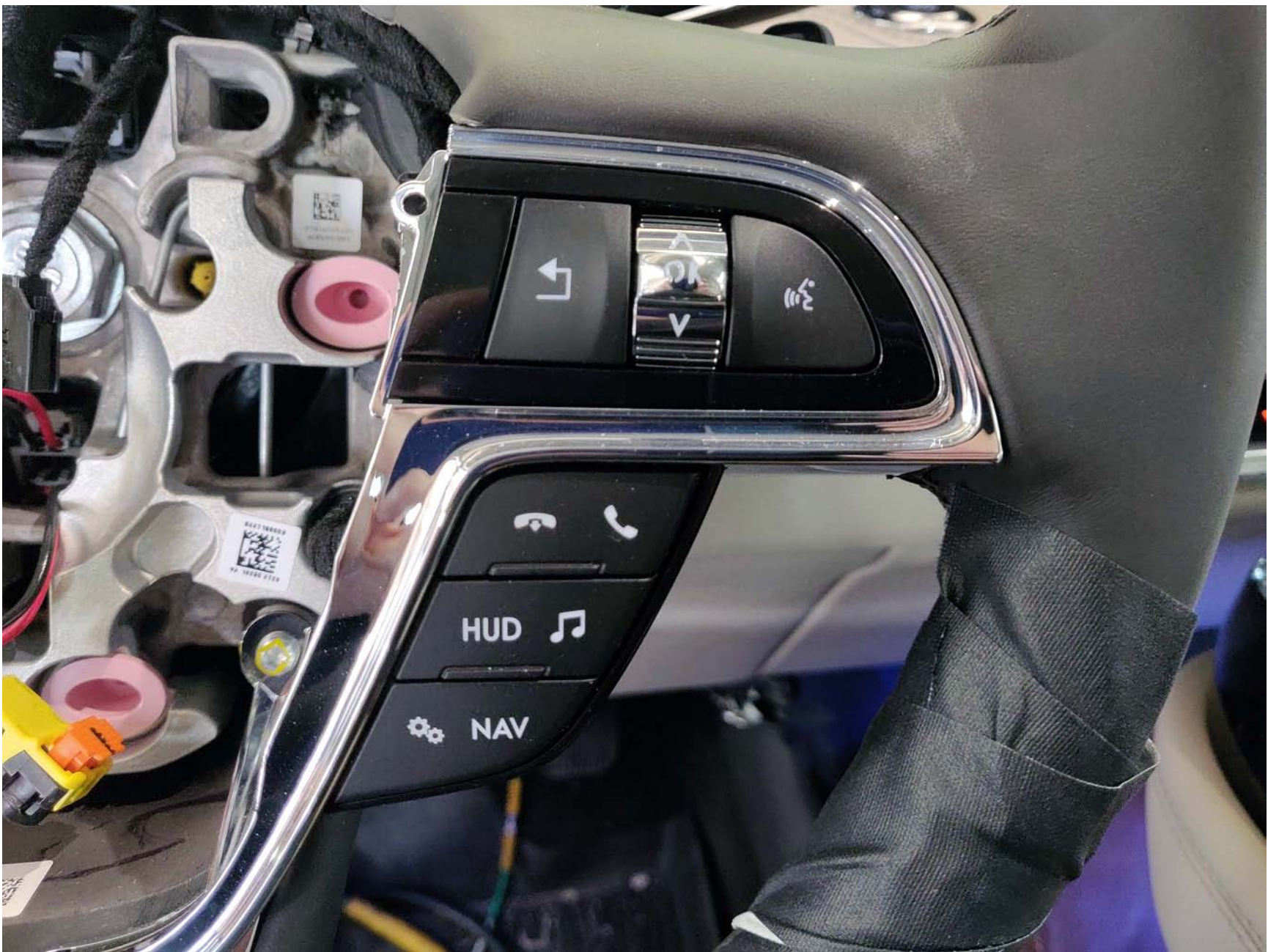
Figure A19. Steering Wheel Mounted Control Buttons for Changing Parameters
