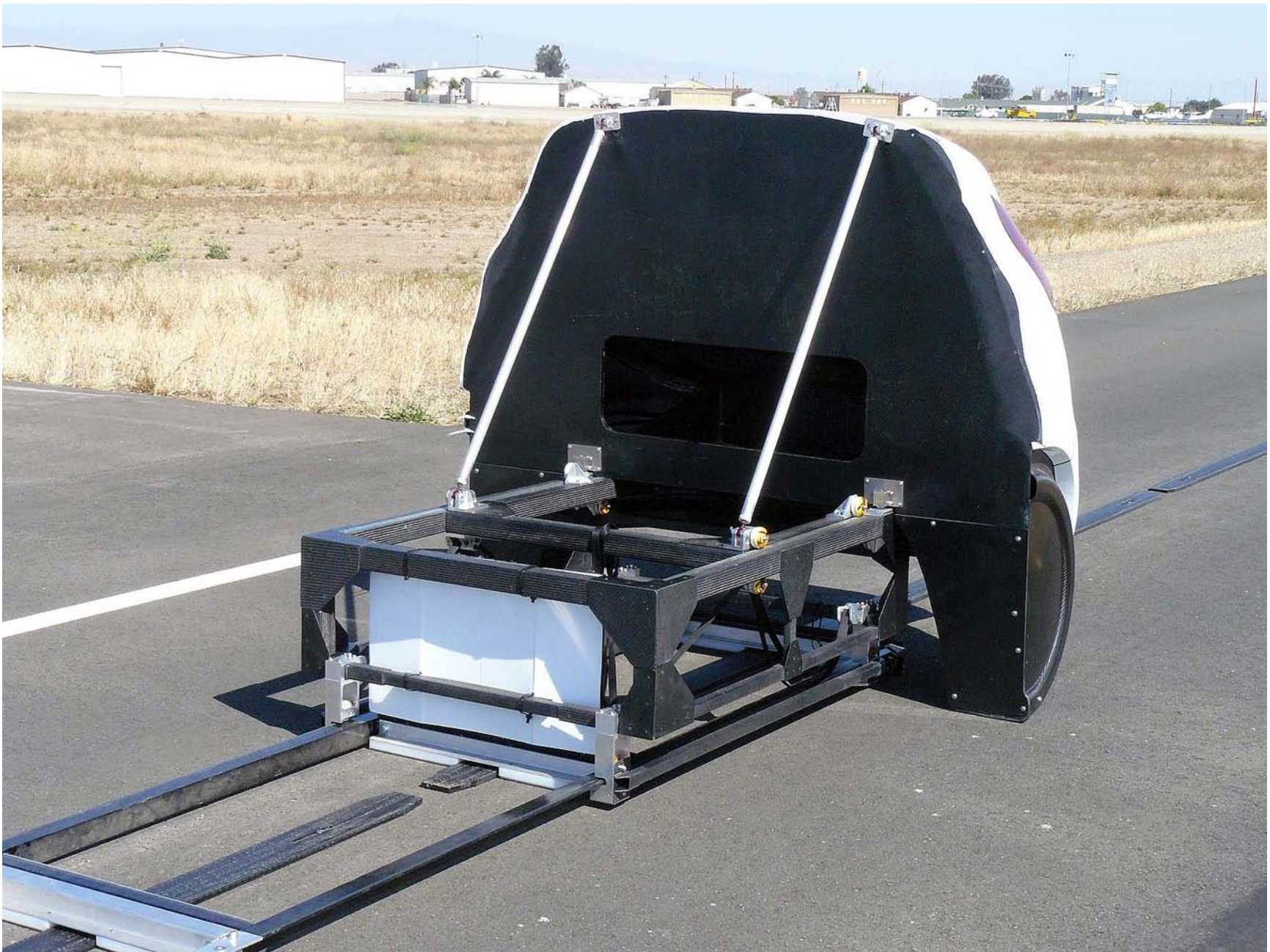
Figure A7. Load Frame/Slider of SSV
