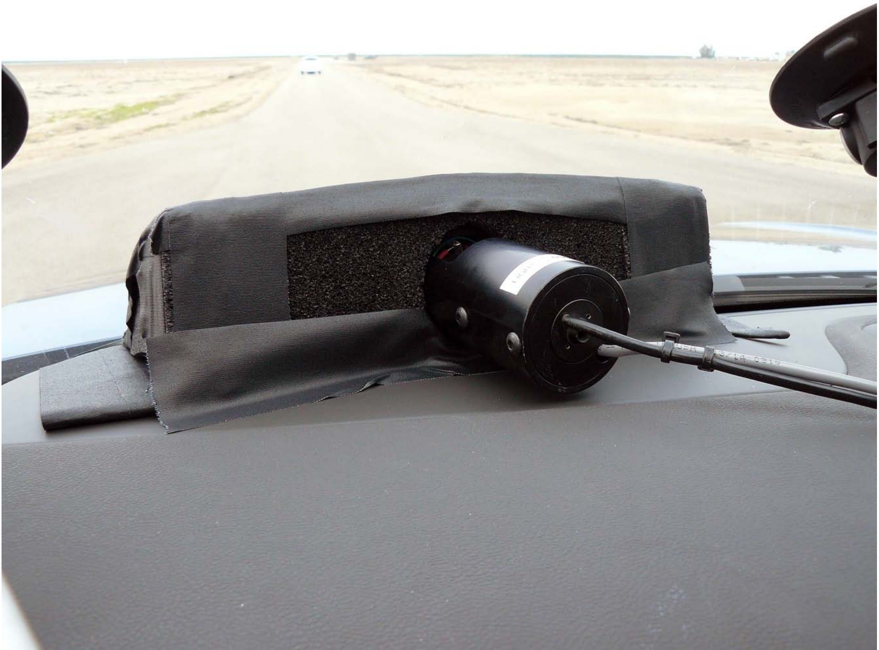
Figure A11. Sensor for Detecting Heads Up Visual Alert
