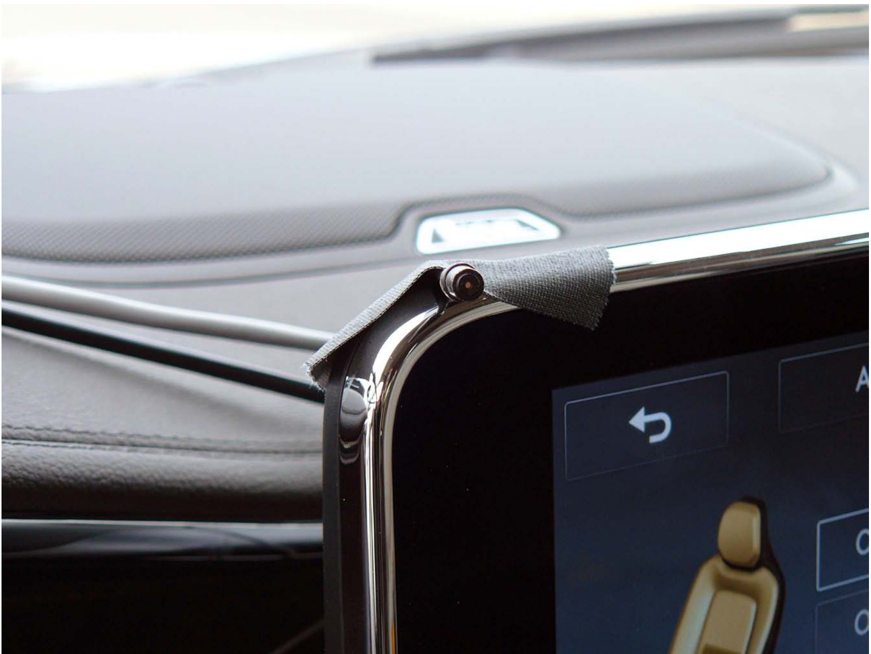
Figure A12. Sensor for Detecting Auditory Alert
