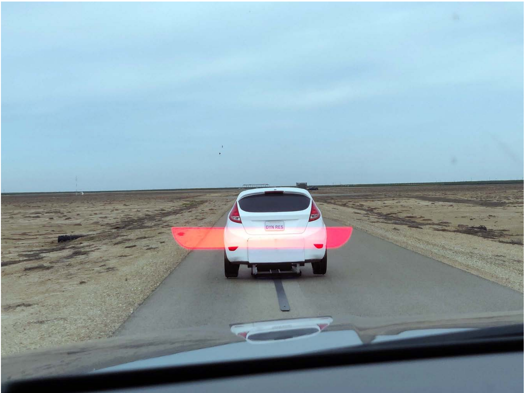
Figure A16. Heads Up Collision Warning Visual Alert
