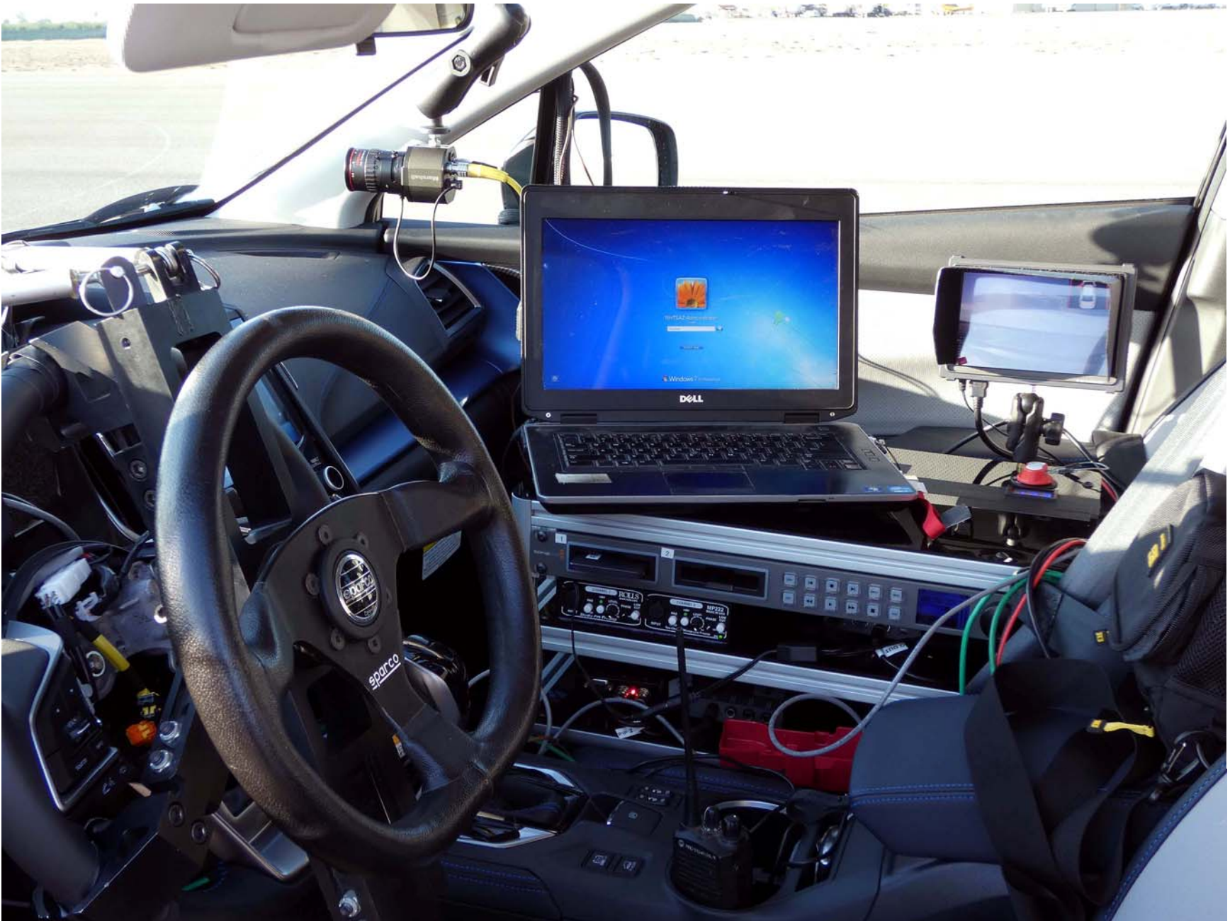
Figure A11. Computer Installed in Subject Vehicle
