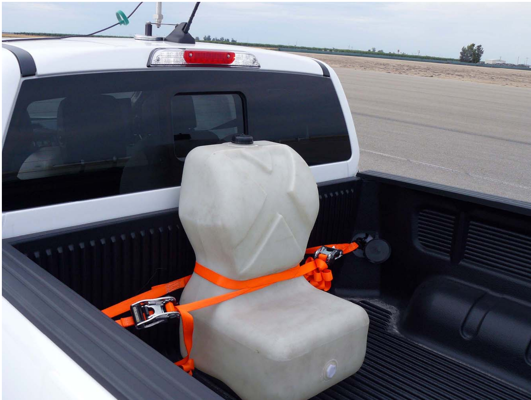
Figure A10. Bed Ballast
