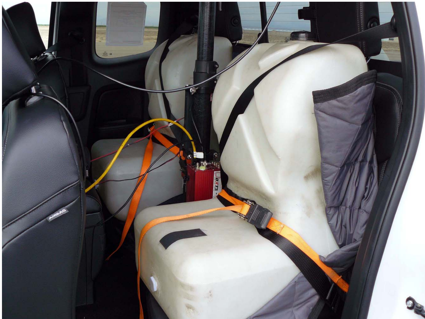
Figure A9. Instrumentation and Rear Seat Ballast in Test Vehicle
