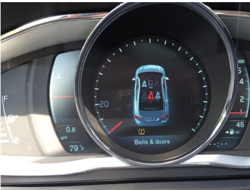
Image 3: Visual Alerts When There is a Change of Status of a Rear Seat Belt on Volvo S60 (MY 2014)
