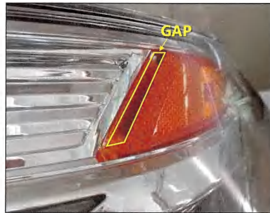
Figure 3. Photo of reflector in worst-case condition
