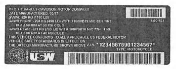
As discussed below, however, tests performed by the respective tire manufacturers demonstrate that these tires have an actual load carrying capacity that exceeds the GAWR at the recommended cold inflation pressure stated on the certification label.
