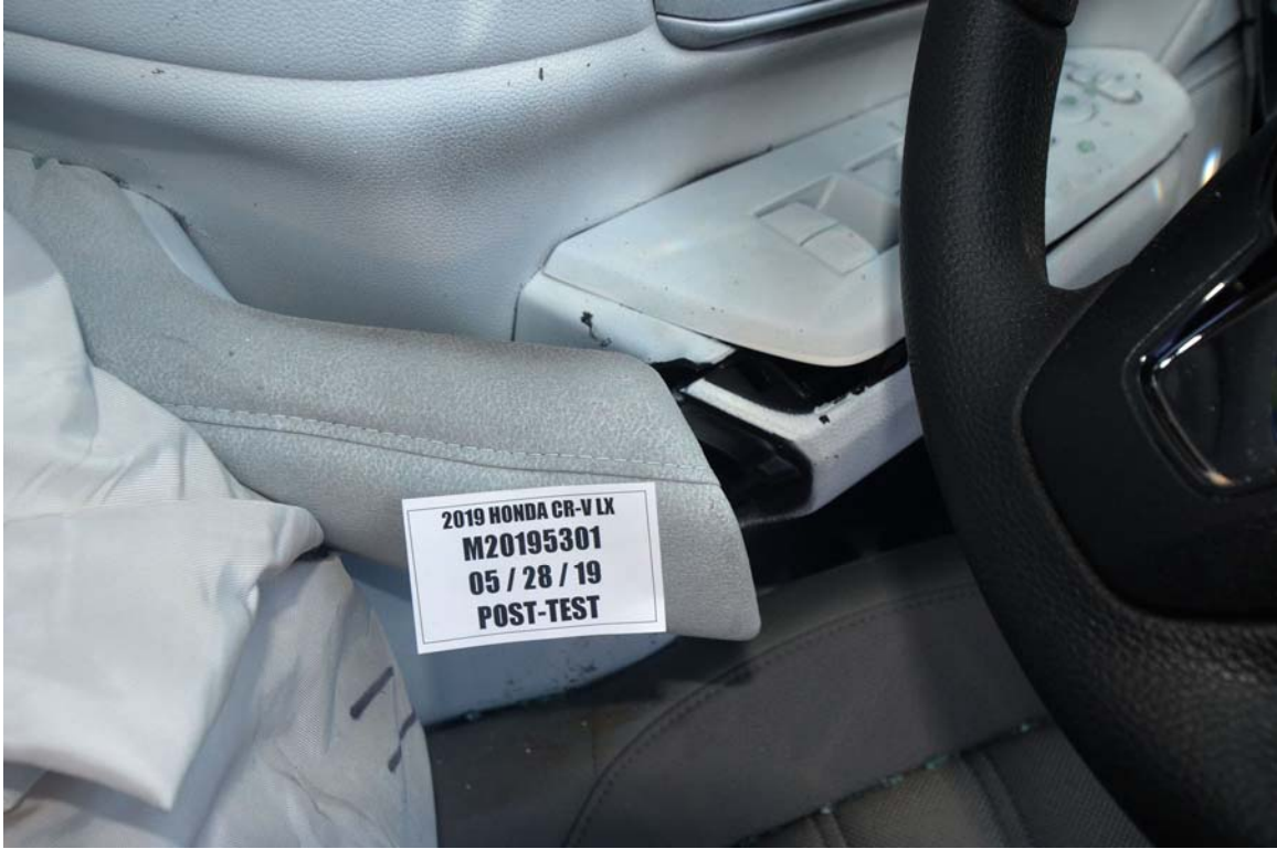
FIGURE 71. Post-Test View of Shattered Vehicle Inner Door Pane
