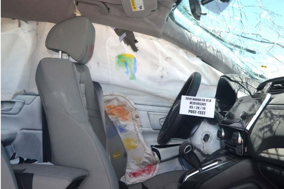
FIGURE 45. Post-Test Inner Door Panel View Showing Dummy Contact Locations
