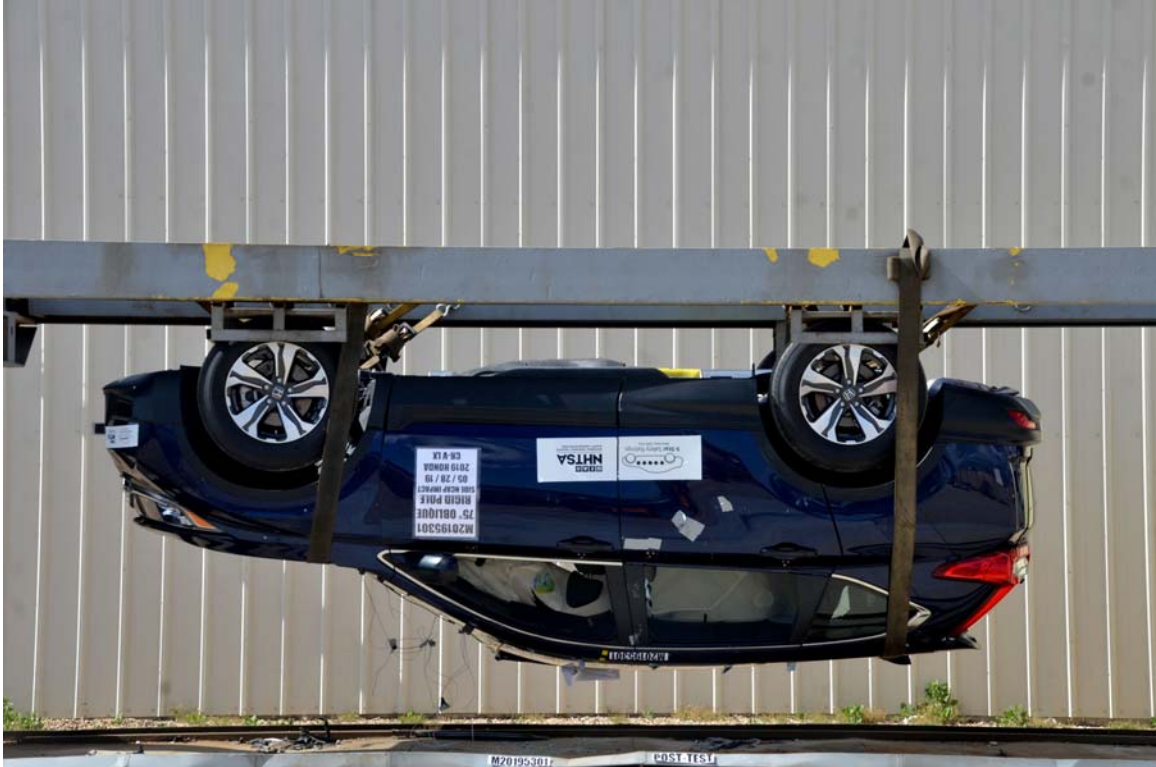
FIGURE 65. FMVSS No. 301 Static Rollover 180 Degrees
