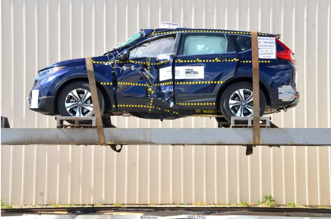
FIGURE 63. FMVSS No. 301 Static Rollover 0 Degrees
