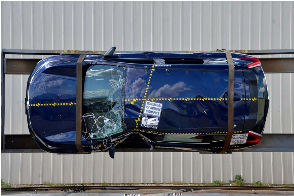
FIGURE 64. FMVSS No. 301 Static Rollover 90 Degrees
