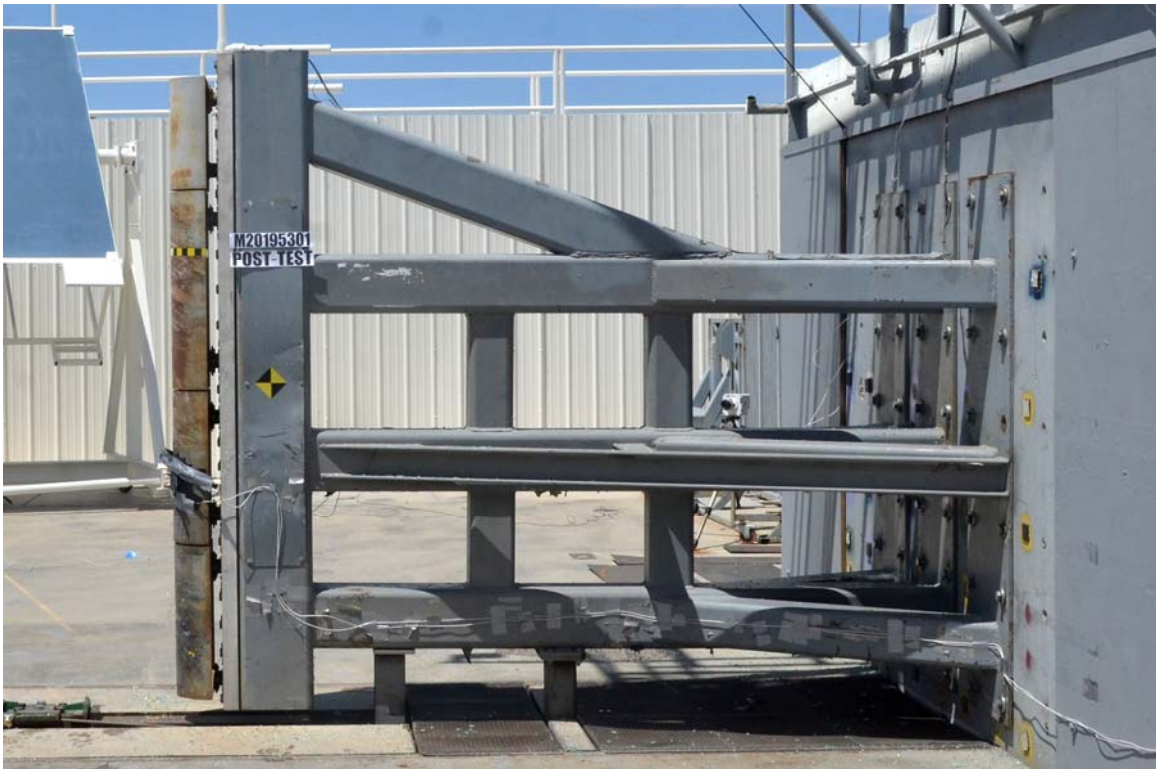
FIGURE 60. Post-Test Pole Barrier Side View
