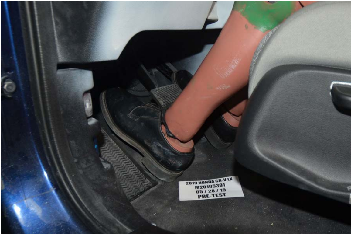
FIGURE 32. Pre-Test Placement of Dummy's Feet
