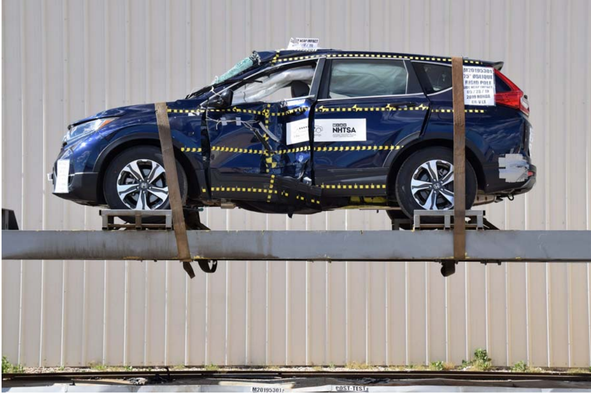
FIGURE 67. FMVSS No. 301 Static Rollover 360 Degrees
