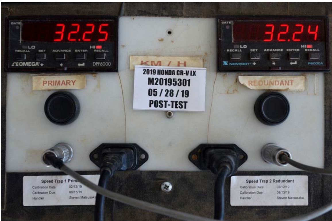
FIGURE 62. Post-Test Primary and Redundant Speed Trap Read-Out
