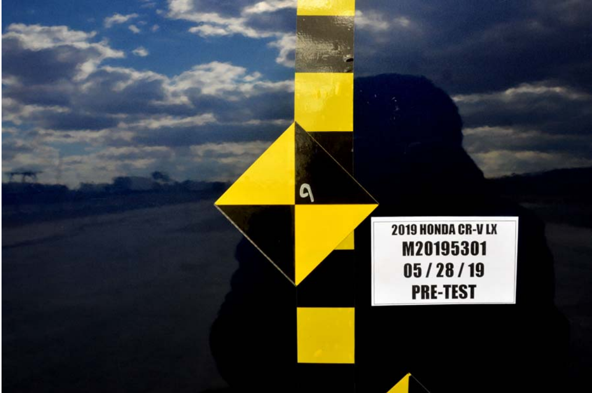
FIGURE 19. Pre-Test Close-Up View of Impact Point Target
