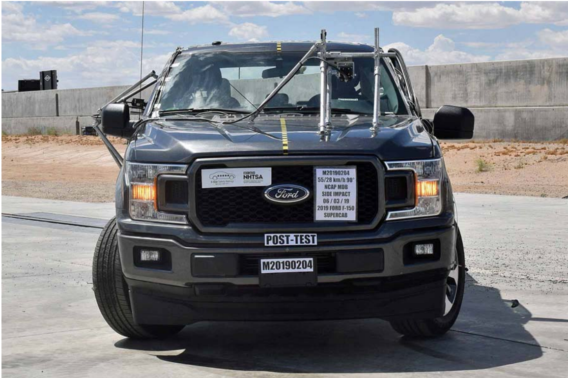
FIGURE 4. Post-Test Frontal View of Test Vehicle
