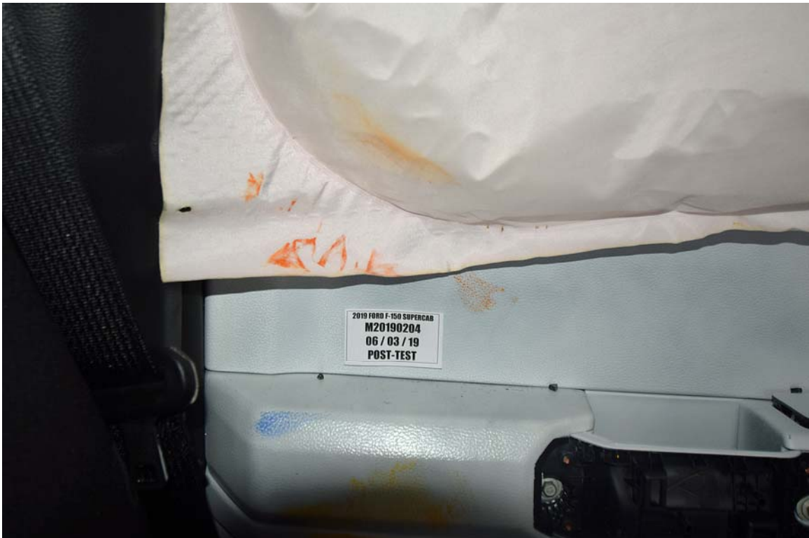
FIGURE 78. Post-Test Rear Passenger Dummy Close-Up Torso Contact with Side Airbag View
