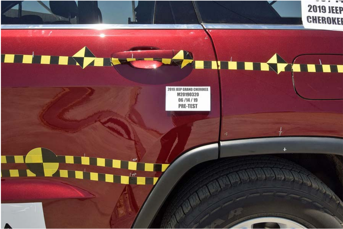
FIGURE 23. Pre-Test Left Rear Door Latch Close-Up
