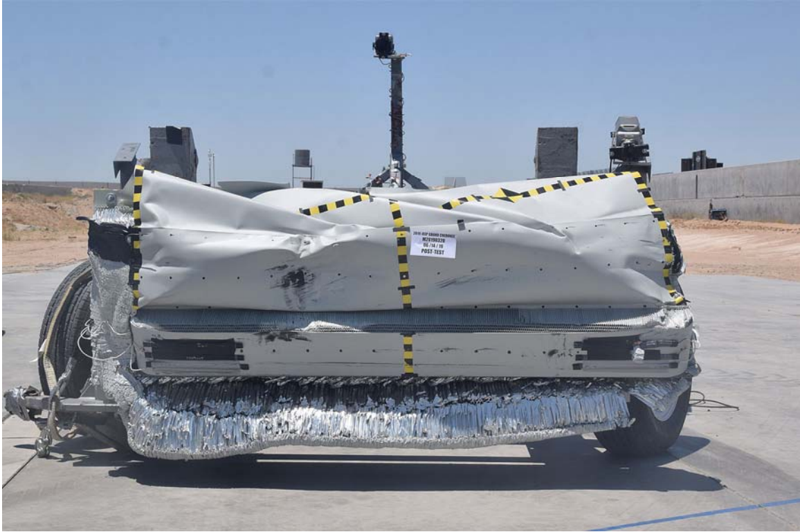
FIGURE 85. Post-Test Front View of MDB Impactor Face
