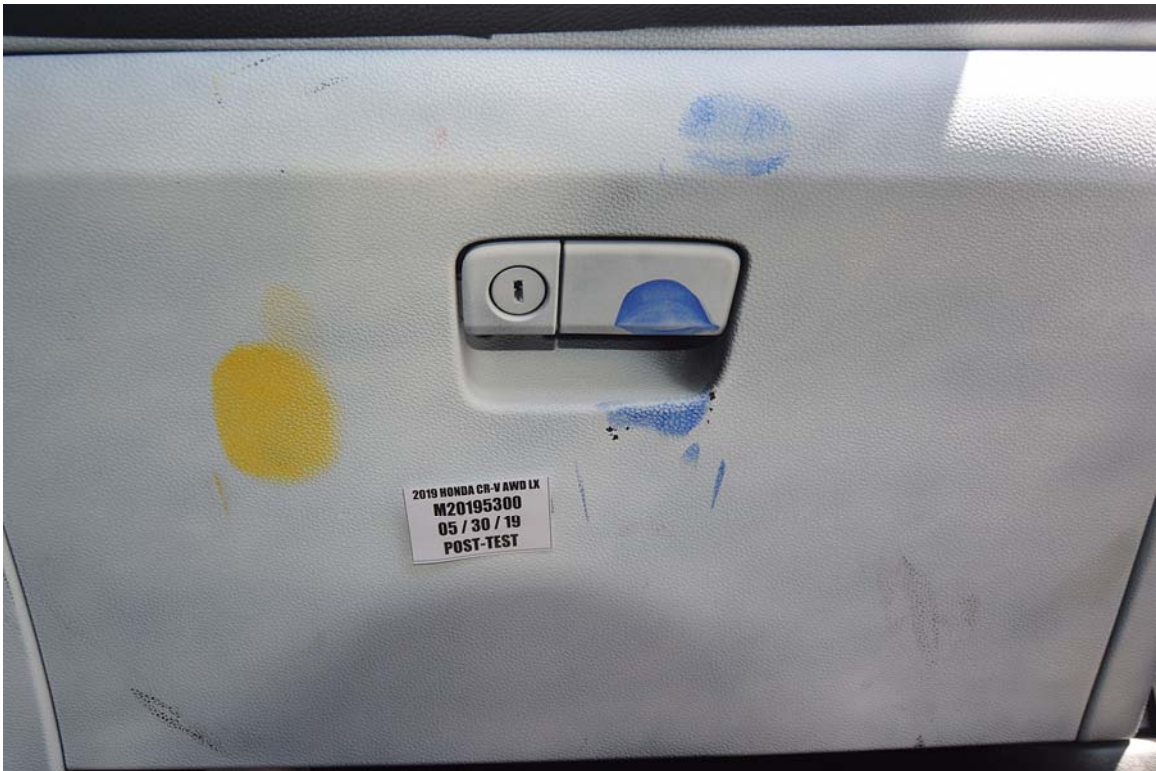
FIGURE 69a. Post-Test Passenger Dummy Contact with Glove Box
