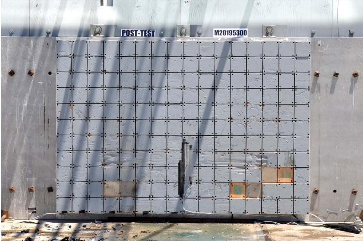
FIGURE 3. Post-Test Load Cell Wall
