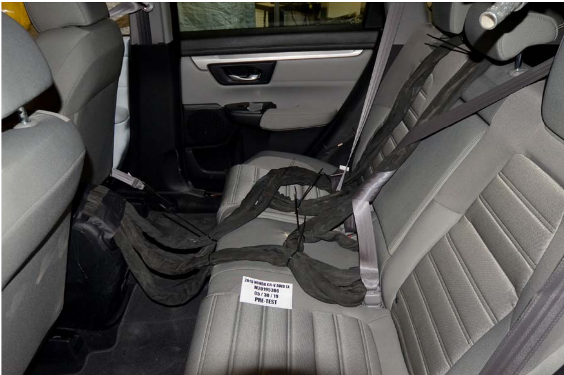
FIGURE 28. Pre-Test Dummy Cable Routing
