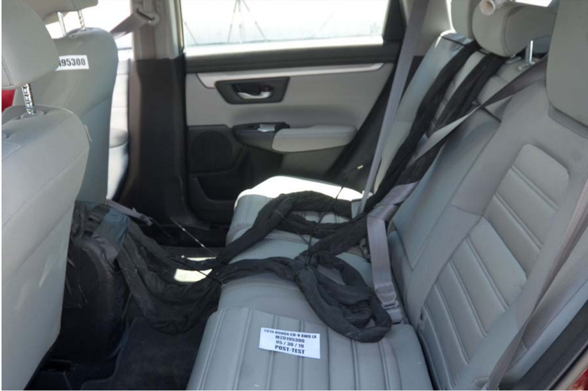
FIGURE 29. Post-Test Dummy Cable Routing
