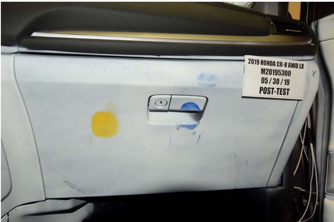
FIGURE 64. Post-Test Passenger's Side Knee Bolster
