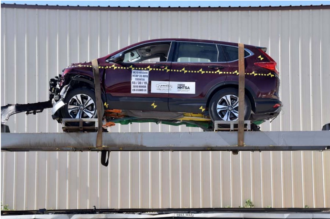
FIGURE 77. Vehicle at 360° on Static Rollover Device
