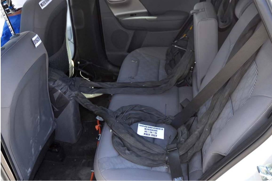
FIGURE 29. Post-Test Dummy Cable Routing
