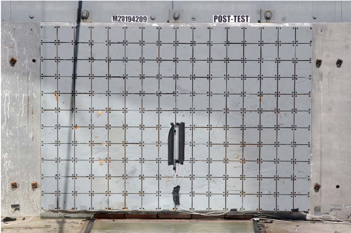
FIGURE 3. Post-Test Load Cell Wall
