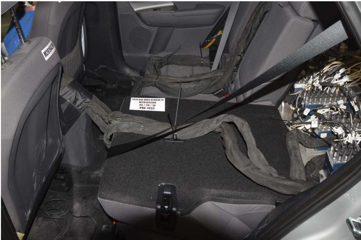
FIGURE 28. Pre-Test Dummy Cable Routing
