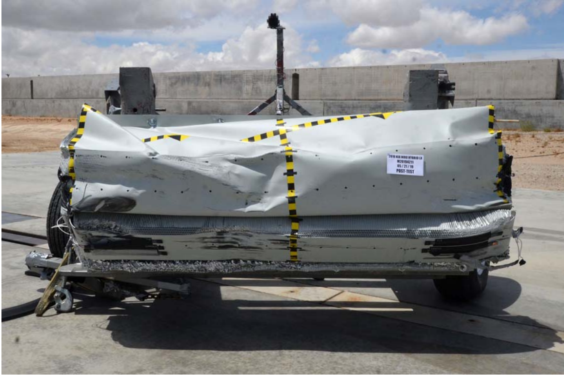
FIGURE 85. Post-Test Front View of MDB Impactor Face
