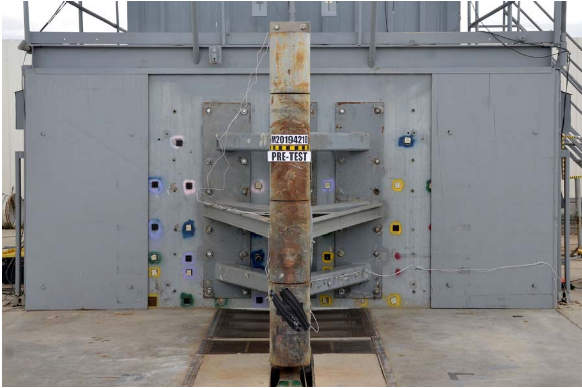
FIGURE 57. Pre-Test Pole Barrier Front View
