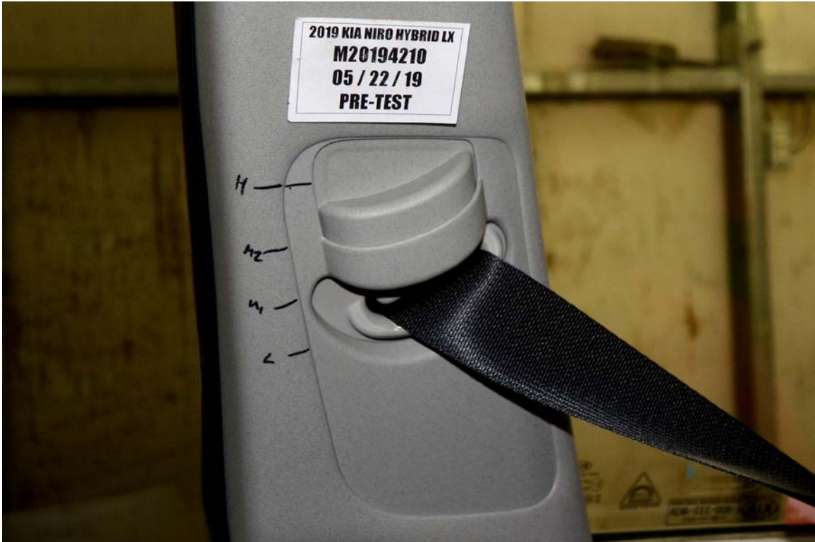
FIGURE 33. Pre-Test View of Belt Anchorage for Dummy
