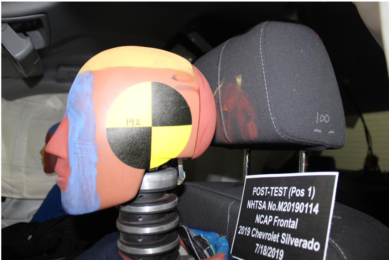
Figure A-48: Post-Test Driver Dummy Contact With Headrest
