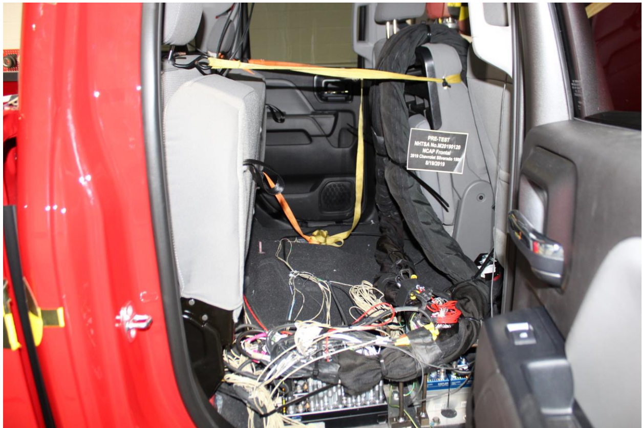
Figure A-28: Pre-Test Dummy Cable Routing
