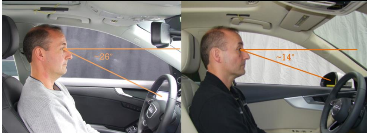
Figure 28. Downward Viewing Angle, CMS Display Versus Mirror
