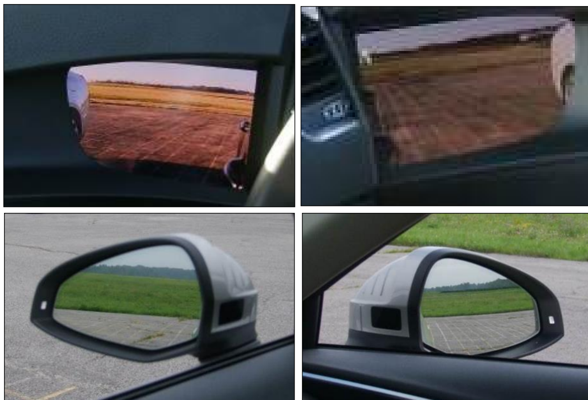
Figure 43. Sedan Positioned 5 Feet (1.52 m) Aft of Front Bumper, as Viewed With Side CMS (top) and Mirrors (bottom) on Driver (left) and Passenger Side (right)
