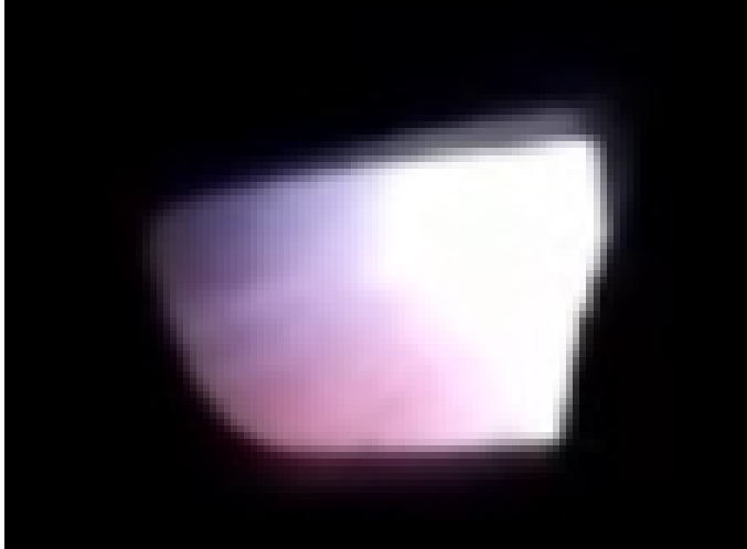
Figure 37. Driver-Side CMS Display, Blooming and Lens Flare
