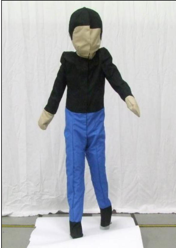
Figure 10. Posable Child Mannequin Test Object, Front View
