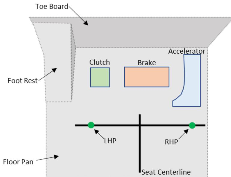
8.1 Using the diagram below, locate the Pedal Reference Point (PRP) and the Right Heel Point (RHP) using a measurement device such as a tape measure, CMM, 200 mm bar, and/or calipers. Use the active part of the pedal, which is defined as the moveable part of the floor-mounted pedal.
