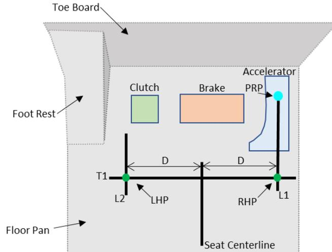
8.5.1 Measure and mark a point on the floor pan to the left of the seat centerline (looking toward the front of the vehicle) that is the same distance (D) from the seat centerline as RHP and is in the same vehicle lateral, vertical (YZ) plane. This is the left heel point (LHP).
