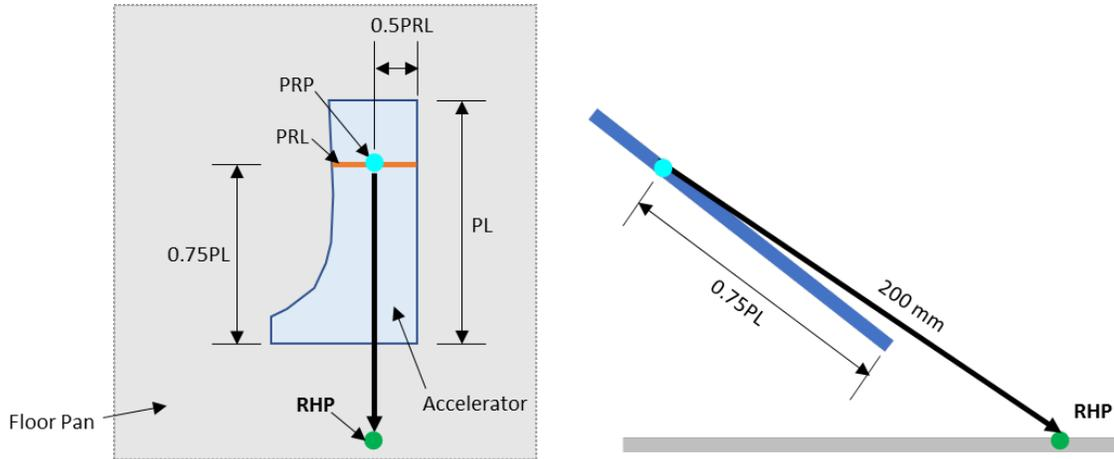
8.1.1 Determine the overall pedal length (PL) on the active pedal, as measured along the surface of the moveable pedal from the top most edge/point to the bottom most edge/point. Record the length: \_\_\_\_\_. Calculate 75% of this length (0.75PL). Establish the pedal reference line (PRL) by marking a line in the y-direction on the pedal surface at 0.75PL from the bottom edge of the pedal.
