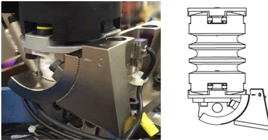
**Figure 6: WSID-50M Head/Neck Adjustment**
