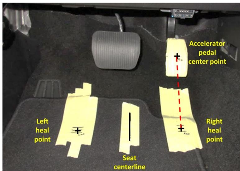
**Figure 5: Foot Placement Diagram**
