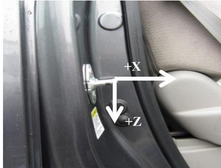
11.27 Create a Seat Tracking Point (STP): Place a target point 20 mm forward of the H-point machine H-point on a rigid part of the seat and record its location in the table below. This reference point will be used to locate the dummy H-point relative to the seat if the seat cannot be set to the mid-track position.
