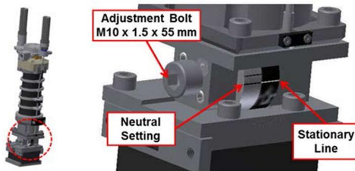
**Figure 7: THOR-50M Neck Setup for Use in Crash Testing**
