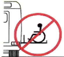
FIGURE 2-2: RICON RECOMMENDS PASSENGERS FACE OUTBOARD WHEN RIDING LIFT PLATFORM
