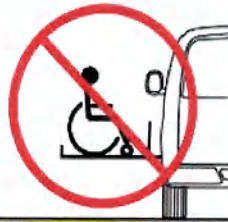
FIGURE 2-2: ALWAYS FACE OUTBOARD WHEN RIDING ON THE LIFT PLATFORM
