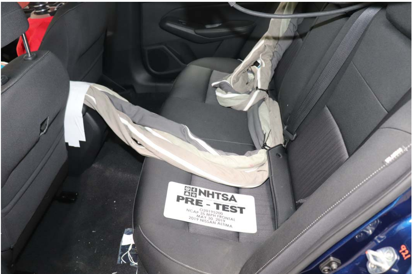
Photo No. 028 - Pre-Test Dummy Cable Routing
