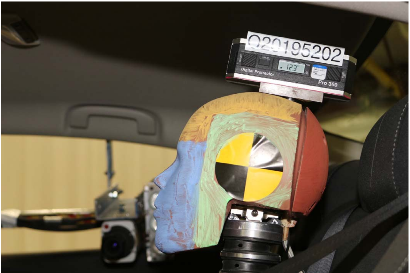
Photo No. 063 - Pre-Test View of Rear Passenger Dummy Head Showing Dummy Head is Level
