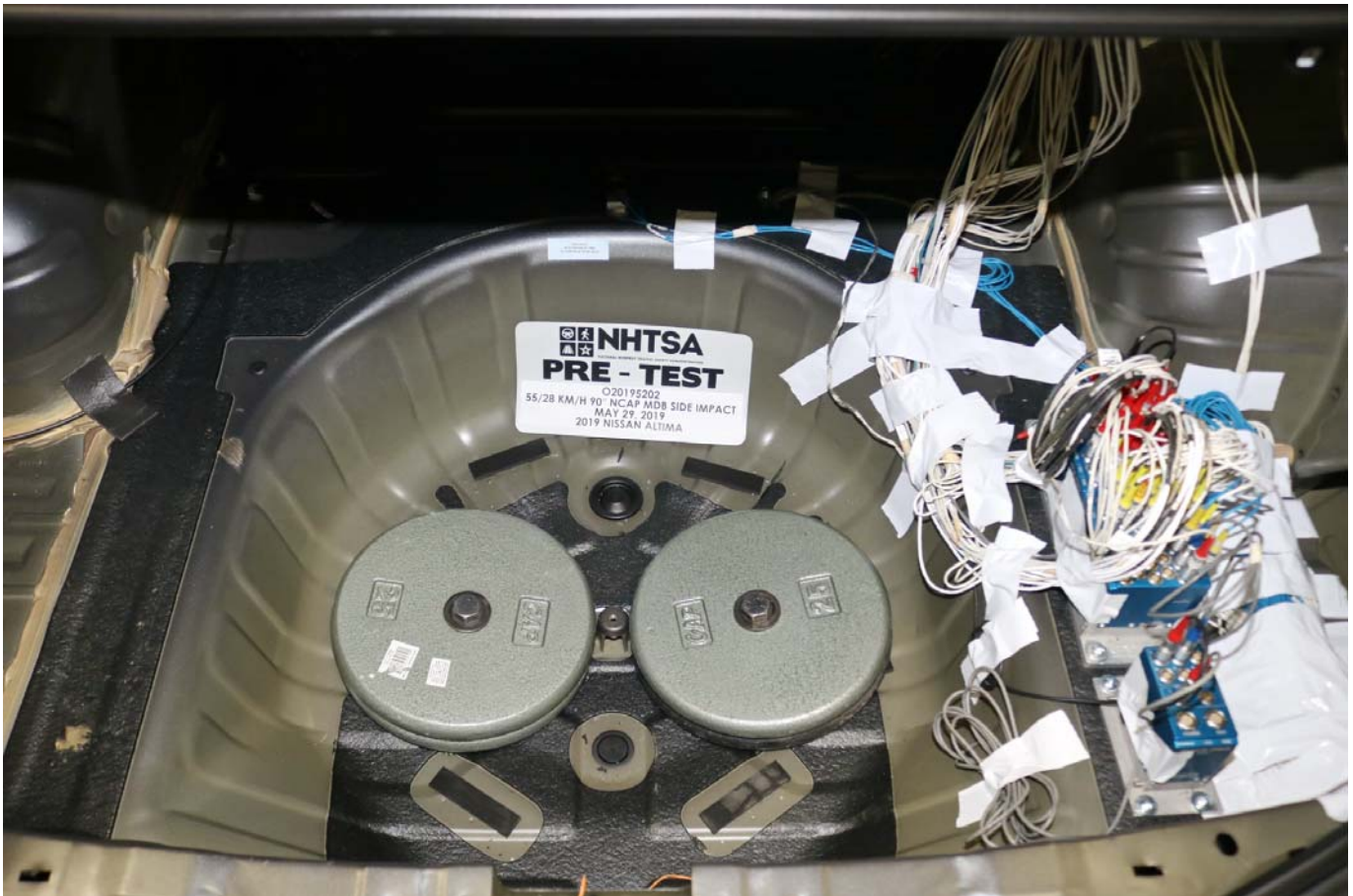
Photo No. 094 - Pre-Test Ballast View
