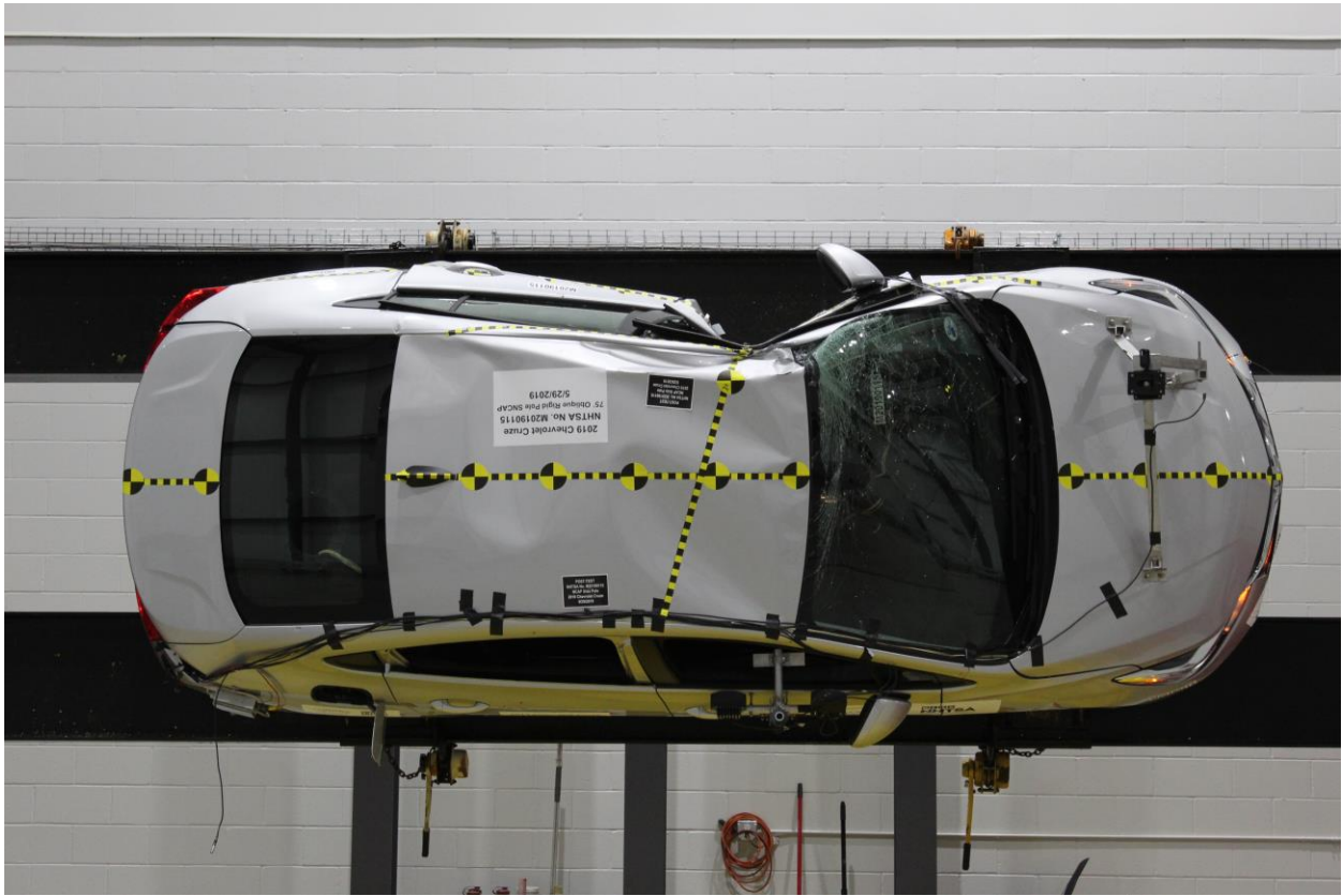
Figure A-64: FMVSS No. 301 Static Rollover 90 Degrees
