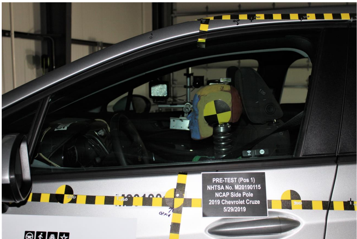
Figure A-24: Pre-Test Left Side View of Dummy Shoulder and Door Top View
