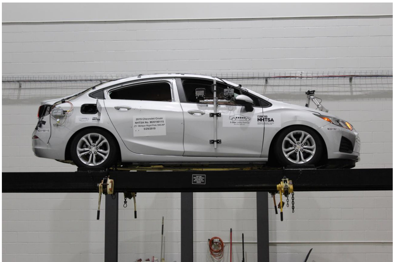
Figure A-63: FMVSS No. 301 Static Rollover 0 Degrees
