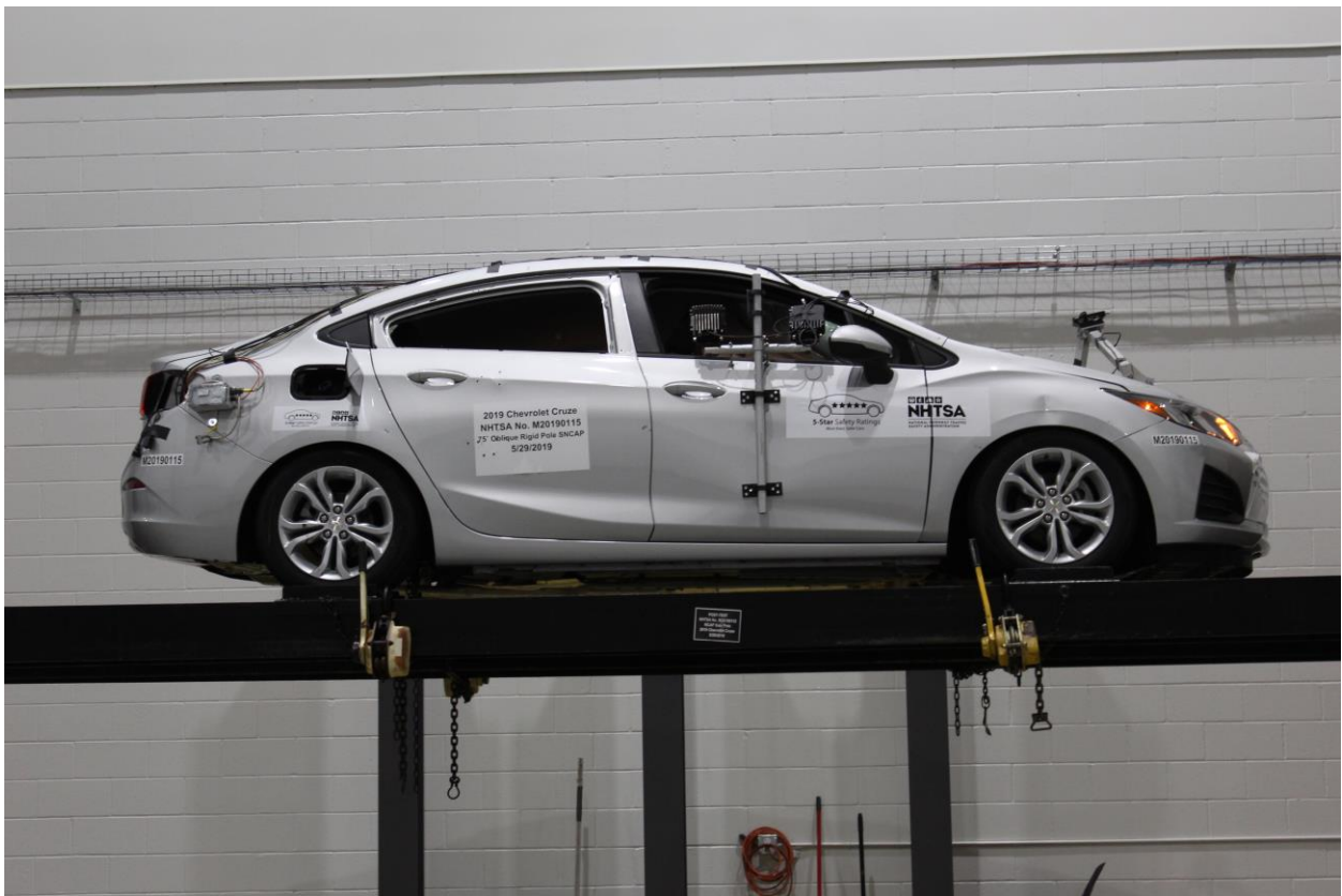
Figure A-67: FMVSS No. 301 Static Rollover 360 Degrees
