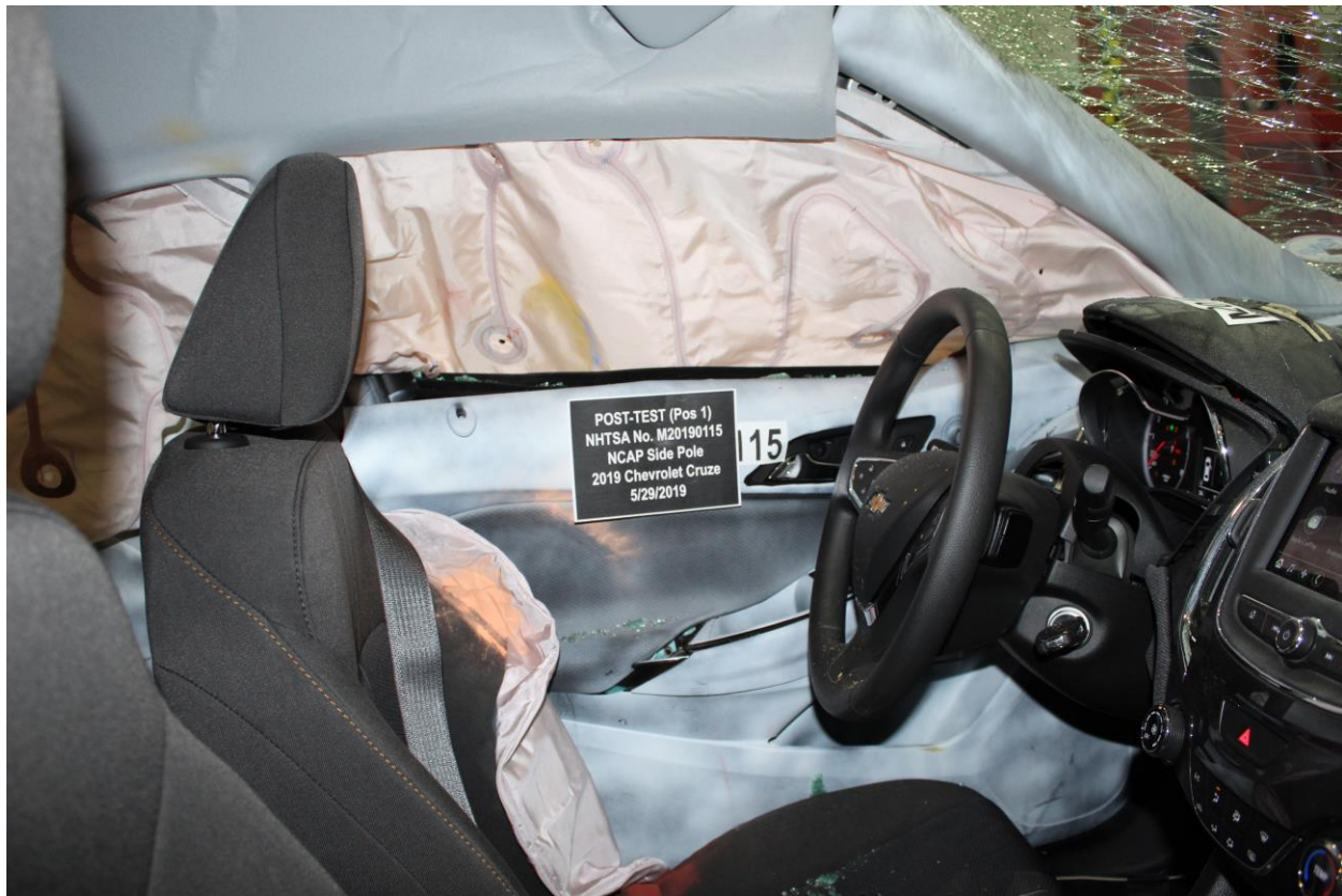
Figure A-71: Post-Test View of Shattered Vehicle Inner Door Panel (if applicable)
