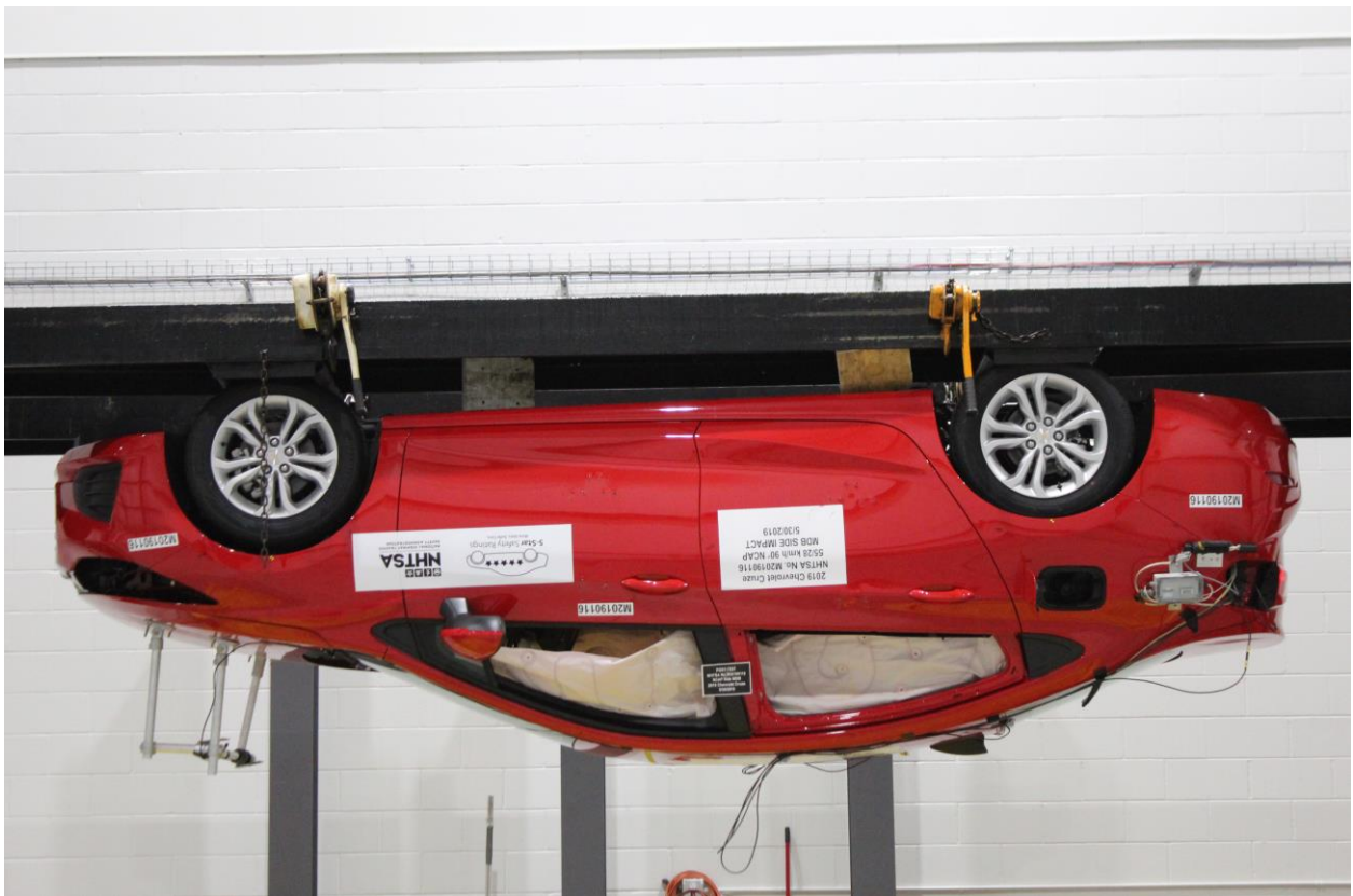
Figure A-98: FMVSS No. 301 Static Rollover 180 Degrees
