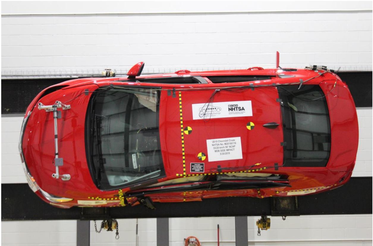
Figure A-99: FMVSS No. 301 Static Rollover 270 Degrees
