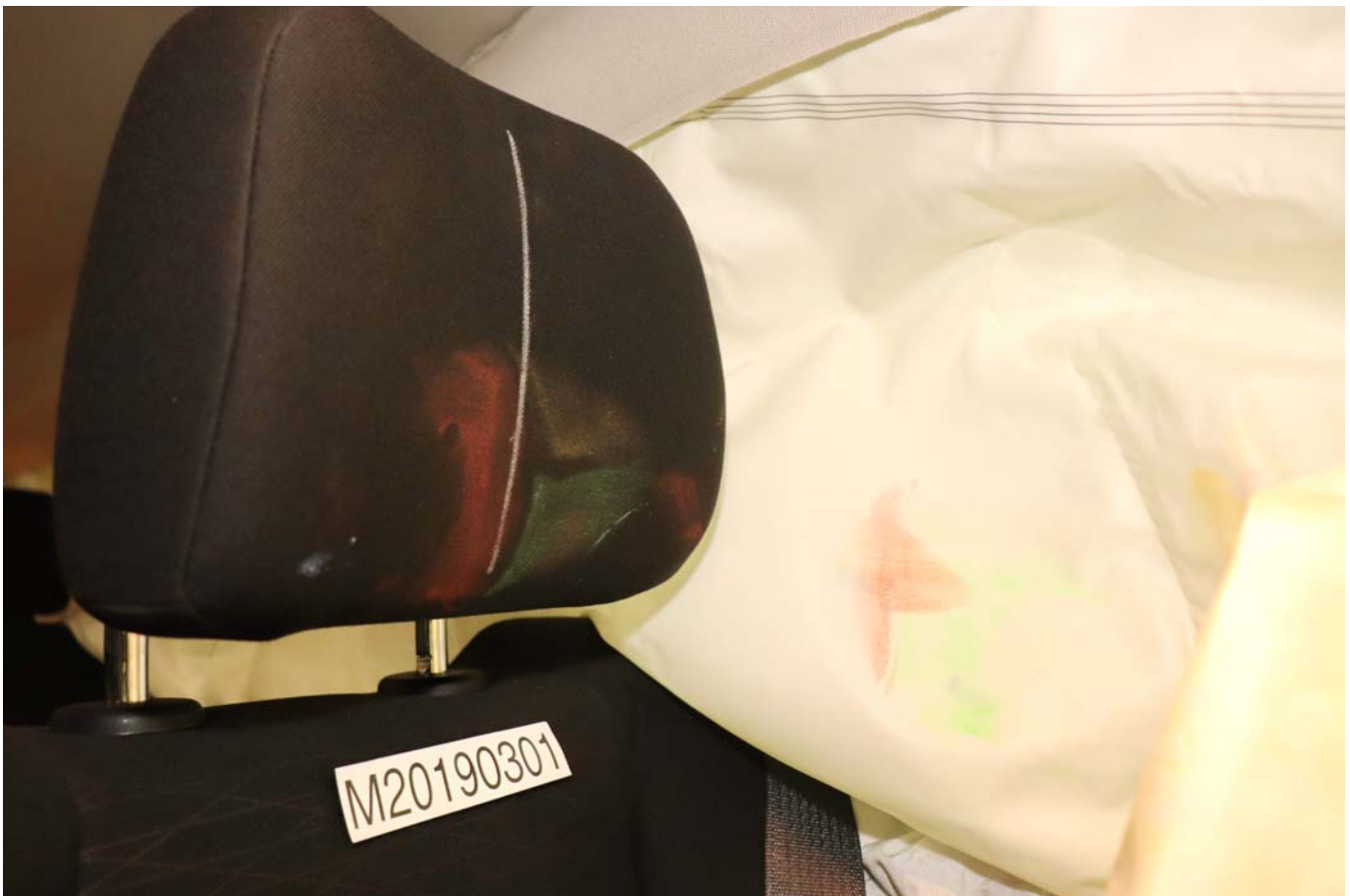
Photo No. 046 - Post-Test Dummy Close-Up Head Contact with Vehicle Interior View
