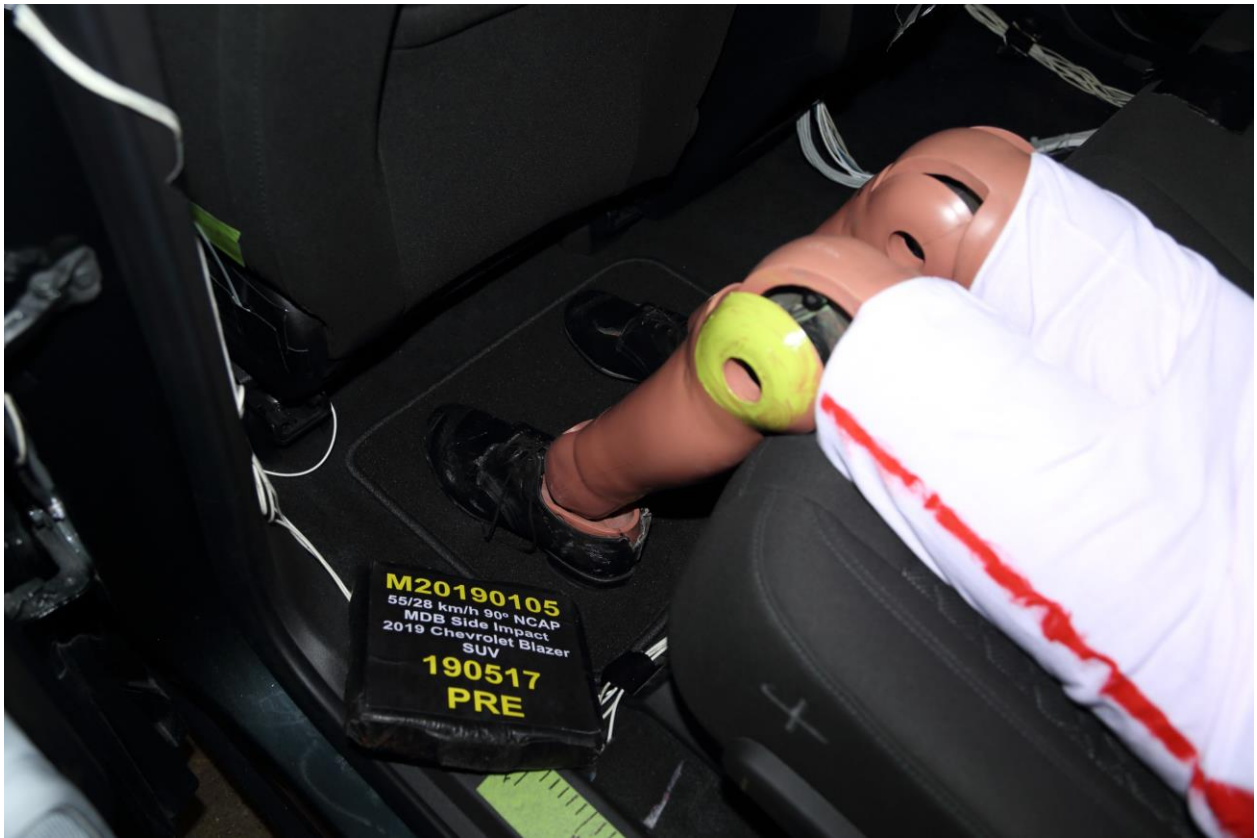
064 Pre-Test Placement of Rear Passenger Dummy's Feet
