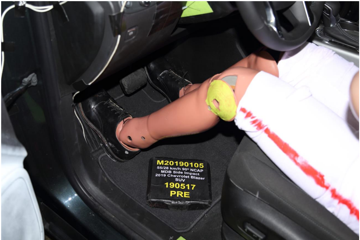
034 Pre-Test Placement of Driver's Dummy Feet
