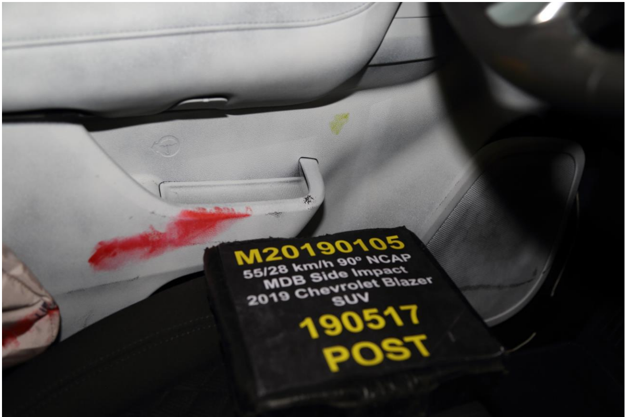
054 Post-Test Driver Dummy Close-Up Knee Contact View
