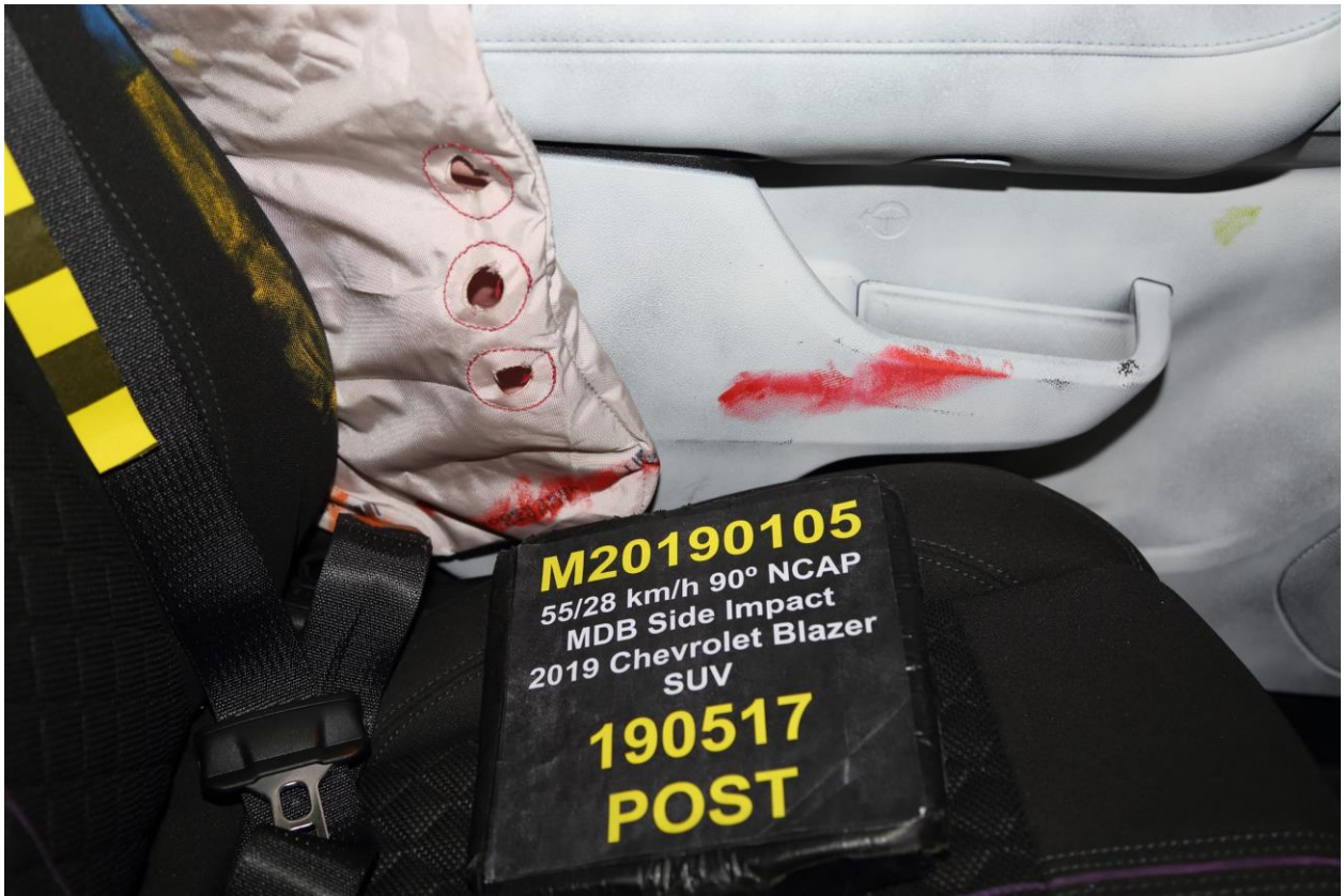
052 Post-Test Driver Dummy Close-Up Pelvis Contact View
