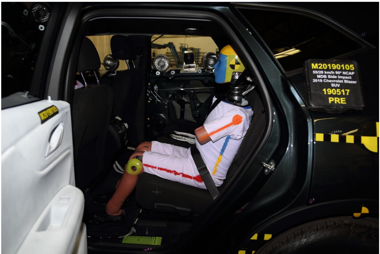
055 Pre-Test Left Side View of Passenger Dummy Showing Belt and Chalking
