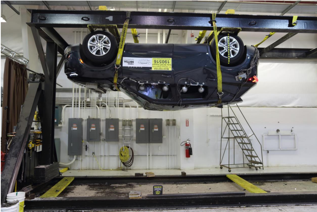
No. 065 FMVSS No. 301 Static Rollover 180 Degrees
