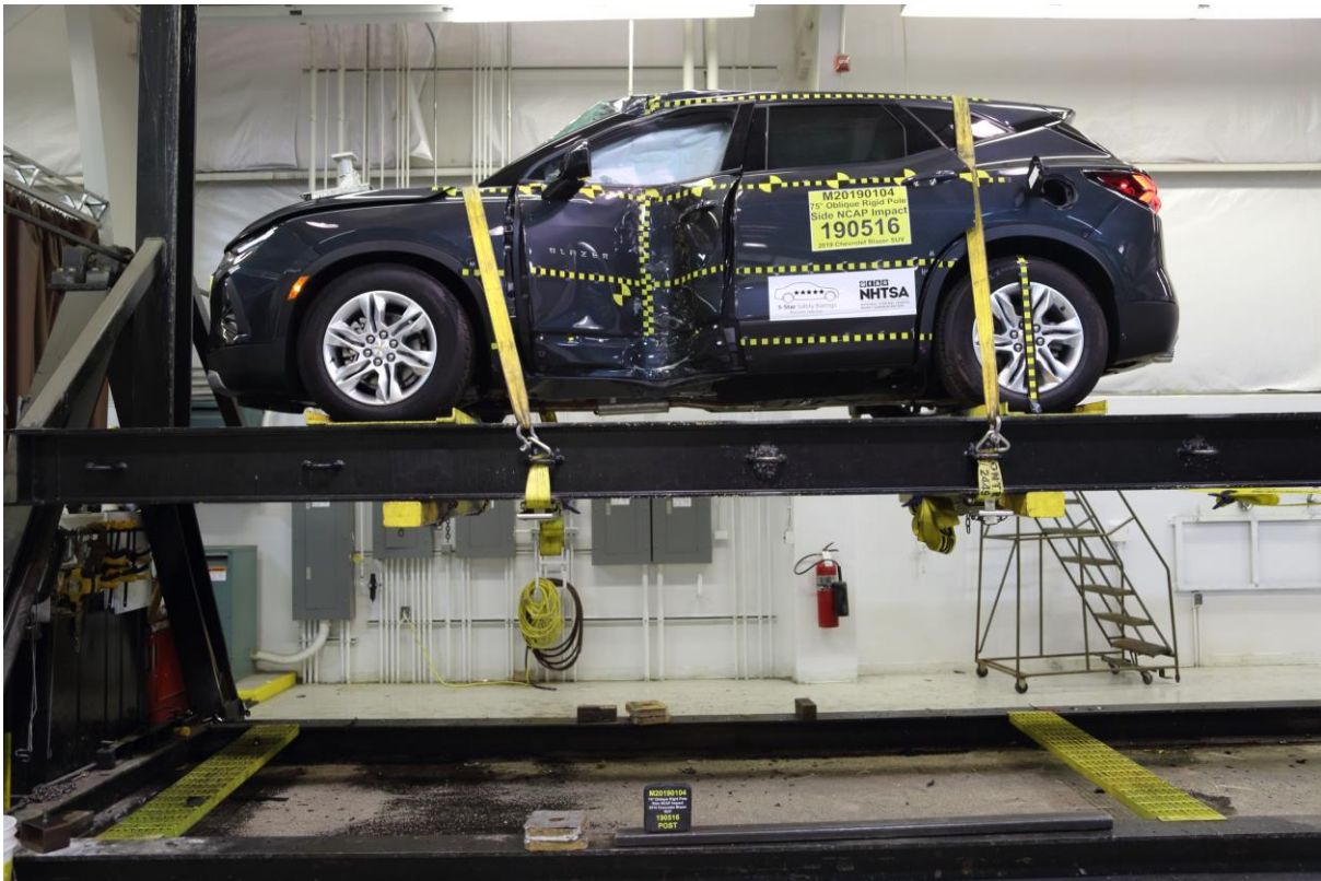
No. 063 FMVSS No. 301 Static Rollover 0 Degrees
