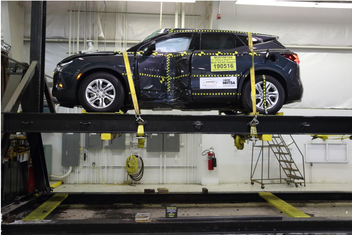
No. 067 FMVSS No. 301 Static Rollover 360 Degrees
