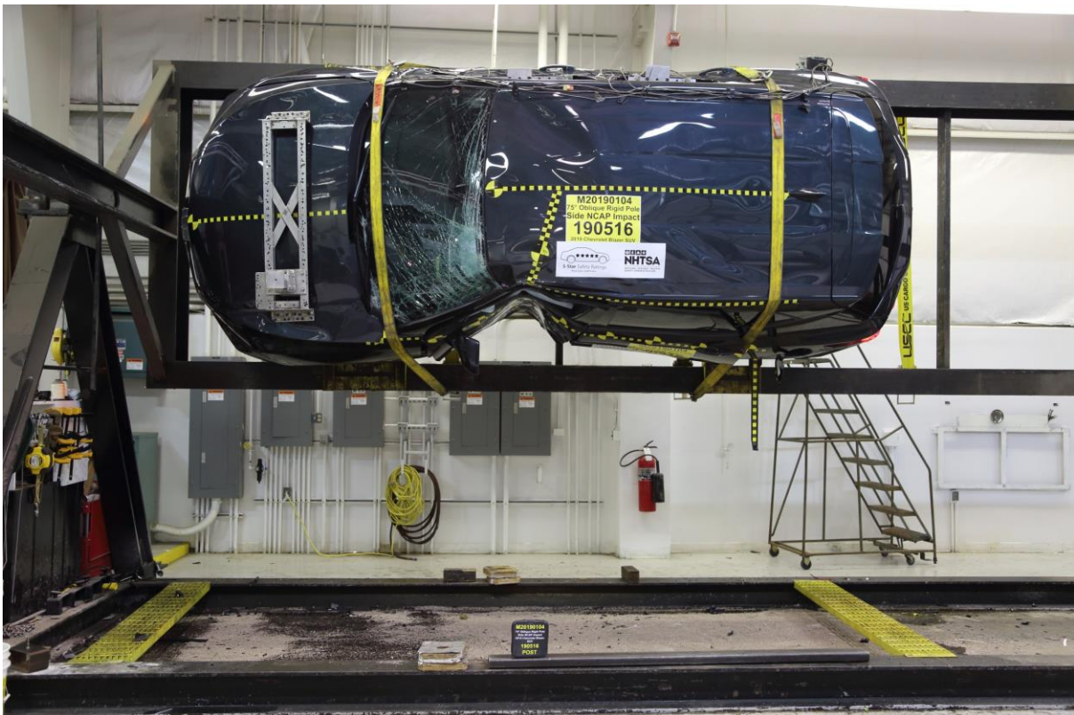
No. 064 FMVSS No. 301 Static Rollover 90 Degrees
