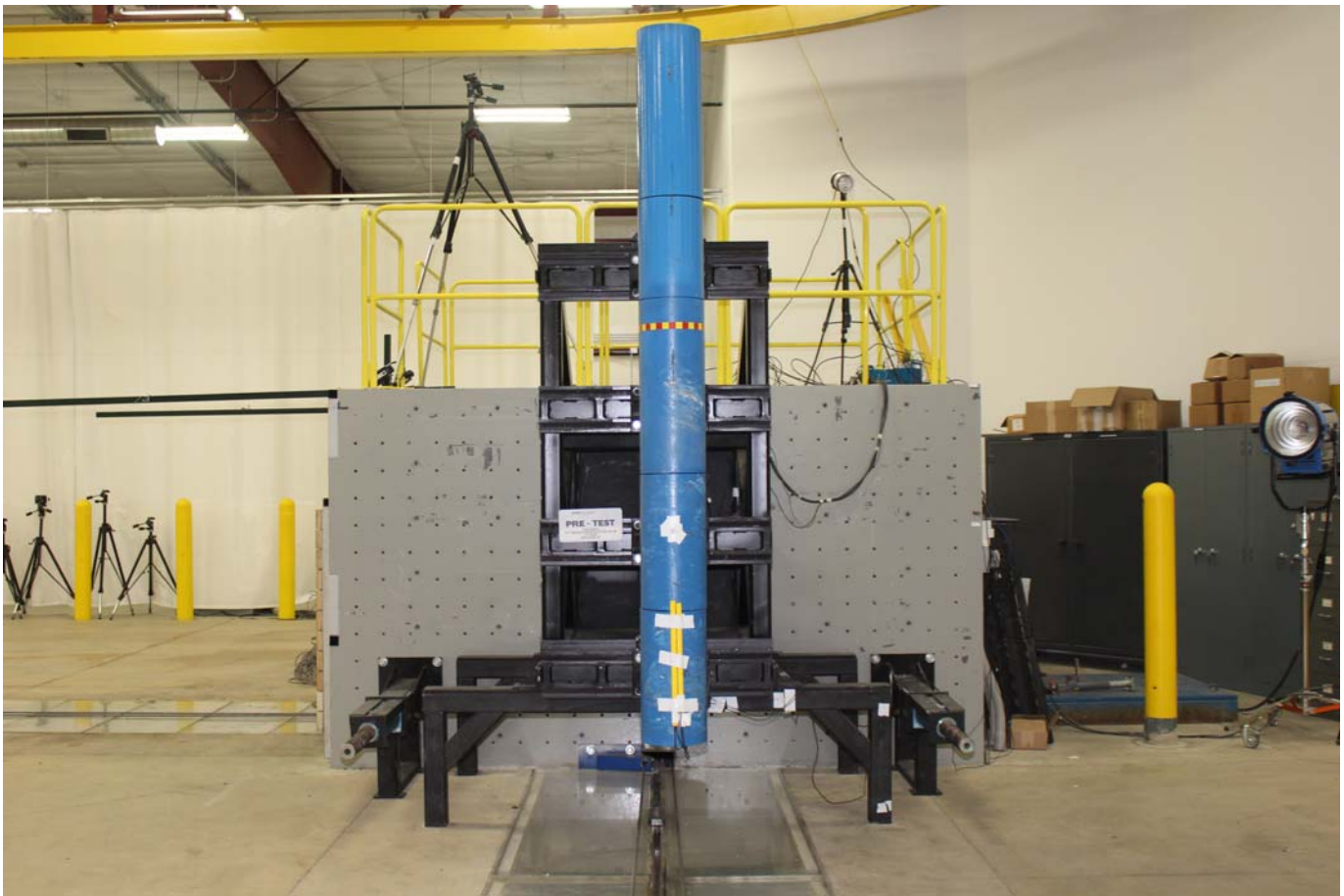
Photo No. 057 - Pre-Test Pole Barrier Front View
