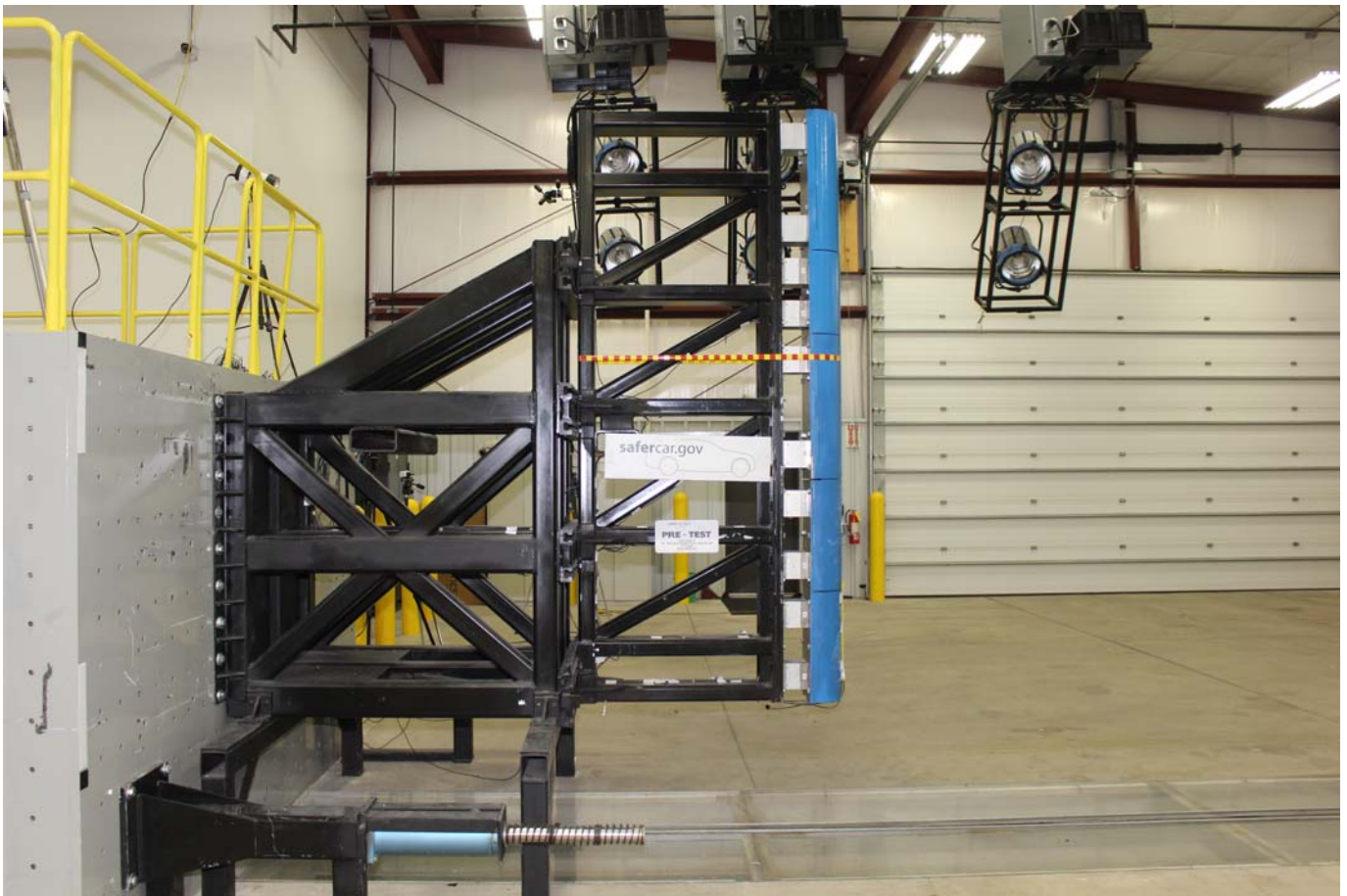
Photo No. 059 - Pre-Test Pole Barrier Side View
