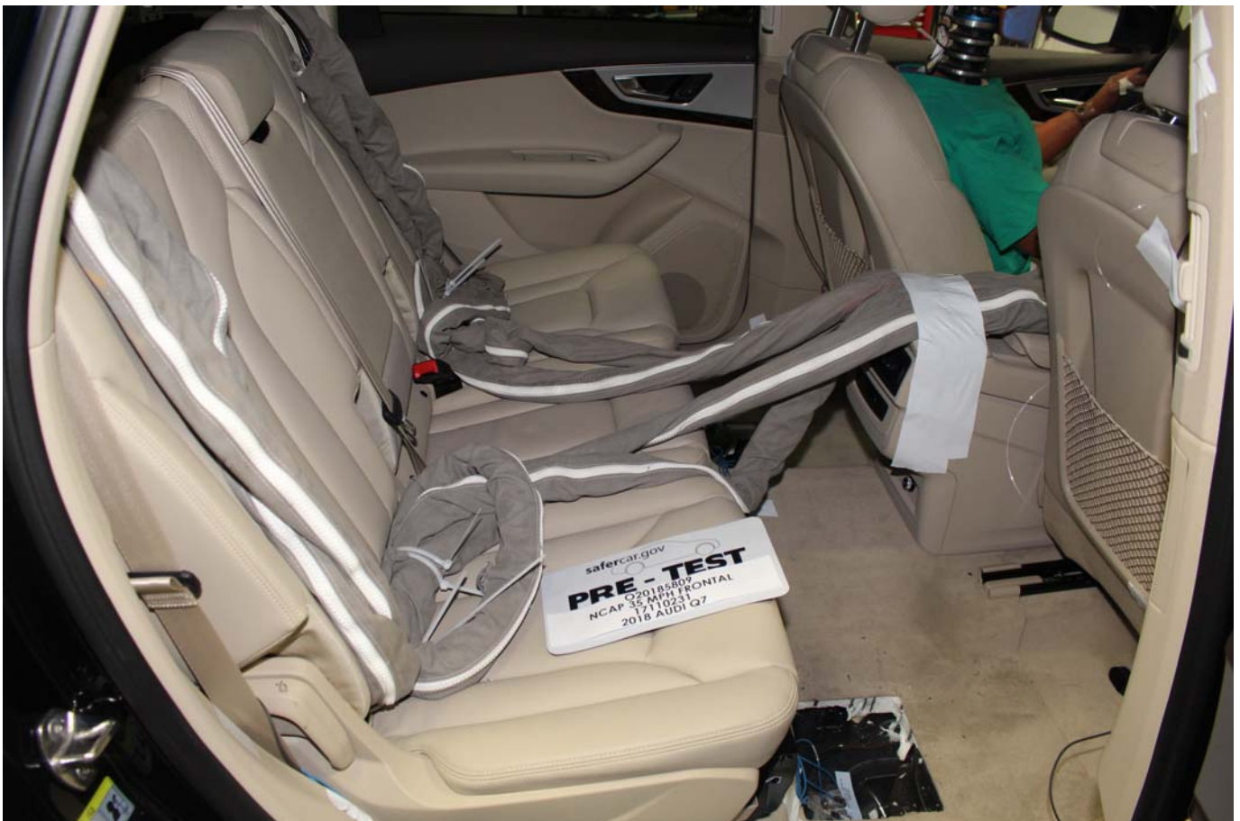
Photo No. 028 - Pre-Test Dummy Cable Routing
