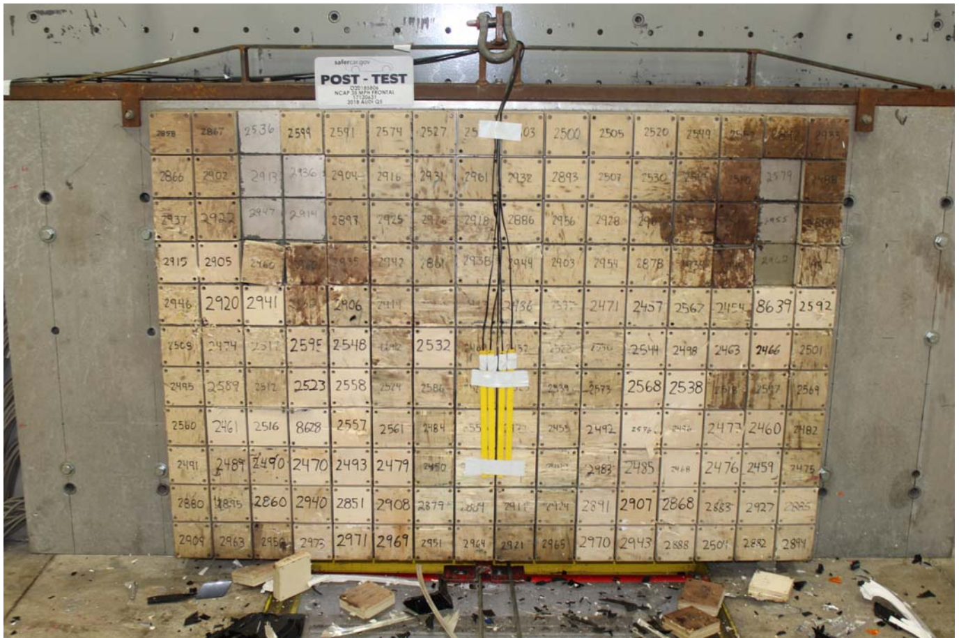
Photo No. 003 - Post-Test Load Cell Wall
