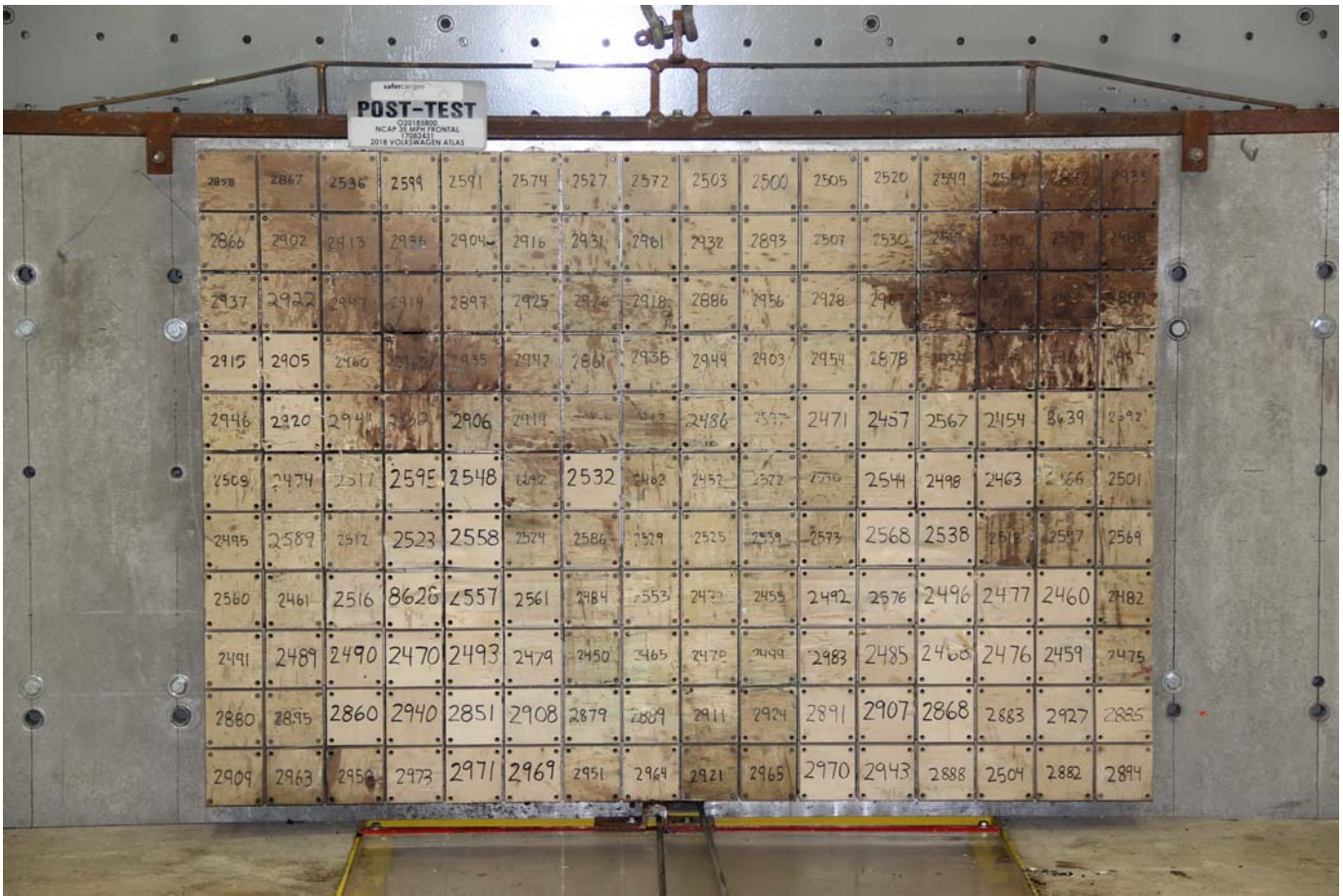
Photo No. 003 - Post-Test Load Cell Wall
